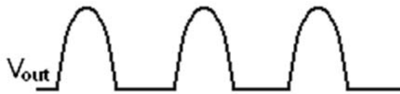
Figure 4.7: Half-wave output voltage for three input cycles.
