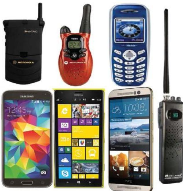
Examples of external and embedded/internal antennas in commercial cellular and CB radios.
