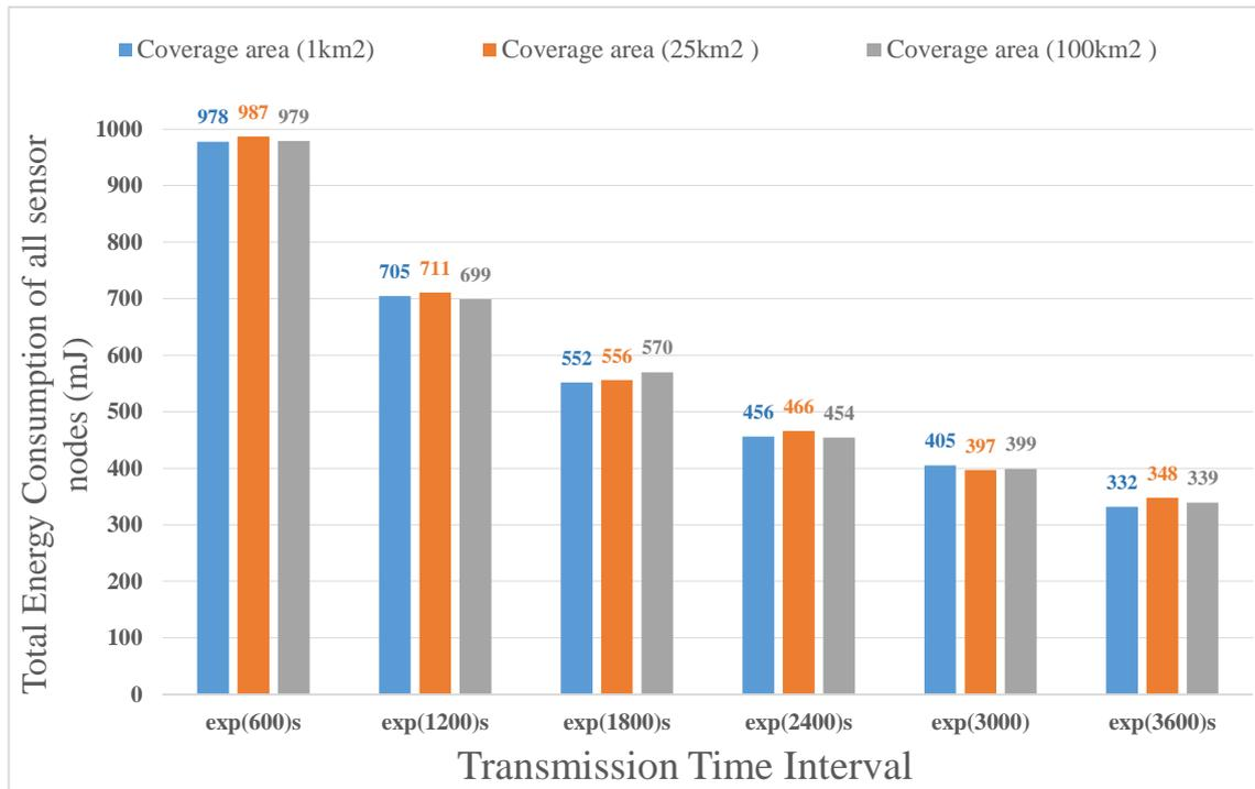
Figure 3.15 The total energy consumption of all sensor nodes vs. the transmission time interval in the coverage areas (1km<sup>2</sup>, 25km<sup>2</sup>, 100km<sup>2</sup>), using 4/5 code rate, 100 sensor nodes, one gateway placed at center of networks.
