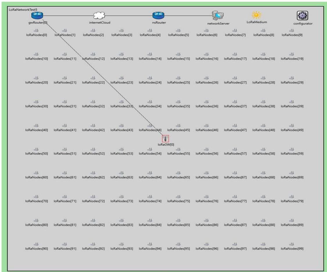
Figure 3.1 Network layout simulation of the Flora window with 100 sensor nodes and LoRa gateway communicated with the network server.
