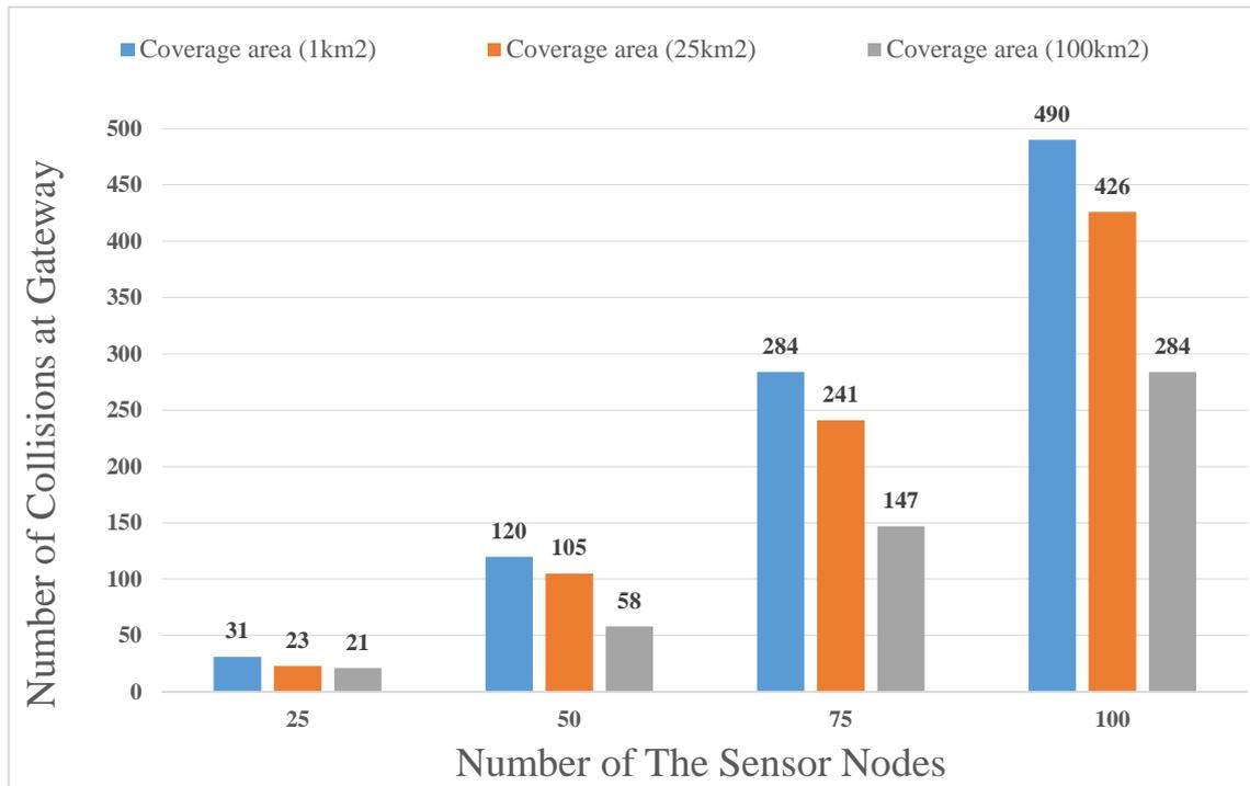
Figure 3.10 The number of collisions at the LoRa gateway vs. the number of the sensor nodes in the coverage areas (1km<sup>2</sup>, 25km<sup>2</sup>, 100km<sup>2</sup>), using 4/5 code rate, one gateway placed at the center of networks, and exp (600)s of the transmission time interval of packets.
