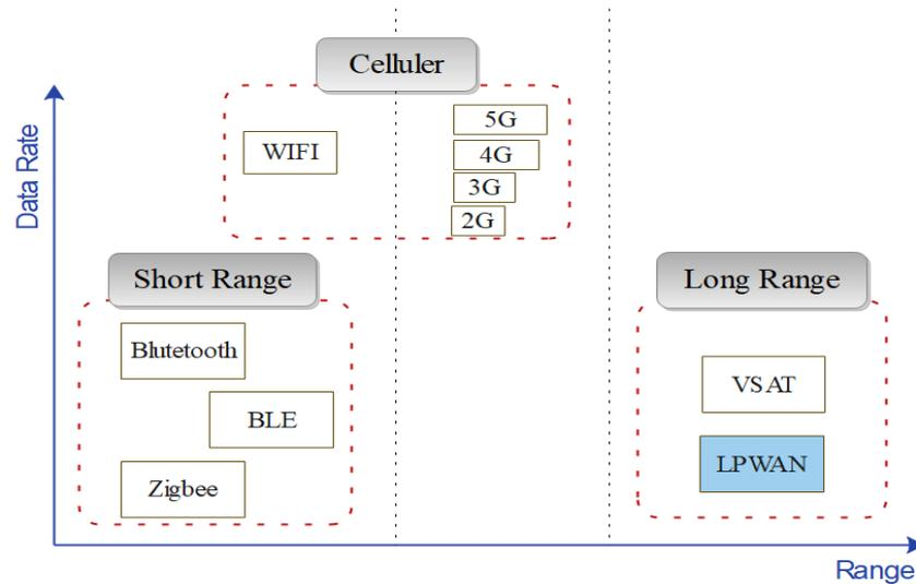
Figure 1.1 Desired data rate versus radio range capacity [1].
