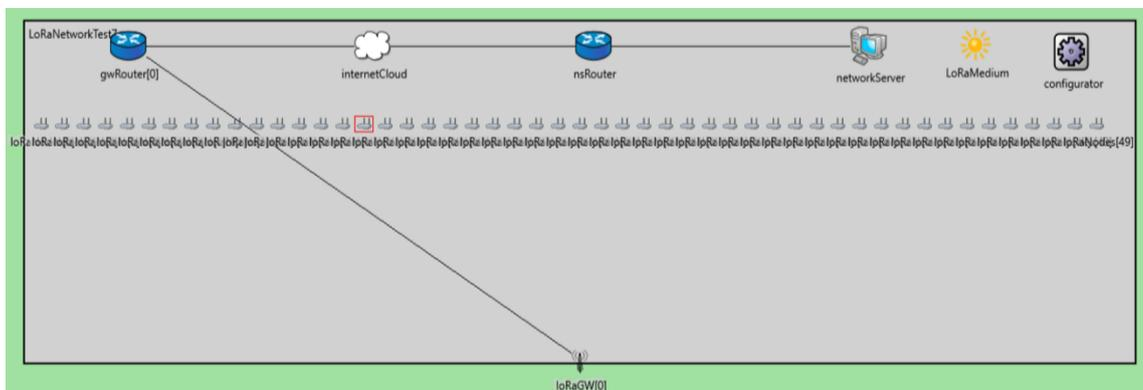
Figure 4.1 Screenshot of a Flora window simulation with 50 sensor nodes and one LoRa gateway communicated with a cloud of the things network (TTN).
