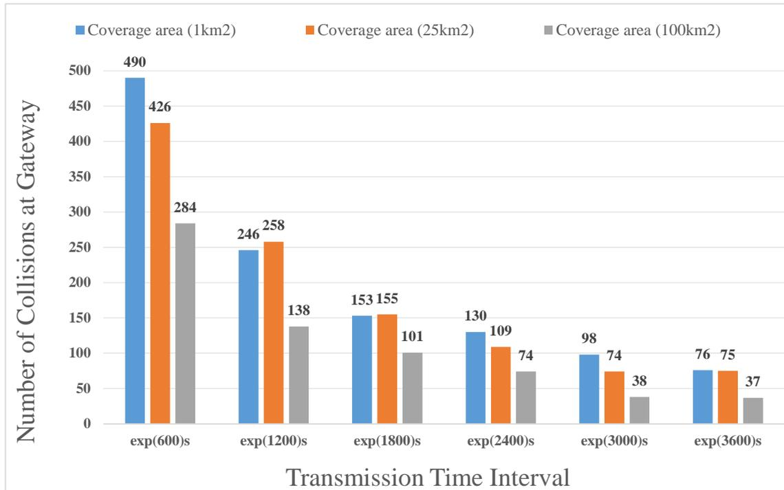
Figure 3.16 The number of collisions at the LoRa gateway vs. the transmission time interval in the coverage areas (1km<sup>2</sup>, 25km<sup>2</sup>, 100km<sup>2</sup>), using 4/5 code rate, 100 sensor nodes, one gateway placed at center of networks.
