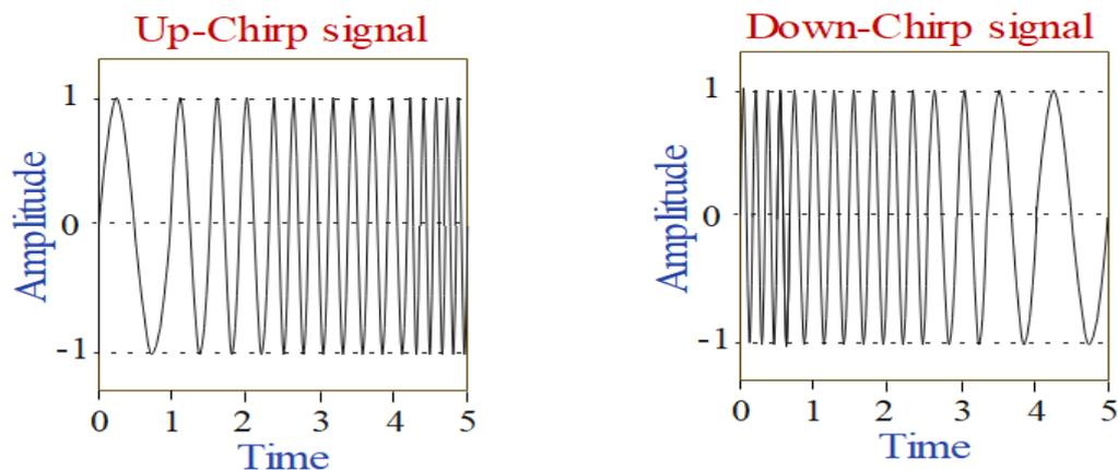
Figure 2.10 Up-chirp and down-chirp waveform [38].
