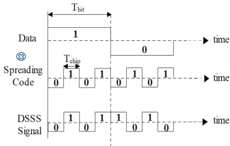
Figure 2.9 Signal of data, spreading code, and DSSS signal [52].
