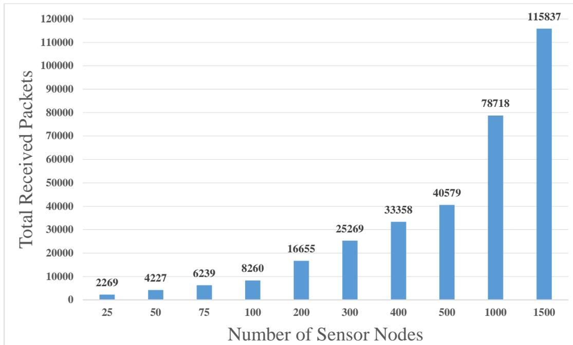
Figure 4.3 The total received packets at the network server vs. the number of sensor nodes, the time interval of transmitting packets exp (600s), one LoRa gateway is placed at (1750x 1000) m.
