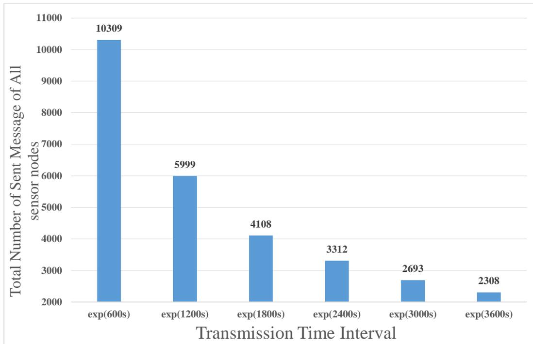
Figure 4.11 The total number of sent message of all sensor nodes vs. transmission time interval, the number of sensor nodes (100), and one LoRa gateway are placed at (1750x 1000) m.
