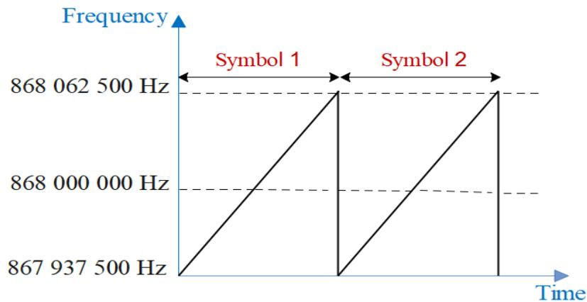
Figure 2.11 (a) LoRa up-chirp at BW= 125KHz [37].
