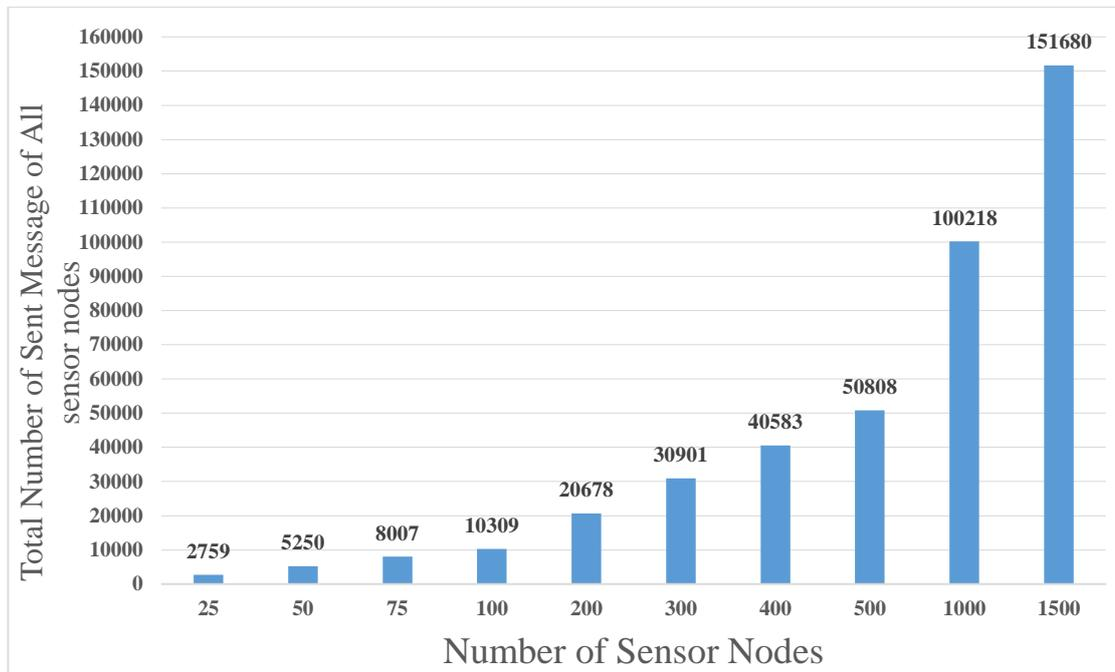
Figure 4.6 The total number of the sent message of all sensor nodes vs. the number of sensor nodes, the time interval of transmitting packets  $\exp(600s)$ , one LoRa gateway is placed at  $(1750 \times 1000)$  m.
