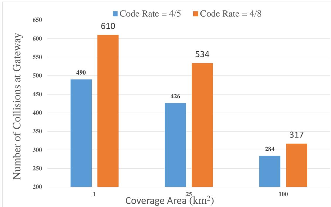
Figure 3.4 The number of collisions at the LoRa gateway vs. the coverage area at code rates 4/5 and 4/8, using 100 of the sensor nodes with one gateway placed at the center of networks, and exp (600)s of the transmission time interval of packets.
