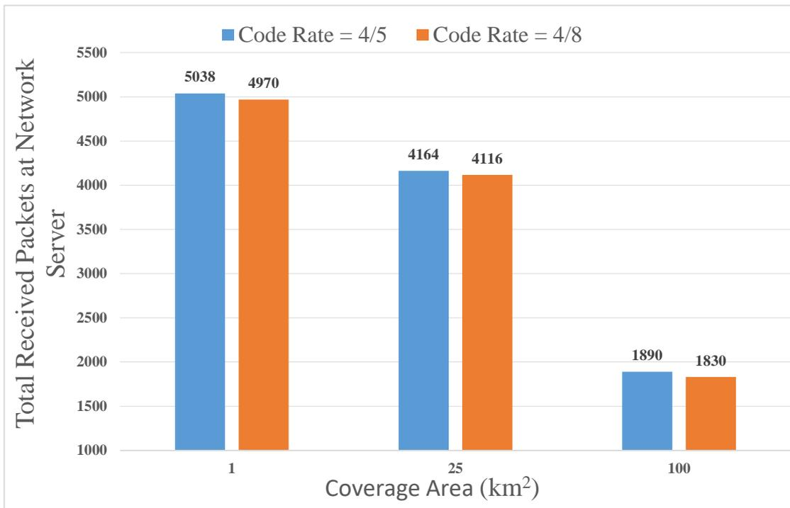
Figure 3.6 The total received packets at the network server vs. the coverage area at code rates 4/5 and 4/8, using 100 of the sensor nodes with
