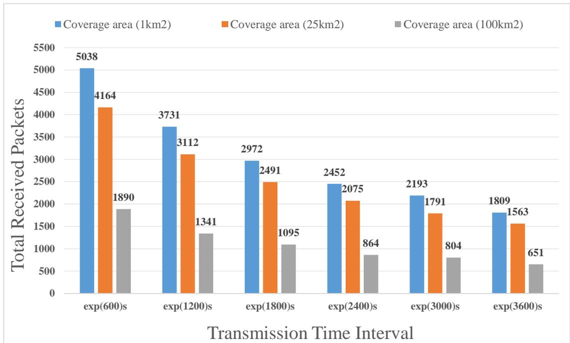
Figure 3.17 The total received packets at the server network vs. the transmission time interval in the coverage areas (1km<sup>2</sup>, 25km<sup>2</sup>, 100km<sup>2</sup>), using 4/5 code rate, 100 sensor nodes, one gateway placed at center of networks.
