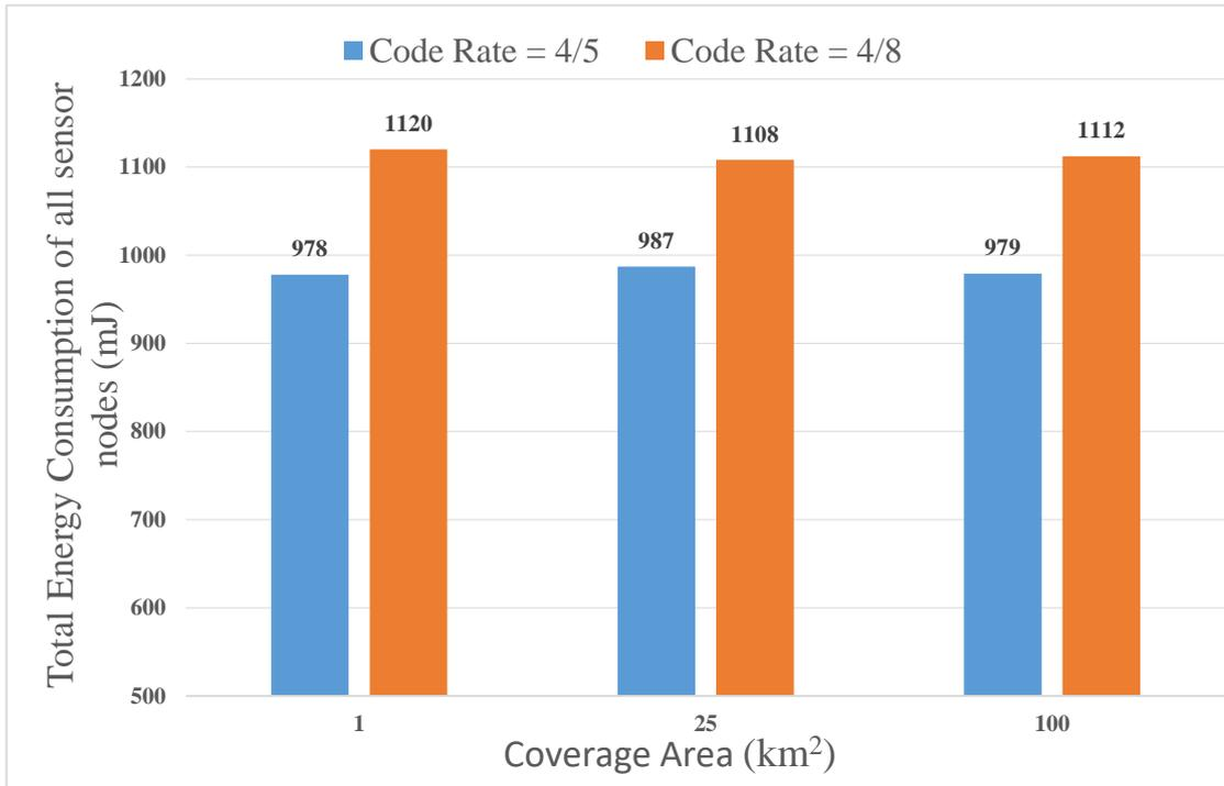
Figure 3.5 The total energy consumption of all sensor nodes vs. the coverage areas at code rates 4/5 and 4/8, using 100 of the sensor nodes with one gateway placed at the center of networks, and exp (600)s of the transmission time interval of packets.
