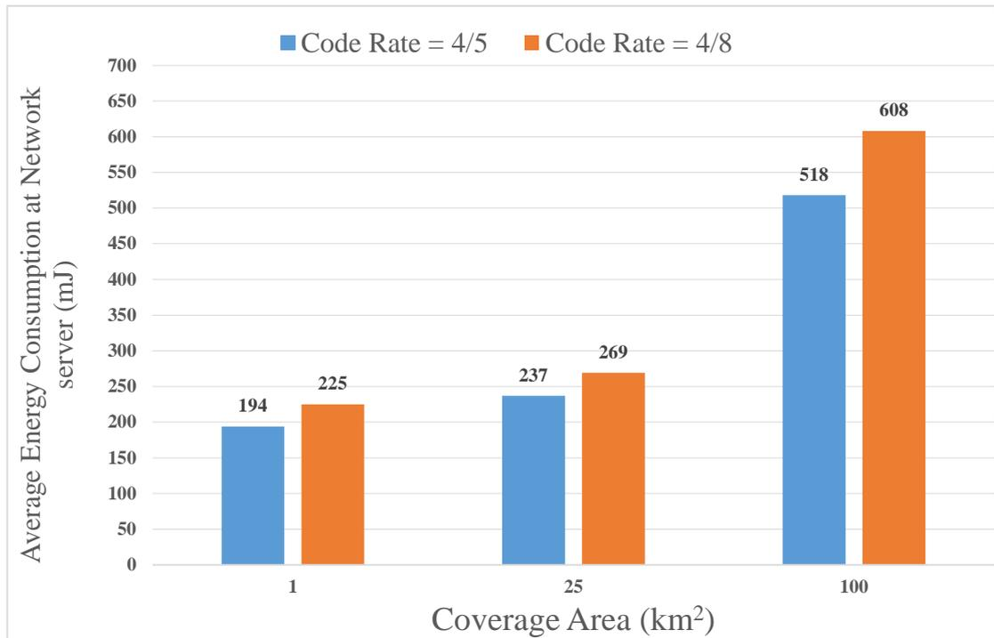
Figure 3.3 The average energy consumption at network server vs. the coverage area at code rates 4/5 and 4/8, using 100 of the sensor nodes with one gateway placed at the center of networks, and exp (600)s of the transmission time interval of packets.
