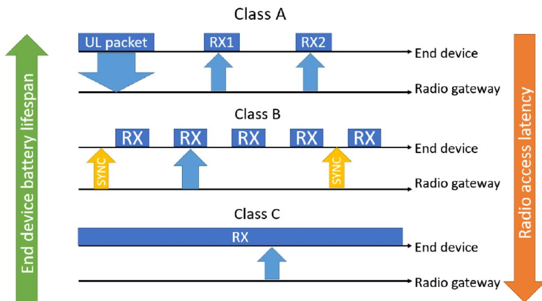
Figure 2.5 Graphical description of the three LoRaWAN classes [43].
