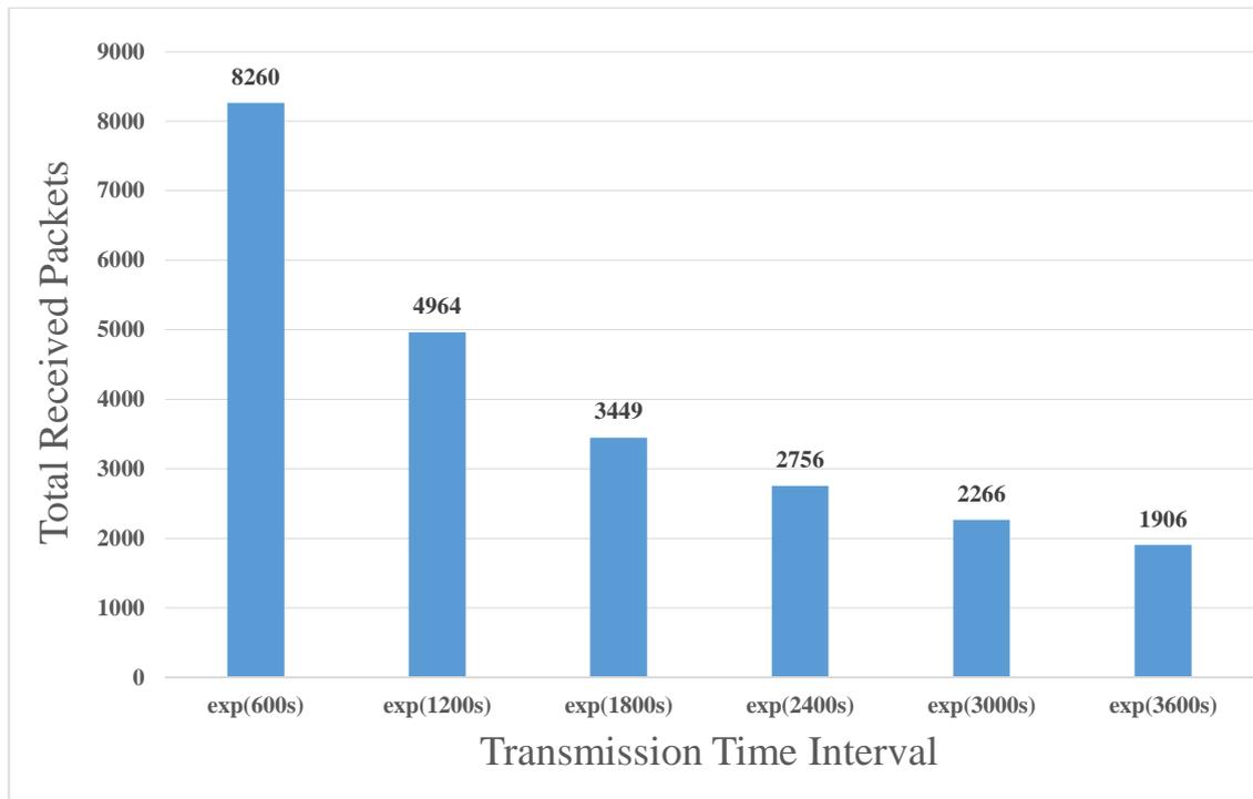
Figure 4.8 The total received packets at the server network vs. transmission time interval, the number of nodes (100), and one LoRa gateway placed at (1750x 1000) m.
