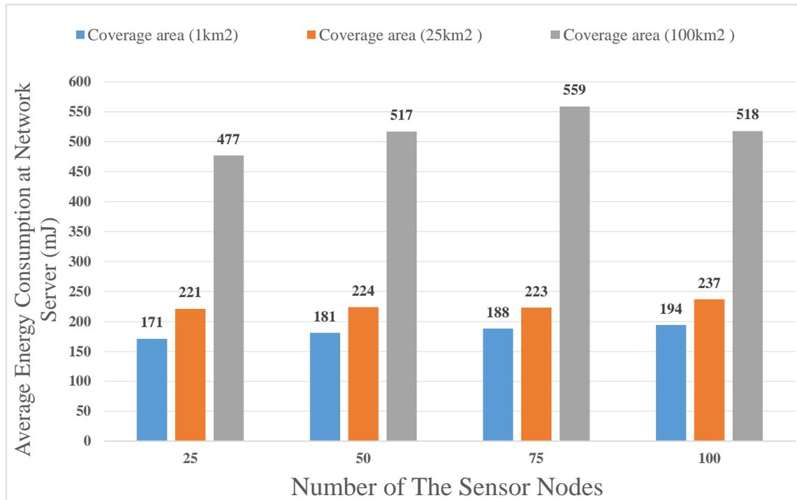
Figure 3.8 The Average energy consumption at the network server vs. the number of the sensor nodes in the coverage areas (1km<sup>2</sup>, 25km<sup>2</sup>, 100km<sup>2</sup>), using a 4/5 code rate, one gateway placed at the center of networks, and exp (600)s of the transmission time interval of packets.
