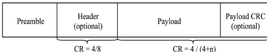
Figure 2.8 LoRa packet structure [48].
