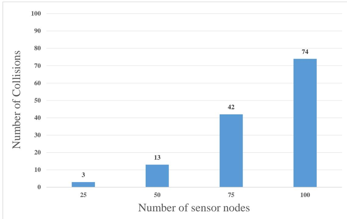
Figure 4.4 The number of collisions at the LoRa gateway vs. the number of sensor nodes, the time interval of transmitting packets  $\exp(600s)$ , one LoRa gateway is placed at  $(1750 \times 1000)$  m.
