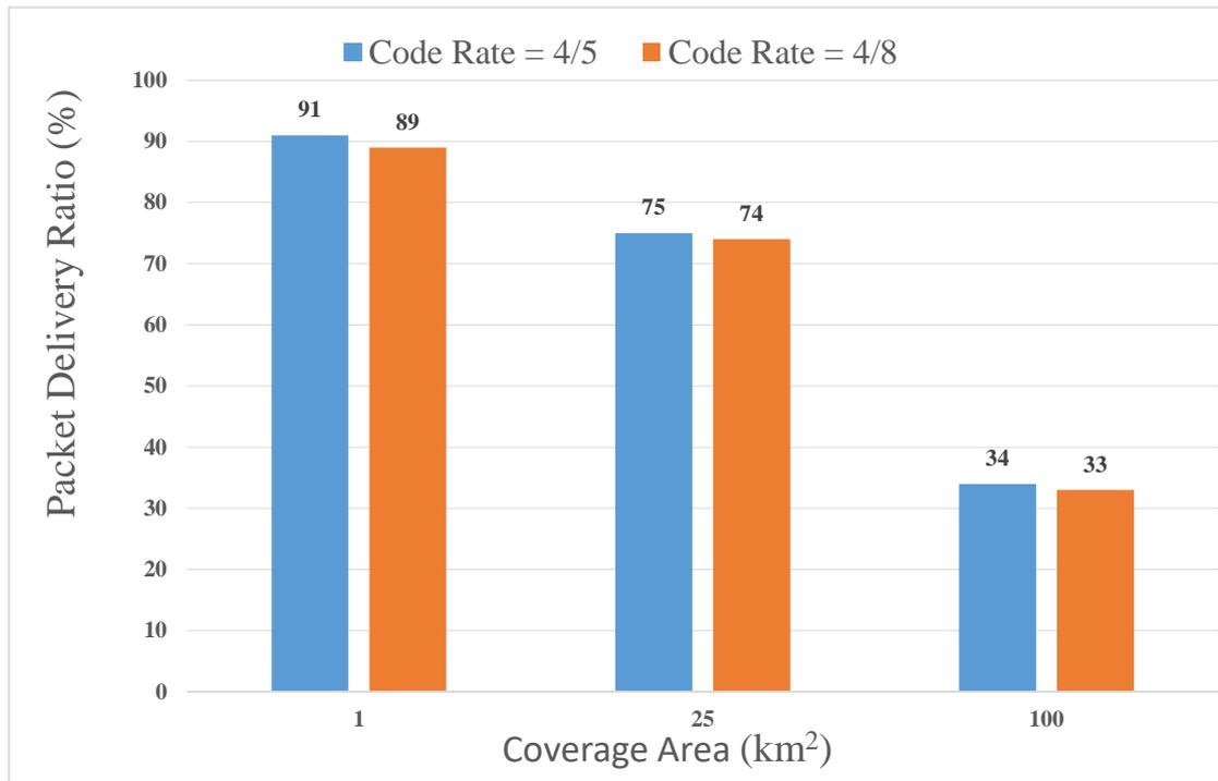
Figure 3.2 The Packet Delivery Ratio vs. the coverage areas at code
