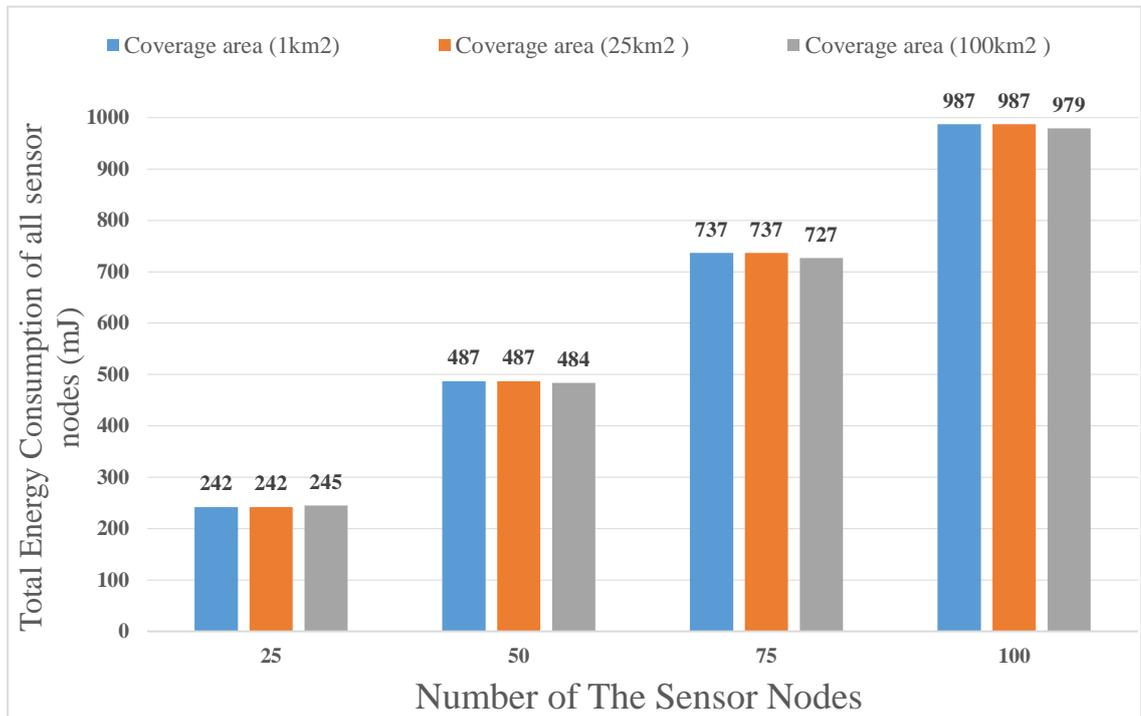
Figure 3.9 The total energy consumption of all sensor nodes vs. the number of the sensor nodes in the coverage areas (1km<sup>2</sup>, 25km<sup>2</sup>, 100km<sup>2</sup>), using 4/5 code rate, one gateway placed at the center of networks, and exp (600)s of the transmission time interval of packets.
