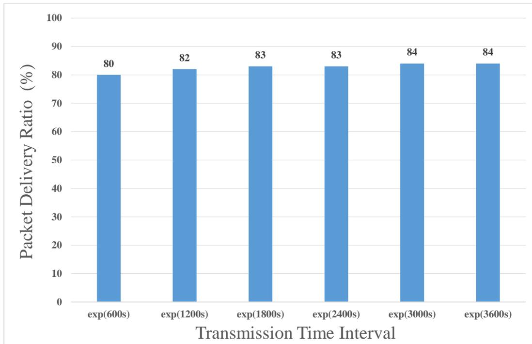
Figure 4.7 The packet delivery ratio vs. transmission time interval, the number of sensor nodes (100), and one LoRa gateway are placed at (1750x 1000) m.
