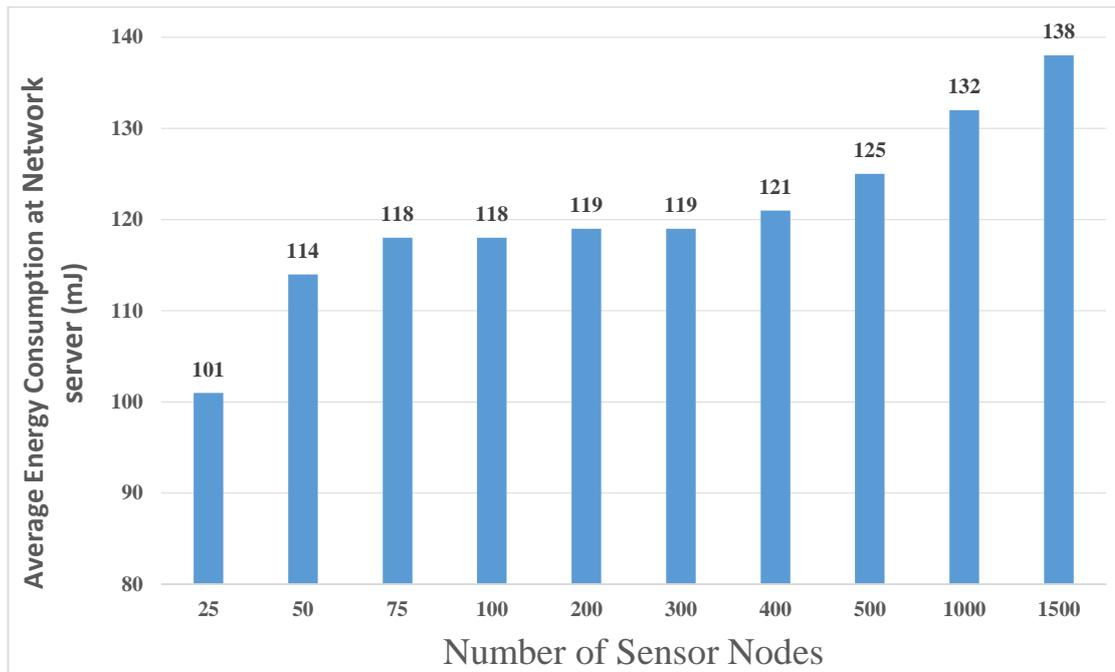
Figure 4.5 The average energy consumption at the network server vs. the number of sensor nodes, the time interval of transmitting packets exp (600s), one LoRa gateway is placed at (1750x 1000) m.
