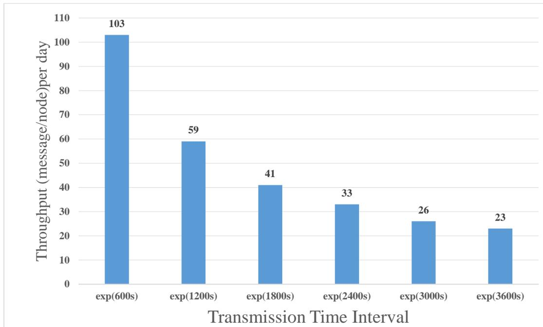
Figure 4.12 The throughput is the total number of sent messages divided by the total of sensor nodes during the day vs. the transmission time interval. The time interval of transmitting packets exp (600s), one LoRa gateway is placed at (1750x 1000) m.
