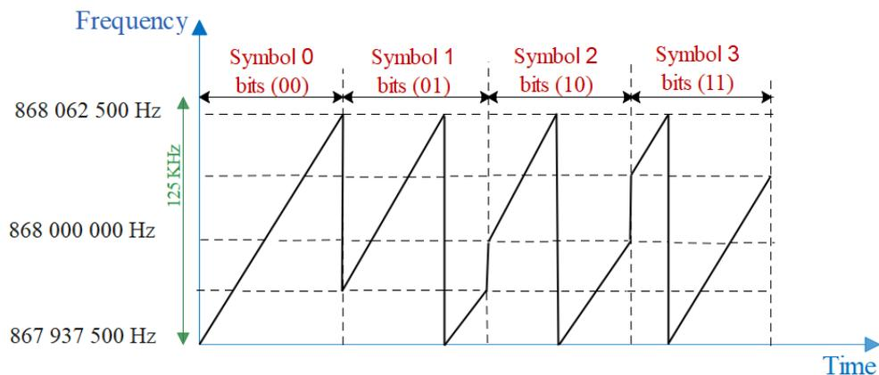
Figure 2.11 (b) Each chirp is split into  $2^2$  chips [37].
