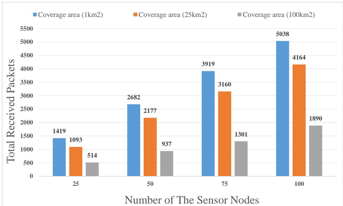
Figure 3.11 The total received packets at the network server vs. the number of the sensor nodes in the coverage areas (1km<sup>2</sup>, 25km<sup>2</sup>, 100km<sup>2</sup>), using 4/5 code rate, one gateway placed at the center of networks, and exp (600)s of the transmission time interval of packets.
