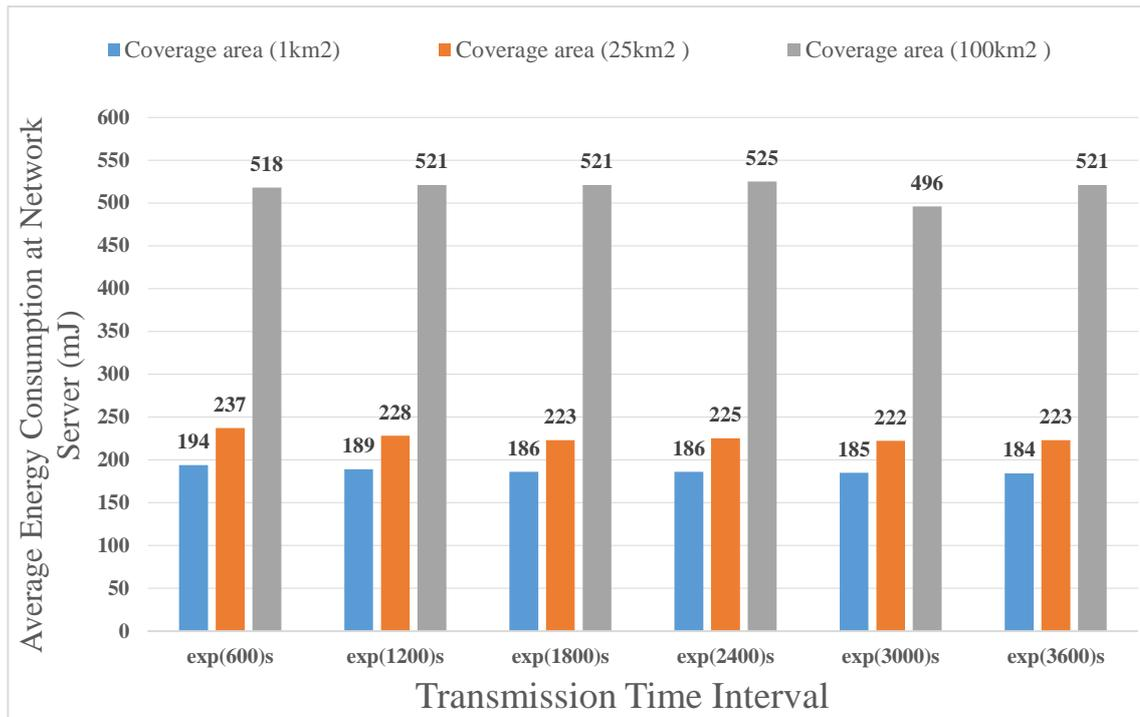
Figure 3.14 The Average energy consumption at the network server vs. the transmission time interval in the coverage areas (1km<sup>2</sup>, 25km<sup>2</sup>, 100km<sup>2</sup>), using a 4/5 code rate, 100 sensor nodes, and one gateway placed at the center of networks.
