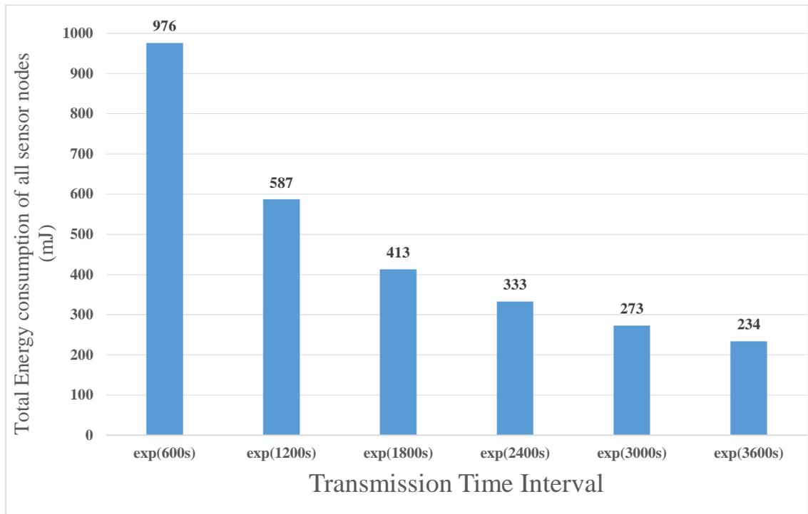
Figure 4.10 The total energy consumption of all sensor nodes vs. transmission time interval. The number of nodes (100), and one LoRa gateway is placed at (1750x 1000) m.
