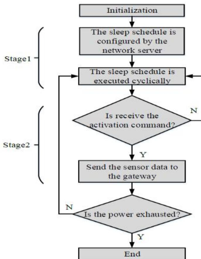
Figure 2.4 Flowchart of each LoRa sensor node [41].
