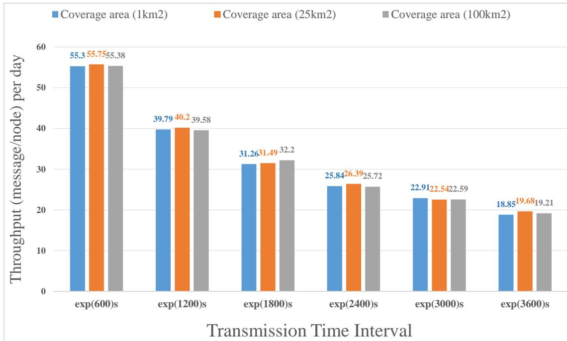
Figure 3.19 The throughput is the total number of sent messages divided by the total sensor nodes during the day vs. the transmission time interval in the coverage areas (1km<sup>2</sup>, 25km<sup>2</sup>, 100km<sup>2</sup>), using 4/5 code rate, 100 sensor nodes, one gateway placed at center of networks.
