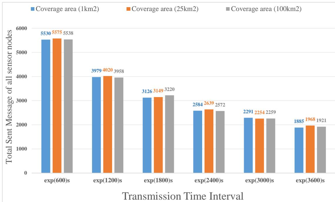
Figure 3.18 The total sent message of all sensor nodes vs. the transmission time interval in the coverage areas (1km<sup>2</sup>, 25km<sup>2</sup>, 100km<sup>2</sup>), using 4/5 code rate, 100 sensor nodes, one gateway placed at center of networks.
