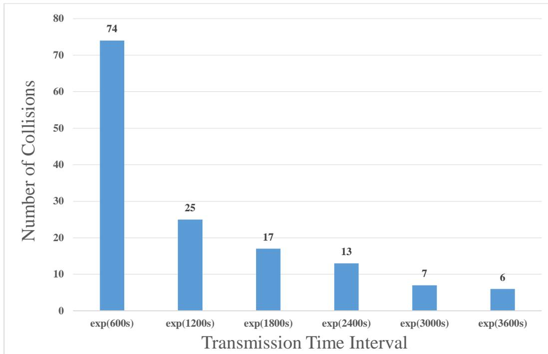
Figure 4.9 The number of collisions at the LoRa gateway vs. transmission time interval, the number of sensor nodes (100), and one LoRa gateway are placed at (1750x 1000) m.
