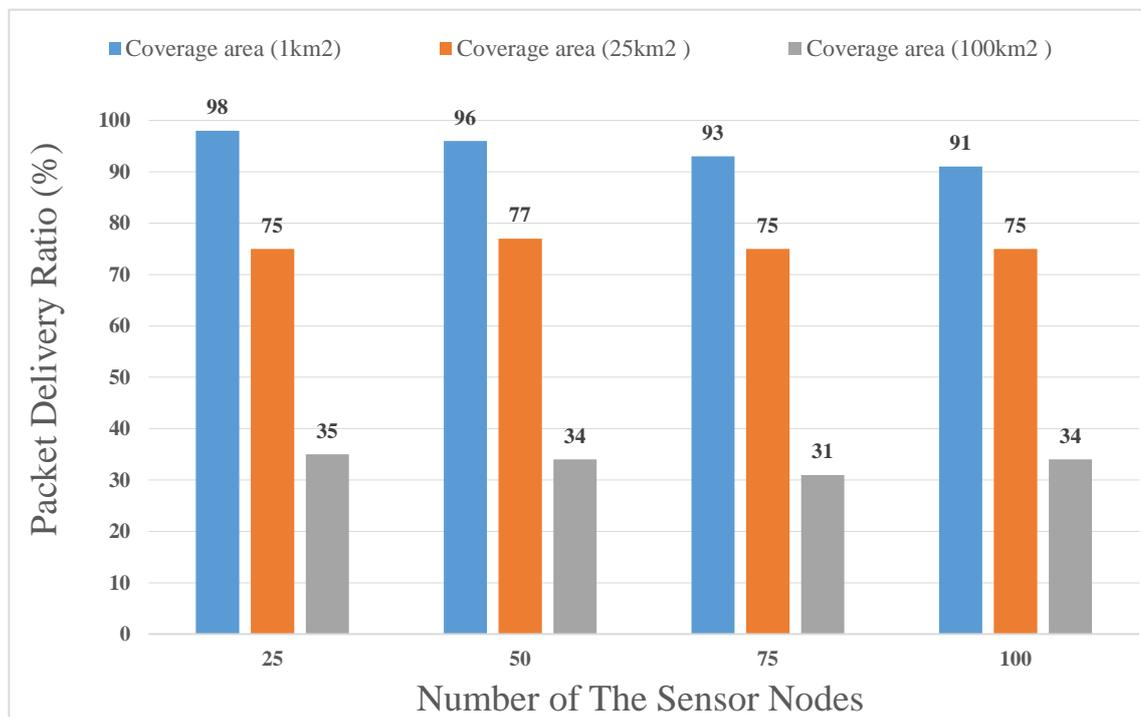
Figure 3.7 The packet delivery ratio vs. the number of the sensor nodes in the coverage areas (1km<sup>2</sup>, 25km<sup>2</sup>, 100km<sup>2</sup>), using 4/5 code rate, one gateway placed at center of networks, and exp (600)s of the transmission time interval of packets.
