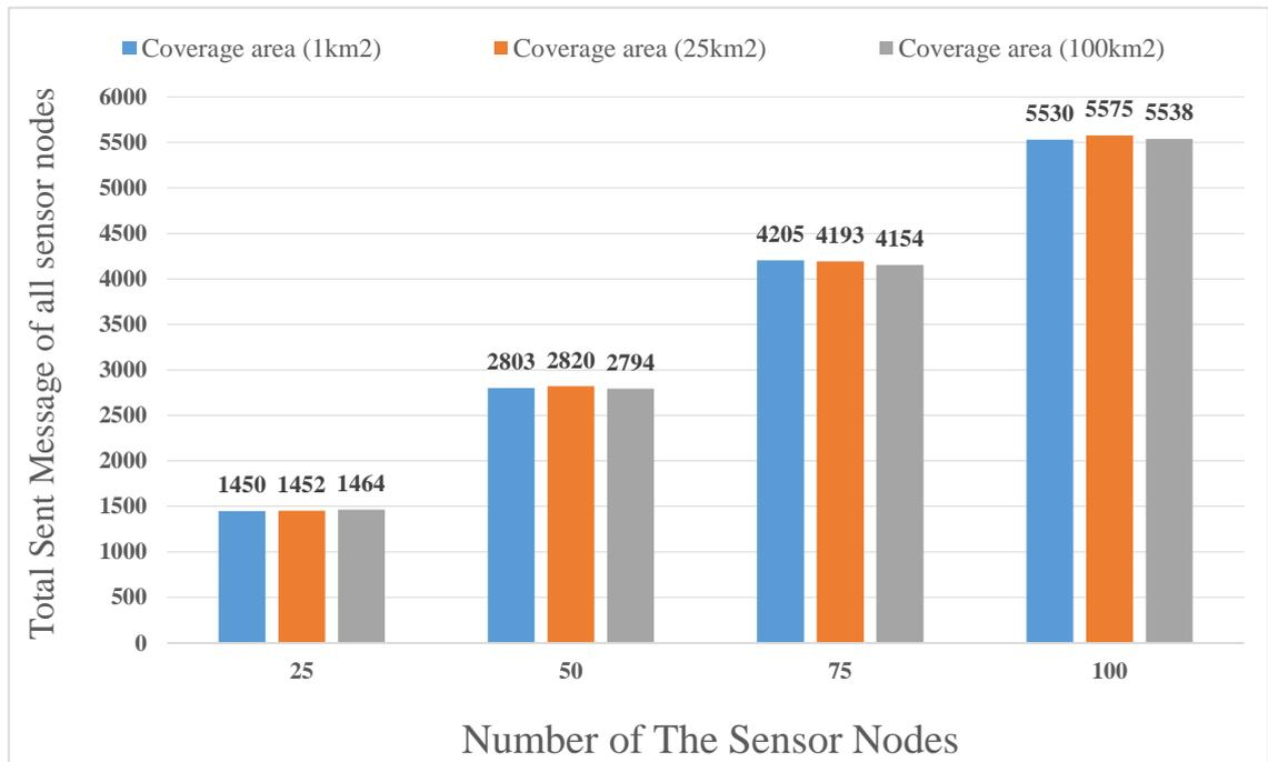
Figure 3.12 The total sent message of all sensor nodes vs. the number of the sensor nodes in the coverage areas (1km<sup>2</sup>, 25km<sup>2</sup>, 100km<sup>2</sup>), using 4/5 code rate, one gateway placed at the center of networks, and exp (600)s of the transmission time interval of packets.
