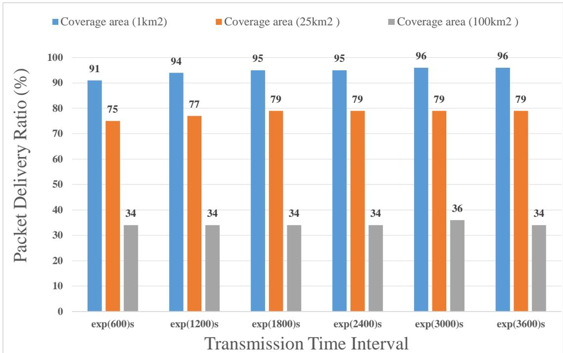
Figure 3.13 The packet delivery ratio vs. the transmission time interval in the coverage areas (1km<sup>2</sup>, 25km<sup>2</sup>, 100km<sup>2</sup>), using a 4/5 code rate, 100 sensor nodes, and one gateway placed at the center of networks.
