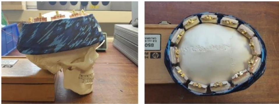
Figure 1. 11: The microwave imaging device, designed to be worn as a head strap, incorporates antennas fabricated from textile materials [35].
