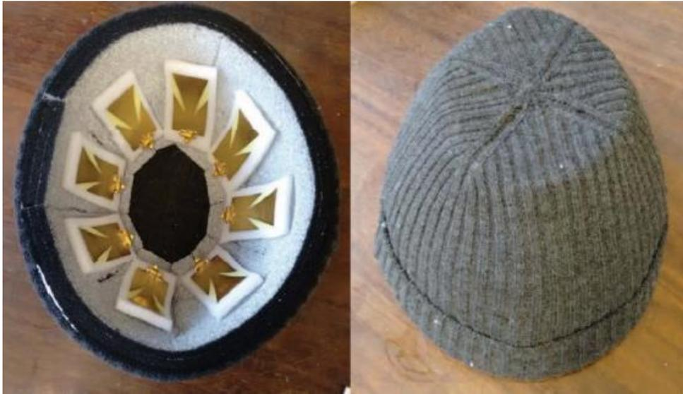
Figure 1. 10: First prototype of a head-mounted microwave imaging device utilizes thin, flexible antennas placed on a PET-film substrate [35].
