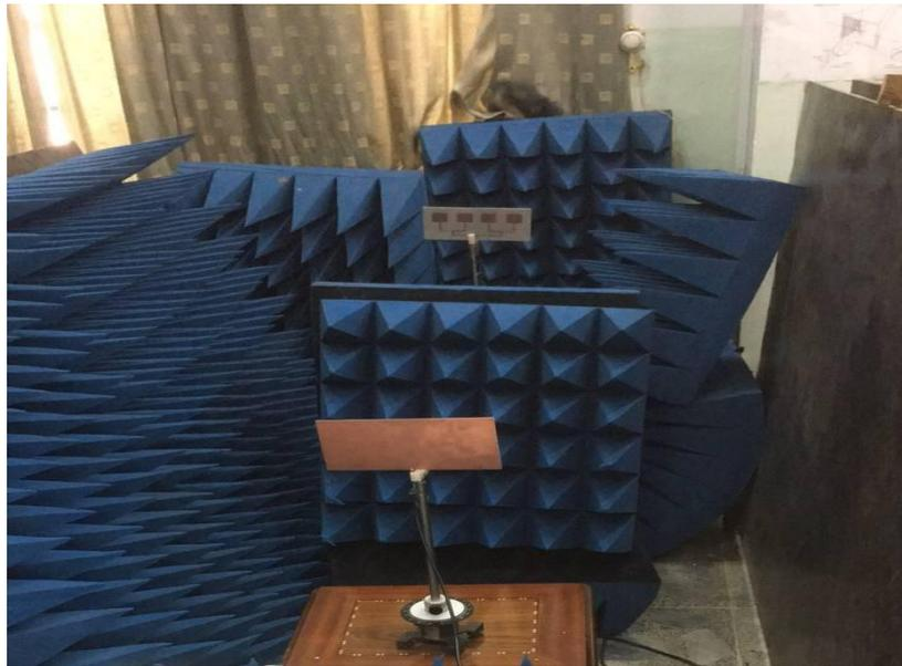
**Figure 4.8.** Measurement of the radiation pattern in the lab.
