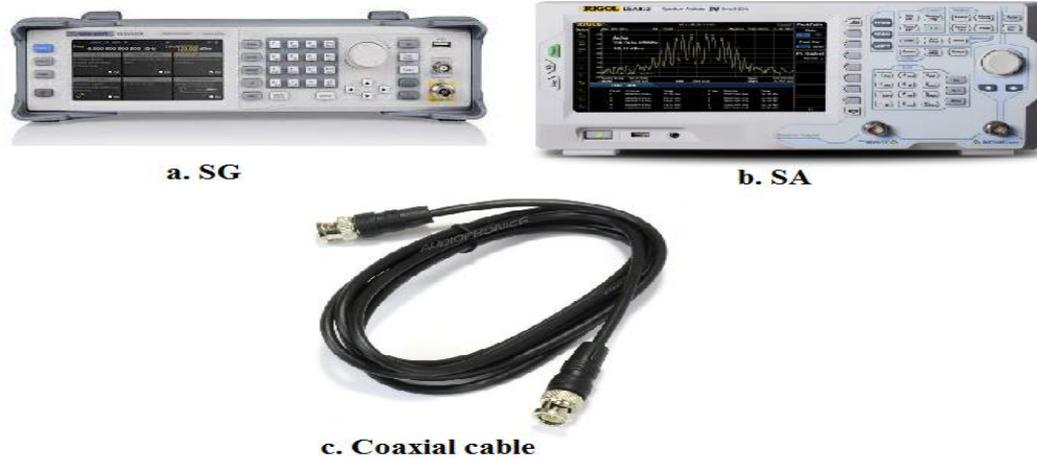
**Figure 4.5.** Laboratory devices.
