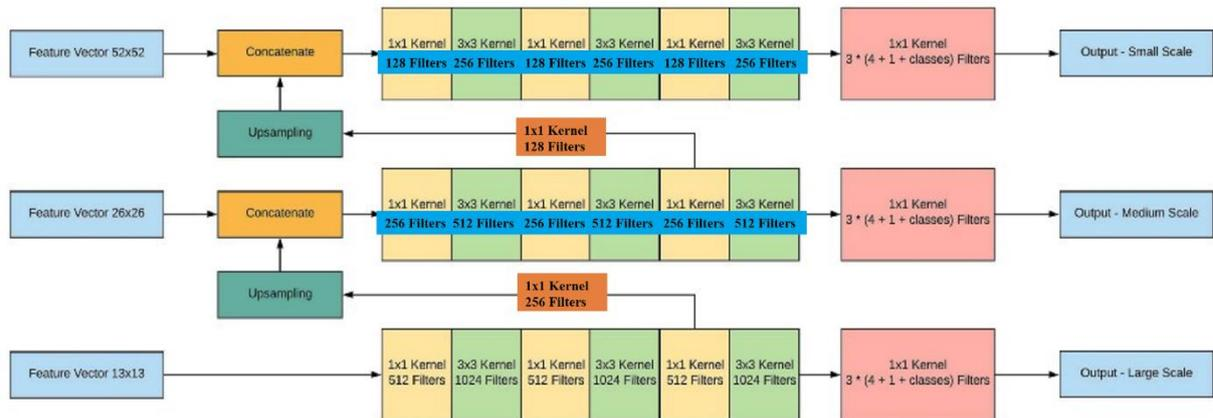
Figure 3.10 Up-Sampling layers and YOLO layers
