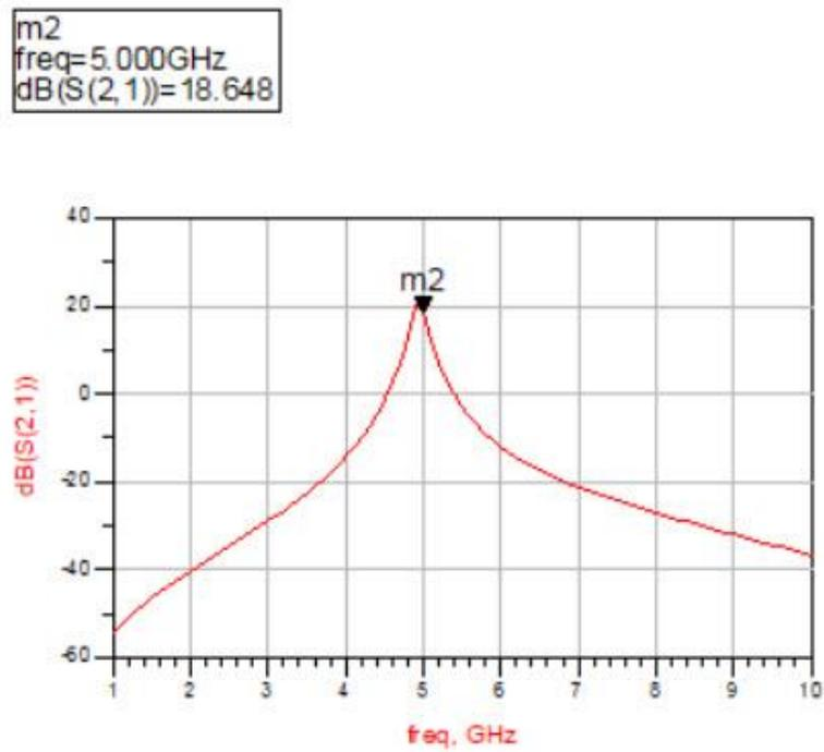
Figure (4-17): Optimized Power Gain Result for 5 GHz DLNA
