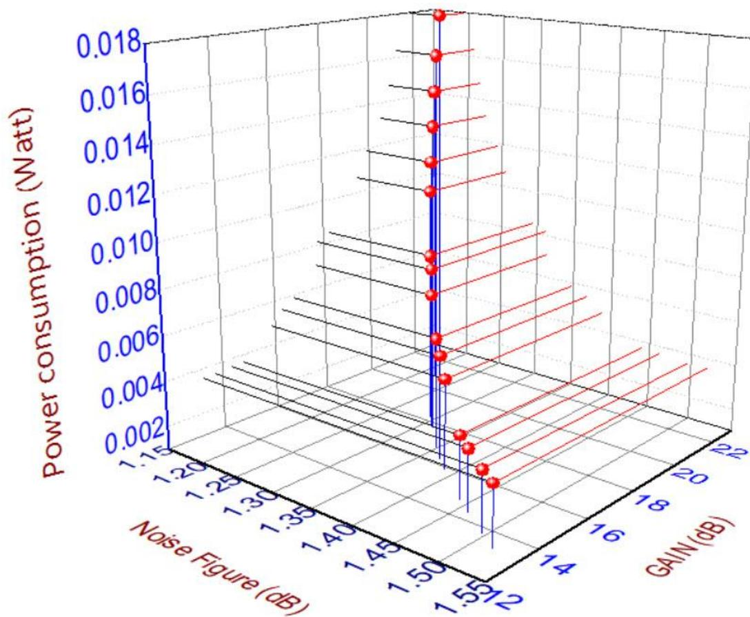
Figure (4-15): Three Dimensional Relationship Between NF, Gain and Power Consumption for 5 GHz DLNA
