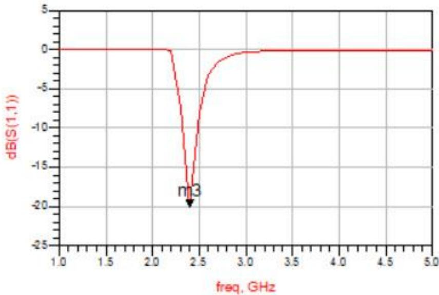
Figure (4-11):  $S_{11}$  Based on Optimized ( $L_s$  and  $L_g$ ) at 2.4 GHz DLNA
