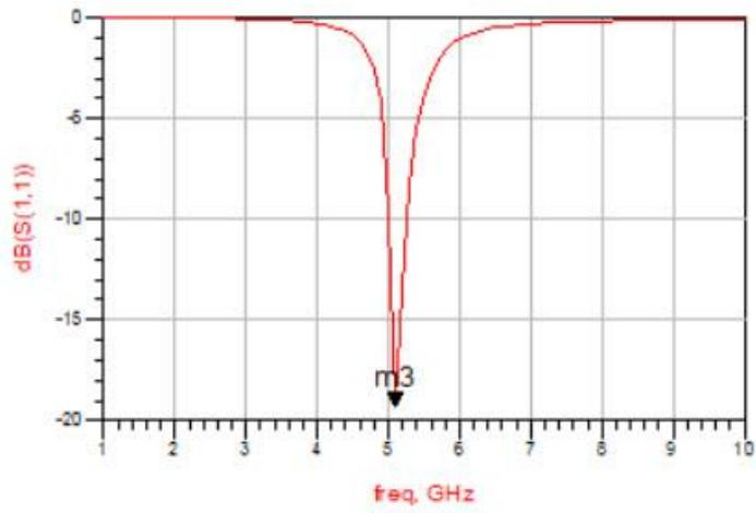
Figure (4-21):  $S_{11}$  Based on Optimized ( $L_S$  and  $L_g$ ) at 5 GHz DLNA
