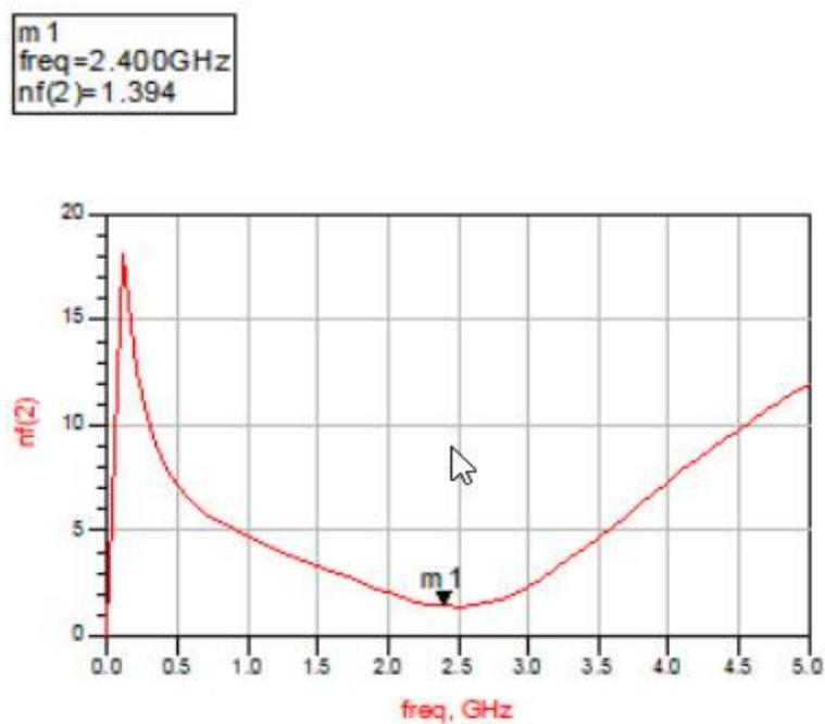
Figure (3-3): Mathematical NF for 2.4 GHz Single Ended LNA
