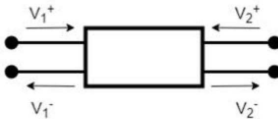
Figure (2-2): Incident and Reflected Waves in a Two-Port Network [42]
