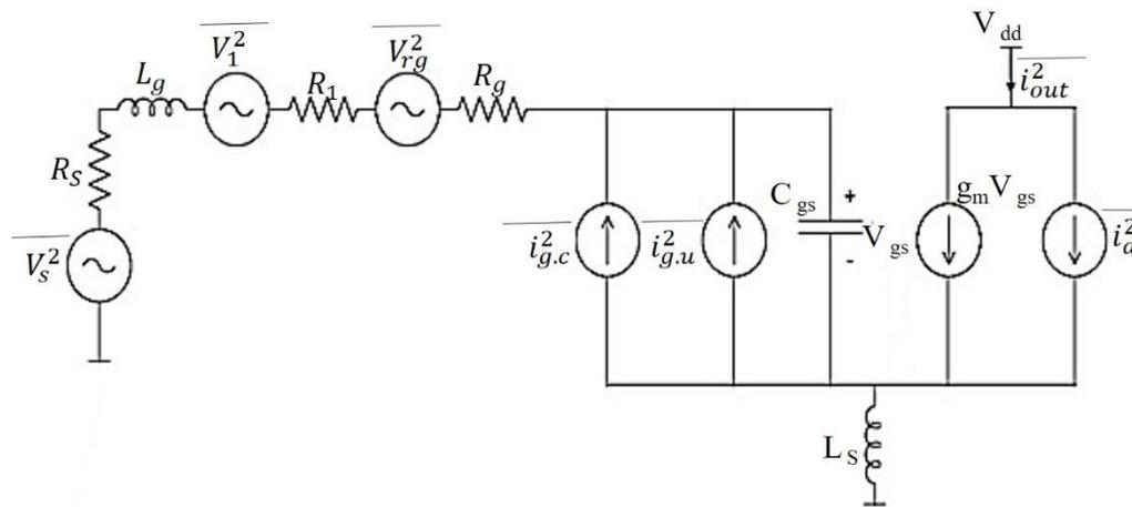
Figure (2-3): Equivalent Circuit for Input Stage for Noise Calculation [44].
