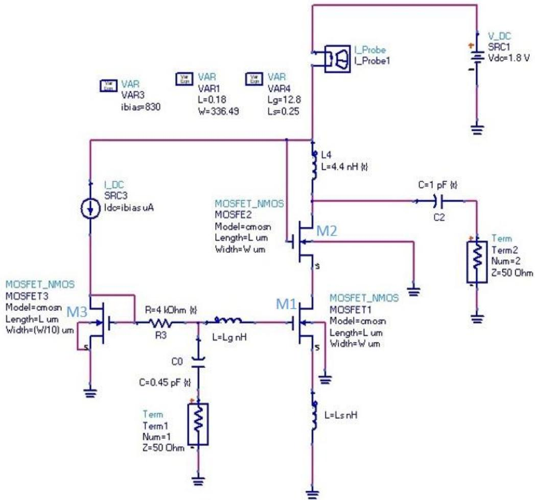
Figure (3-1): Single Ended LNA Topology Simulation Using ADS
