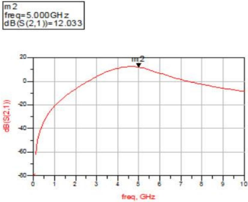
Figure (3-18): Mathematical Power Gain Result for 5 GHz Single Ended LNA
