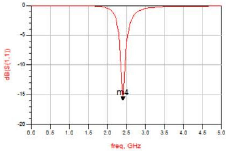
Figure (3-11): The Input Return Loss  $S_{11}$  Optimized Result for 2.4 GHz
