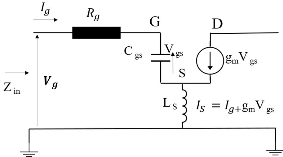
Figure (3-2): New Equivalent Model of MOSFET with Source Degeneration Added .
