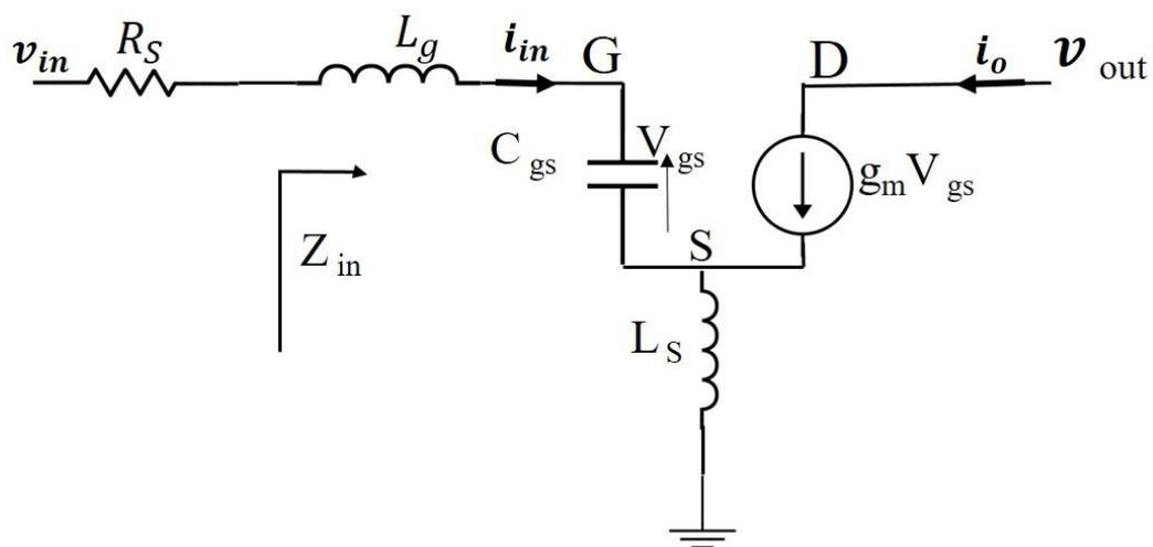
Figure (2-6): Small Signal Model of LNA
