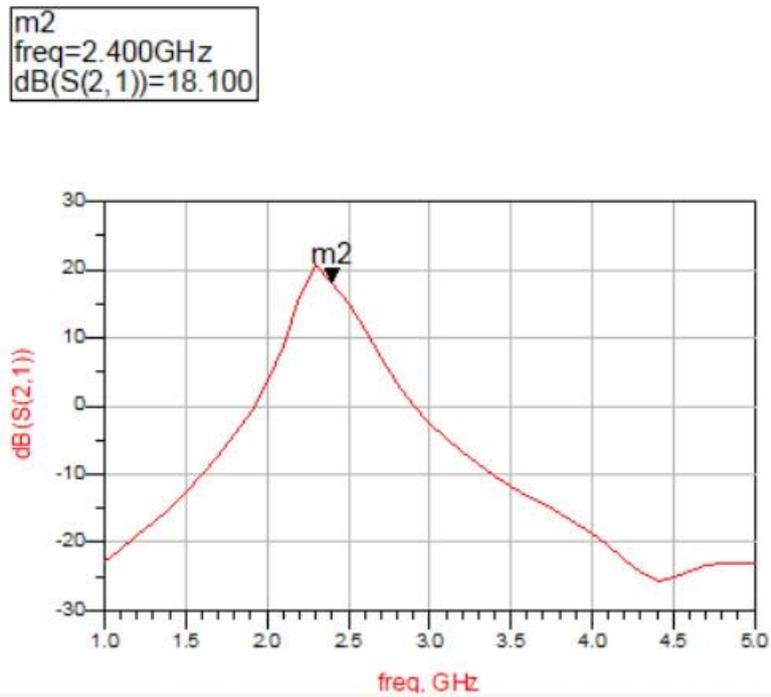
Figure (4-10):  $S_{21}$  Based on Optimized ( $L_S$  and  $L_g$ ) at 2.4 GHz DLNA
