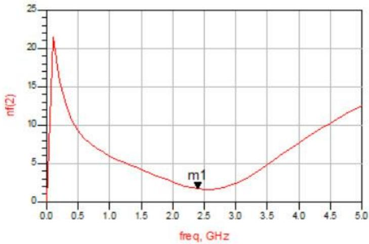
Figure (3-14): NF Based on Optimized ( $L_s$  and  $L_g$ ) at 2.4 GHz Single Ended LNA
