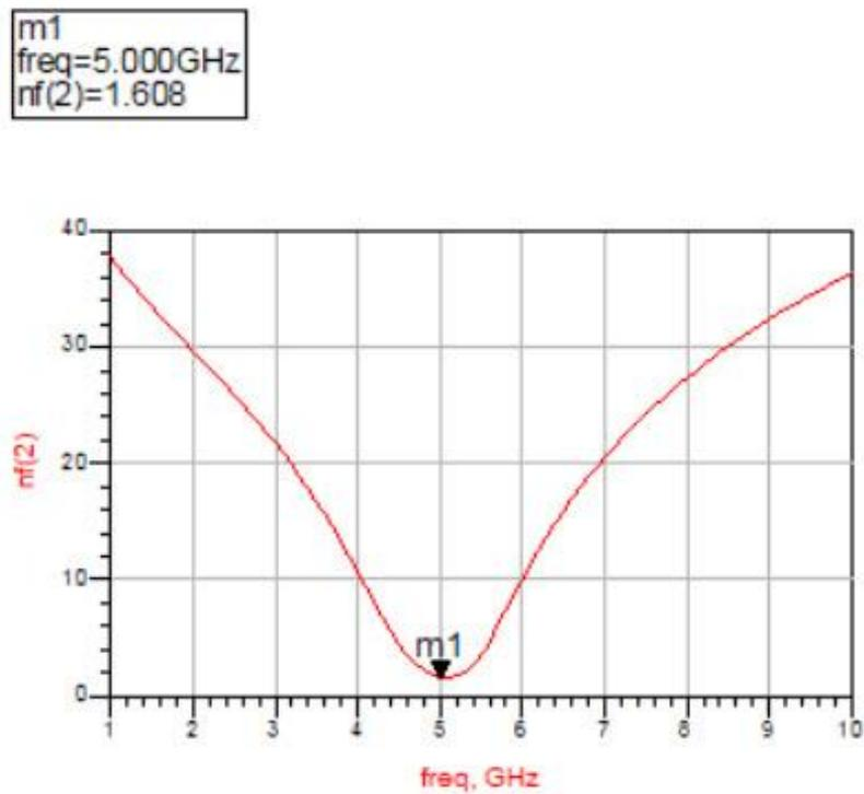
Figure (4-16): Optimized NF Result for 5 GHz DLNA
