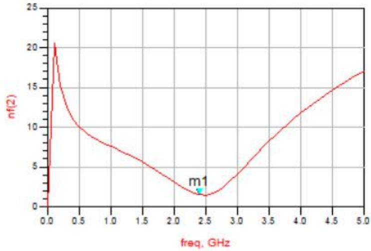
Figure (3-9): NF Optimized Result for 2.4 GHz Single Ended LNA
