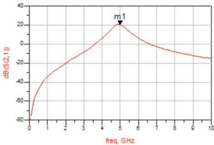
Figure (3-25): Optimized Power Gain Result for 5 GHz Single Ended LNA
