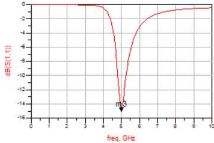
Figure (3-31):  $S_{11}$  Based on Optimized ( $L_s$  and  $L_g$ ) at 5 GHz Single Ended LNA
