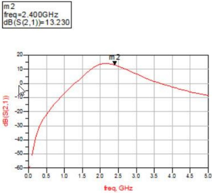
Figure (3-4): Mathematical Power Gain for 2.4 GHz Single Ended LNA
