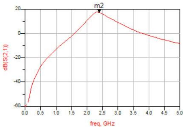
Figure (3-15):  $S_{21}$  Based on Optimized ( $L_s$  and  $L_g$ ) at 2.4 GHz Single Ended LNA
