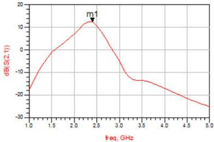
Figure (4-3): Mathematical Power Gain Result for 2.4 GHz DLNA
