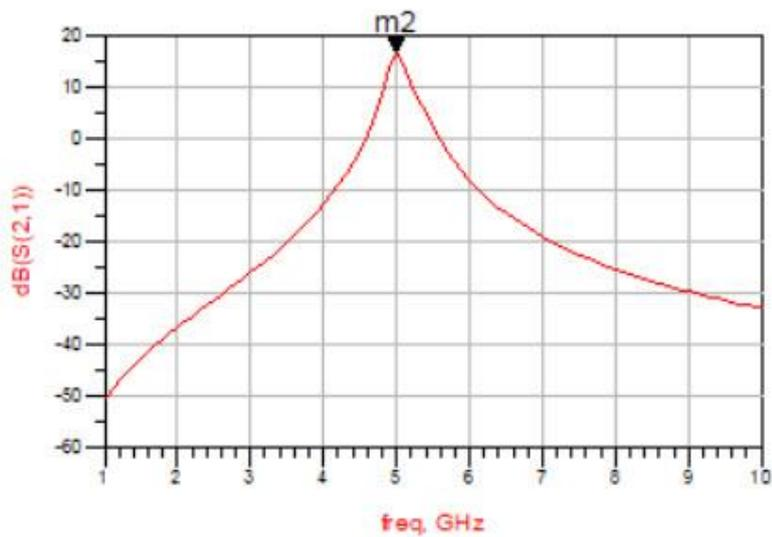
Figure (4-20):  $S_{21}$  Based on Optimized ( $L_S$  and  $L_g$ ) at 5 GHz DLNA
