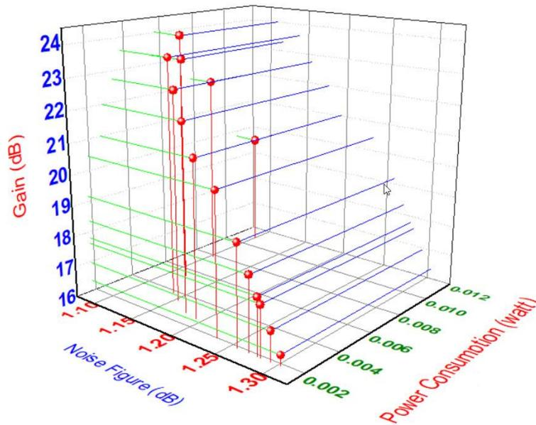
Figure(3-23): Three Dimensional Relationship Between Power , NF and Gain
