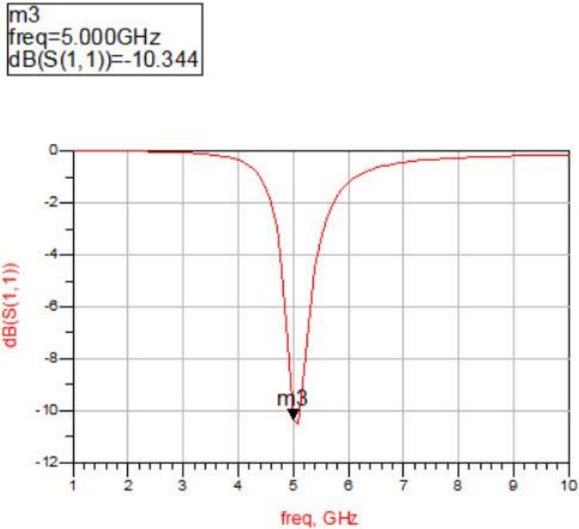
Figure (4-14): Mathematical Input Reflection Coefficients Result for 5 GHz DLNA
