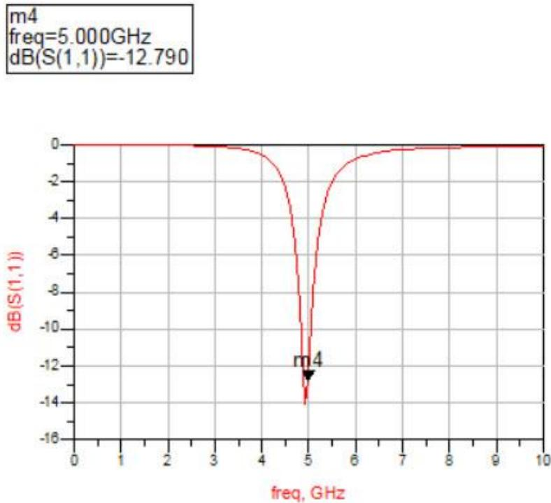
Figure (3-26): Optimized Input Return Loss Result for 5 GHz Single Ended LNA
