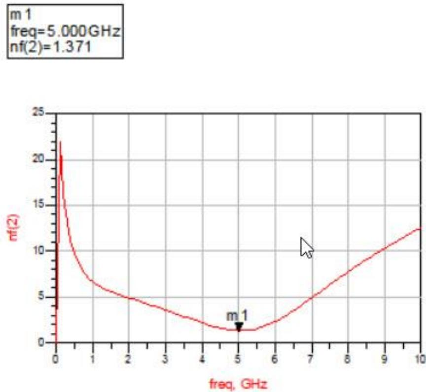
Figure (3-17): Mathematical NF Result for 5 GHz Single Ended LNA
