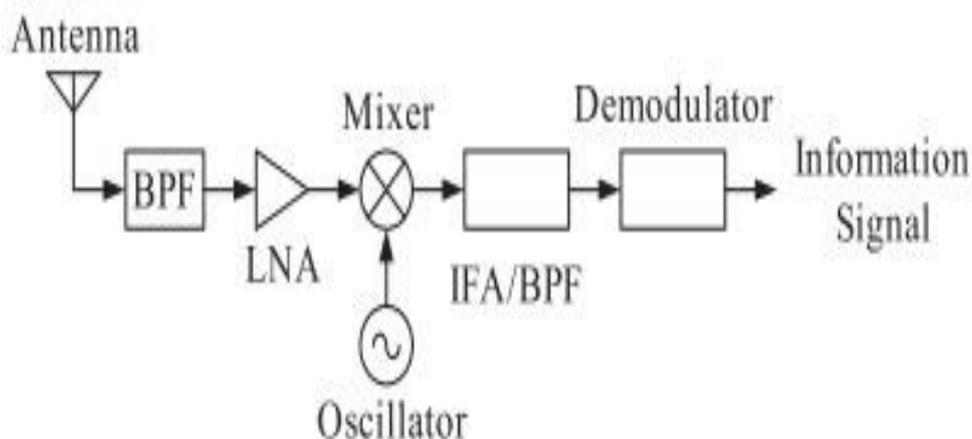
Figure (2-1): Block Diagram of a Typical RF Receiver
