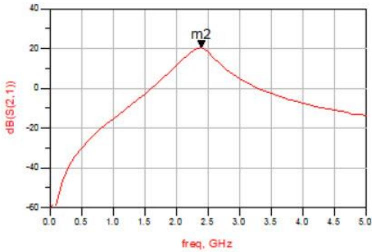
Figure (3-10): Power Gain Optimized Result for 2.4 GHz Single Ended LNA
