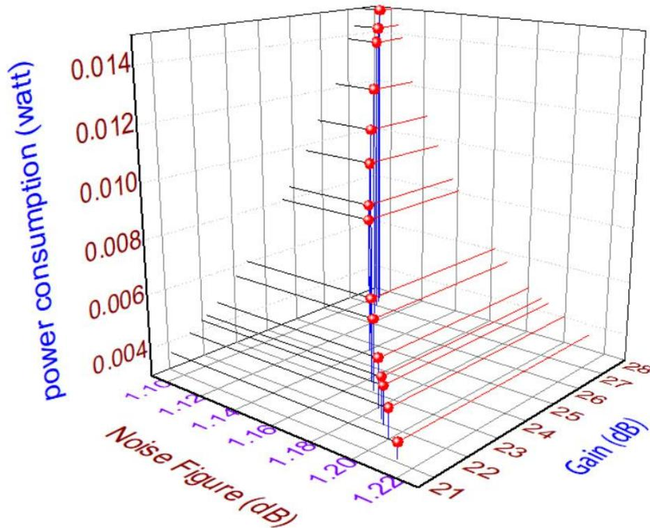
Figure (4-8): Three Dimensional Relationship Between NF, Gain ,Power Consumption for DLNA at 2.4 GHz
