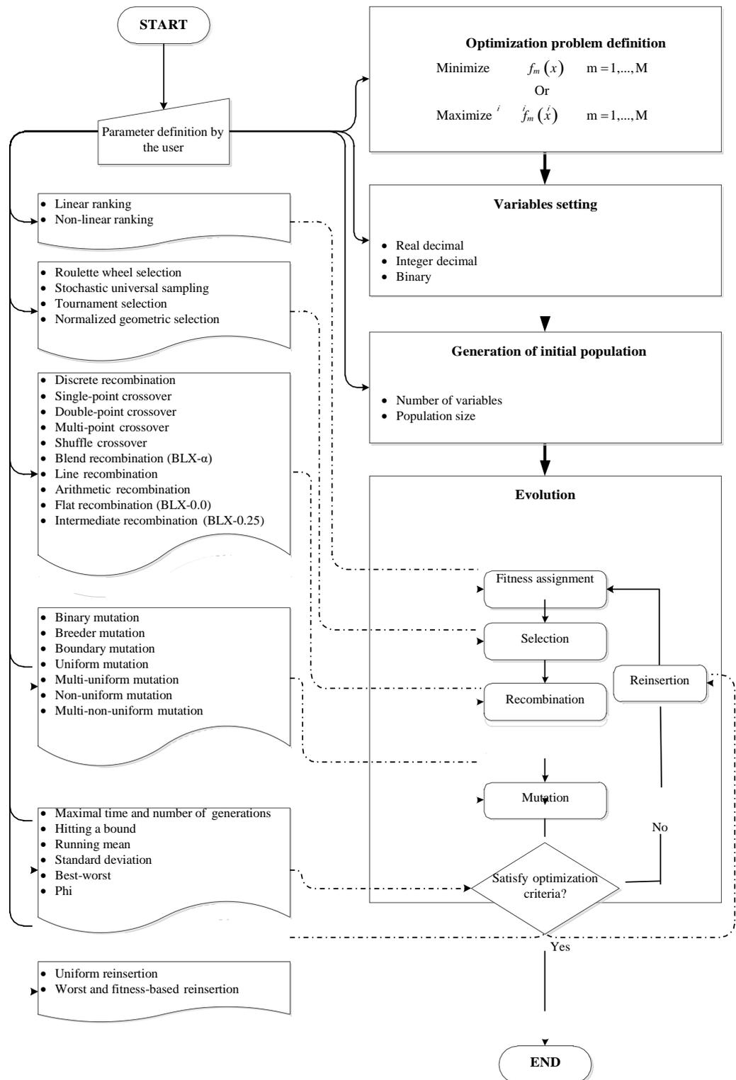
Figure (2-9): Operational Structure of the GA tool box [70].
