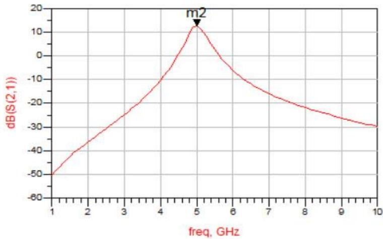
Figure (4-13): Mathematical Power Gain Result for 5 GHz DLNA
