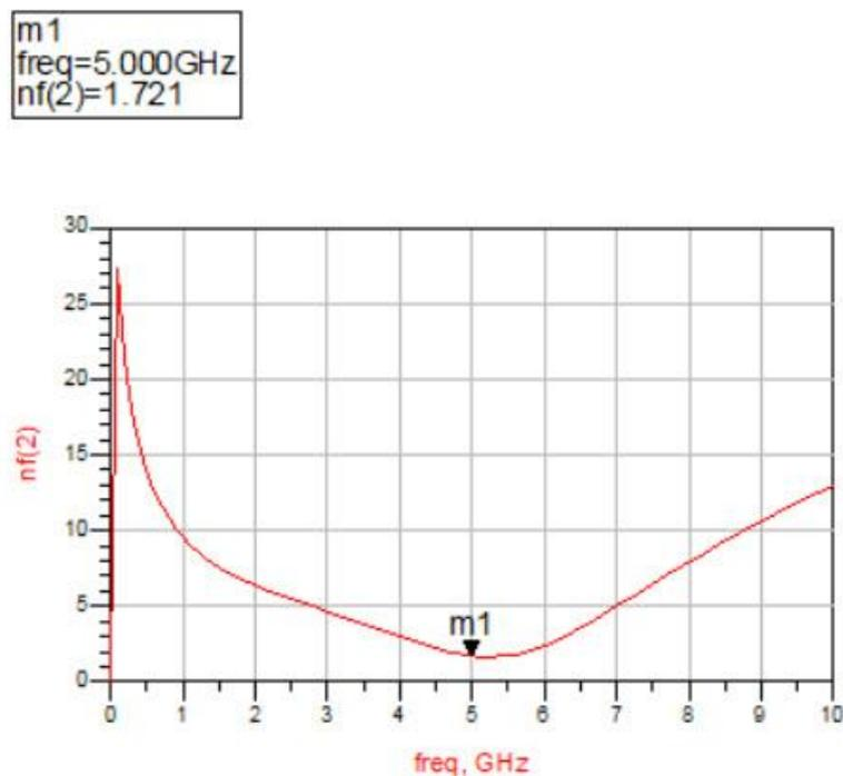
Figure (3-29): NF Based on Optimized ( $L_s$  and  $L_g$ ) at 5 GHz Single Ended LNA
