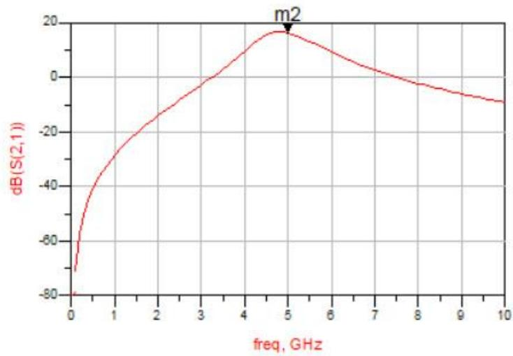
Figure (3-30):  $S_{21}$  Based on Optimized ( $L_s$  and  $L_g$ ) at 5 GHz Single Ended LNA
