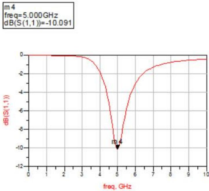
Figure (3-19): Mathematical Input Return Loss Result for 5 GHz Single Ended LNA
