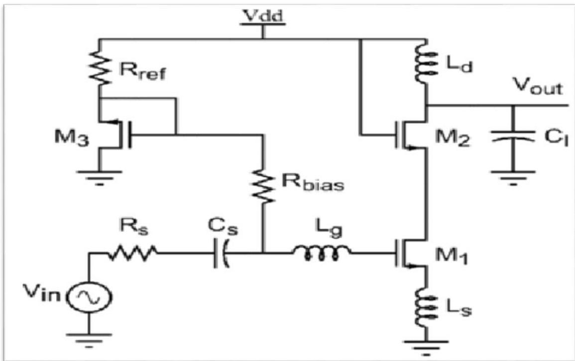
Figure (2-7): Cascode Source Degenerated LNA Topology [60]
