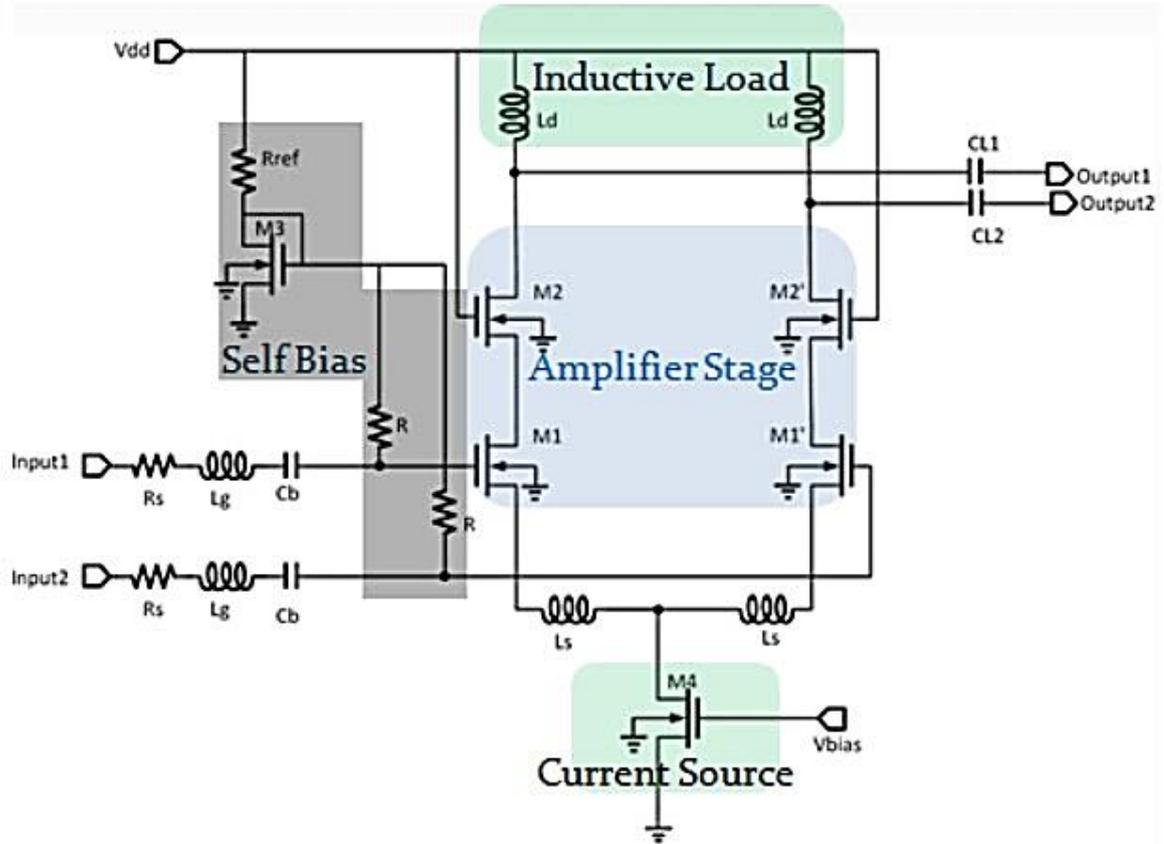
Figure (2-8): Differential LNA Topology [4]
