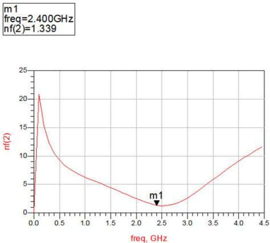
Figure (4-5): Optimized NF Result for 2.4 GHz DLNA
