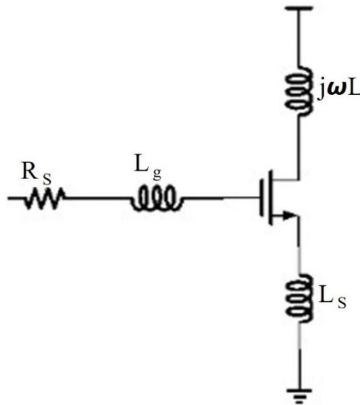
Figure (2-5): Common Source of Inductive Degeneration [4]
