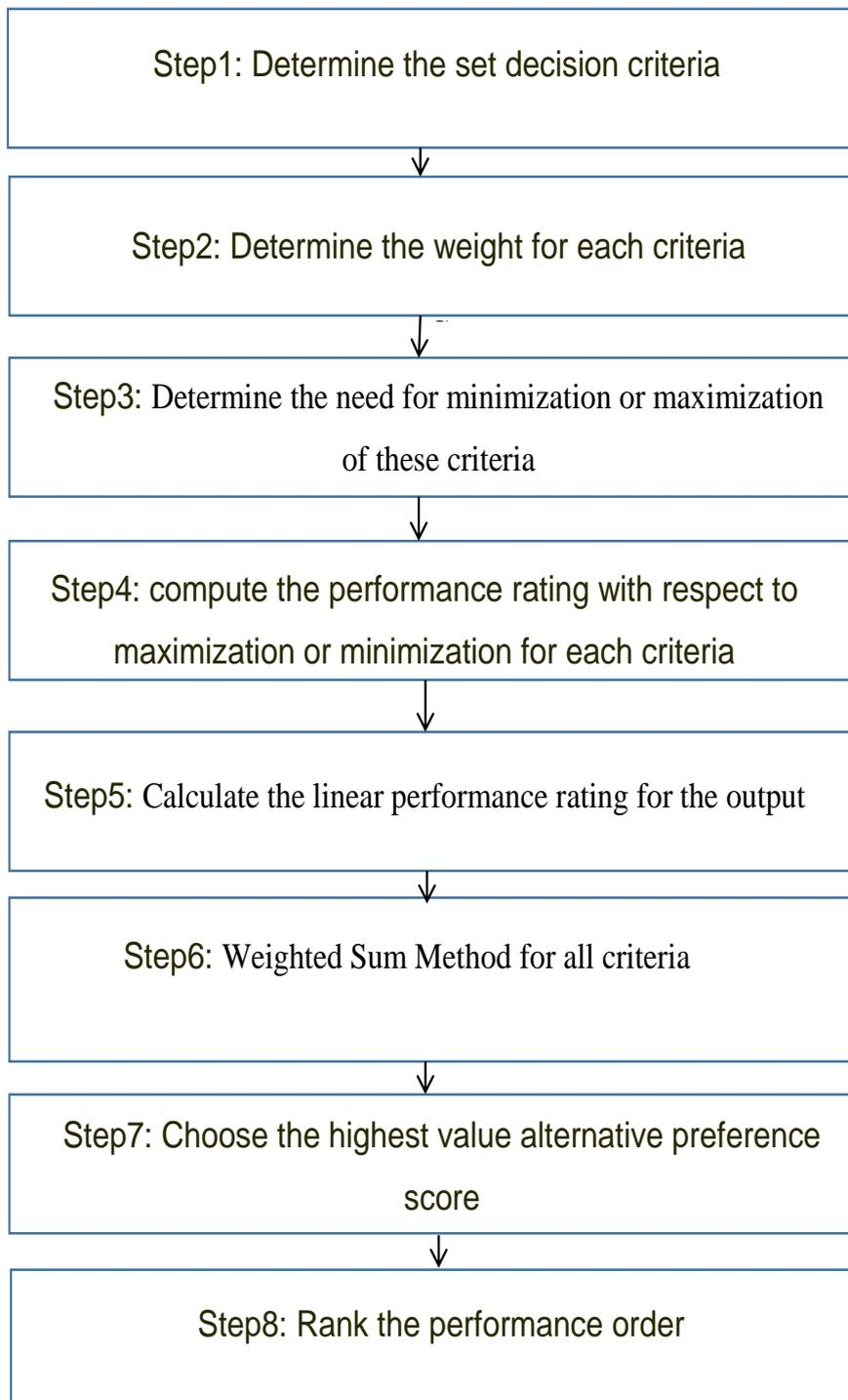
Figure (3-7 ): Flow Chart of Selection for Optimum Parameter Values
