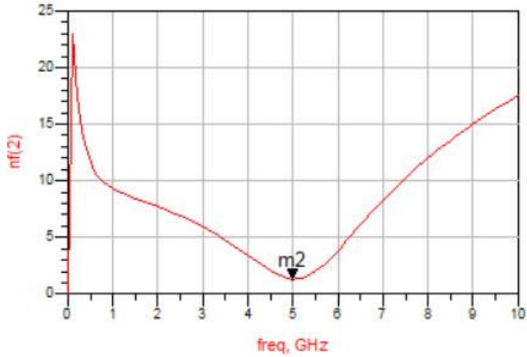
Figure (3-24): Optimized NF Result for 5 GHz Single Ended LNA
