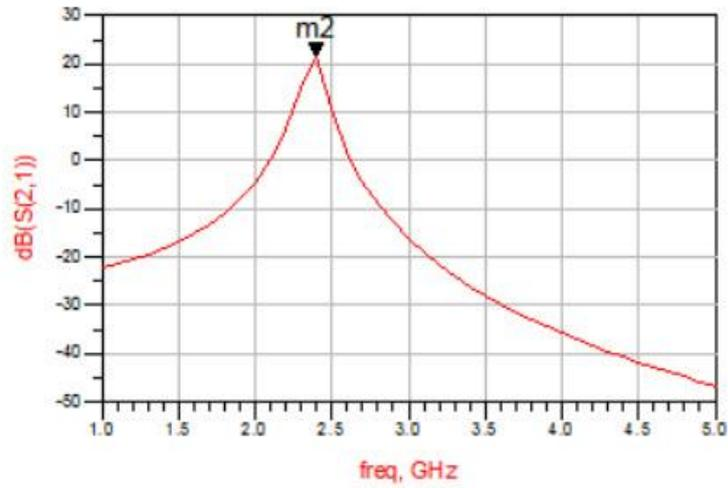
Figure (4-6): Optimized  $S_{21}$  Result for 2.4 GHz DLNA
