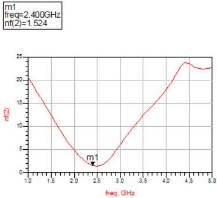
Figure (4-9): NF Based on Optimized ( $L_S$  and  $L_g$ ) at 2.4 GHz DLNA
