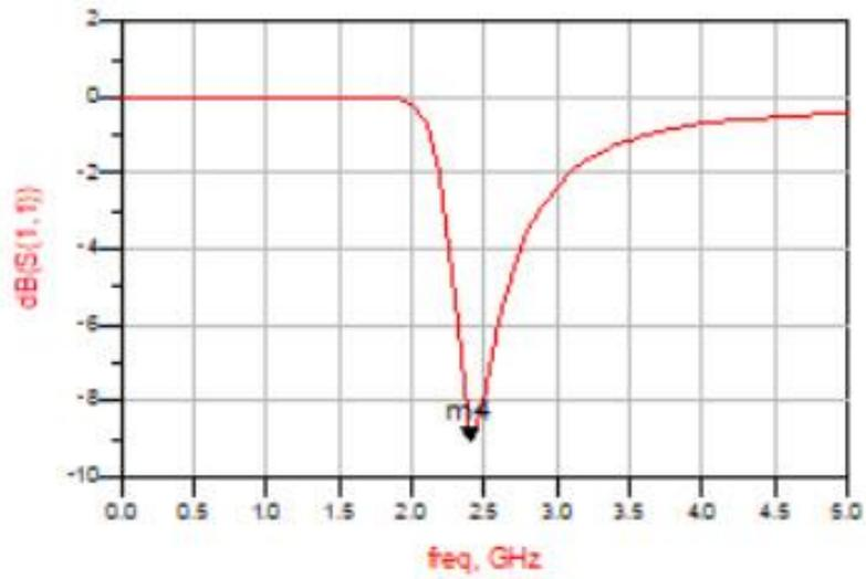
Figure (3-16):  $S_{11}$  Based on Optimized ( $L_s$  and  $L_g$ ) at 2.4 GHz Single Ended LNA
