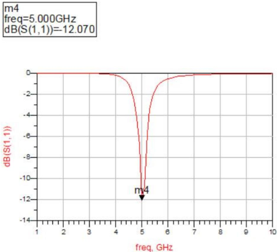
Figure( 4-18): Optimized The Input Reflection Coefficients ( $S_{11}$ ) Result for 5 GHz DLNA
