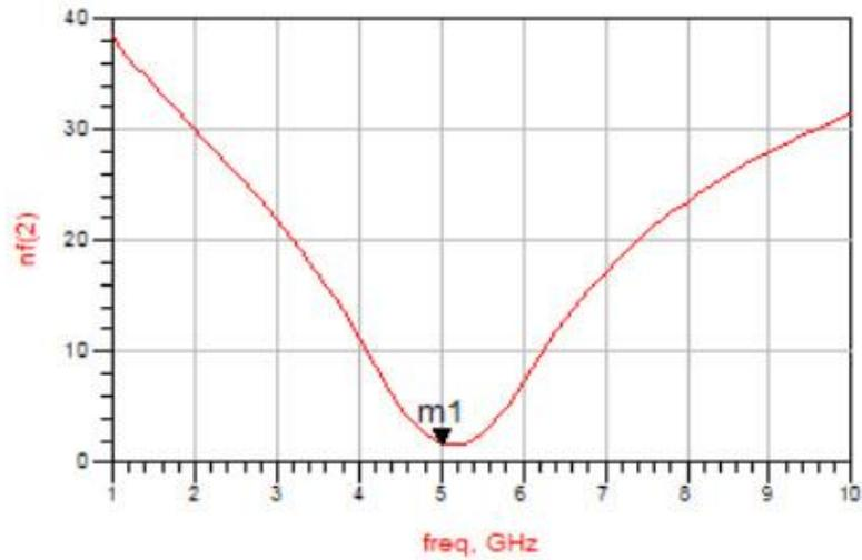
Figure (4-19): NF Based on Optimized ( $L_S$  and  $L_g$ ) at 5 GHz DLNA
