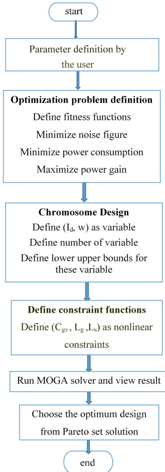
Figure (3-6): Flowchart of Genetic Algorithm Procedure Based on MATLAB
