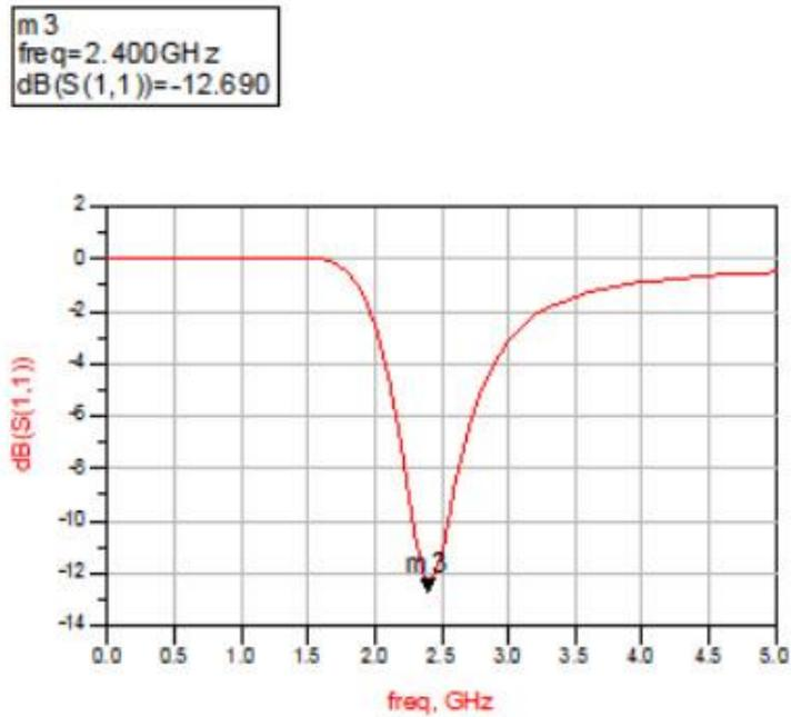
Figure (3-5): Mathematical Input Return Loss  $S_{11}$  for 2.4 GHz Single Ended LNA
