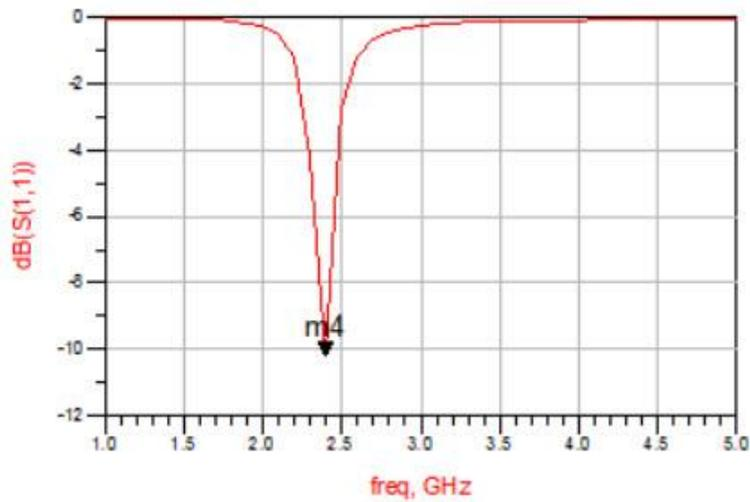
Figure (4-7): Optimized  $S_{11}$  Result for 2.4 GHz DLNA
