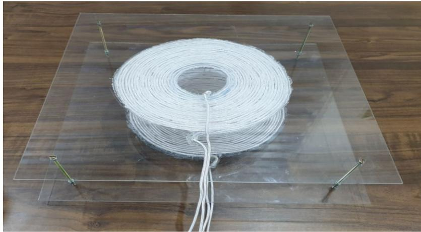
**Fig. 4.7** Circular Litz wire coils.
