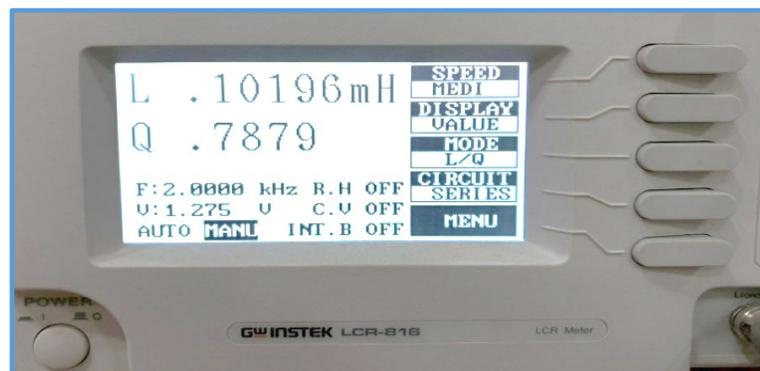
**Fig. 4.6** Laboratory measurement L for the inductive coil.
