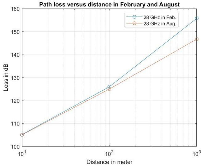
Figure 4.12: Path loss with the distance at 28 GHz.
