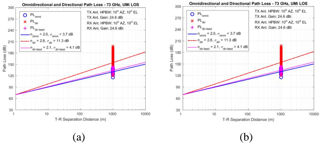
Figure 4.9: 73 GHz path loss in August during a) day b) night.
