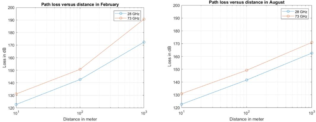
Figure 4.16: Path loss with the distance comparison between 28 and 73 GHz.
