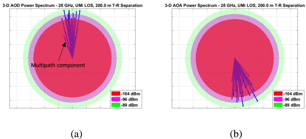
Figure 4.1: Multipath components with power levels and angles. a) Angles of departure (AOD). b) Angles of arrival (AOA).
