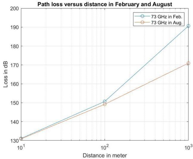
Figure 4.15: Path loss with the distance at 73 GHz.
