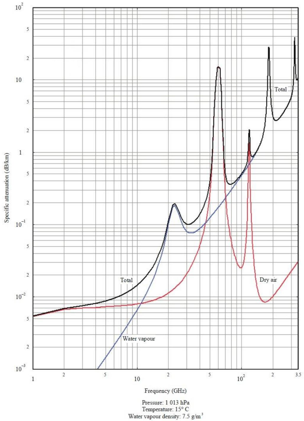
Figure 3.3: Atmospheric losses at millimeter wave band [62].
