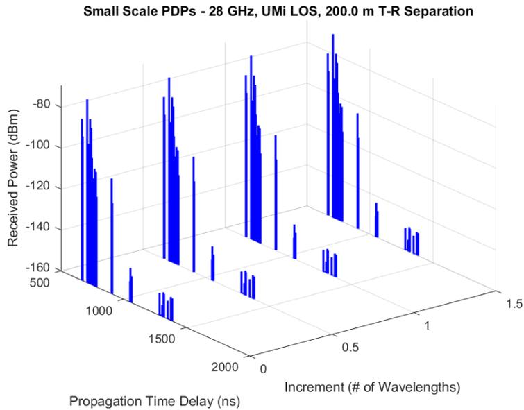
Figure 4.5: Power delay profile (PDP) of the receiving antenna.
