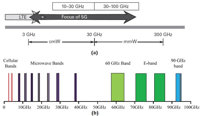
Figure 2.5: Radio spectrum a) frequency bands [7], b) frequency band allocation [47].
