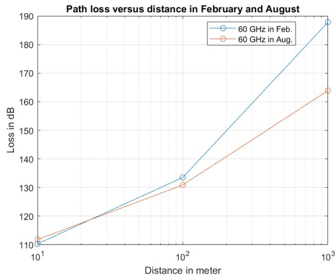
Figure 4.14: Path loss with the distance at 60 GHz.
