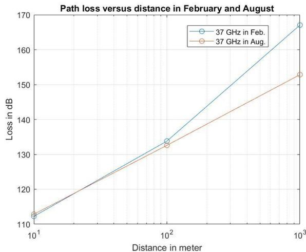
Figure 4.13: Path loss with the distance at 37 GHz.
