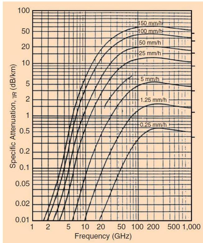
Figure 3.2: Losses due to rain at microwave and millimeter wave bands [58].
