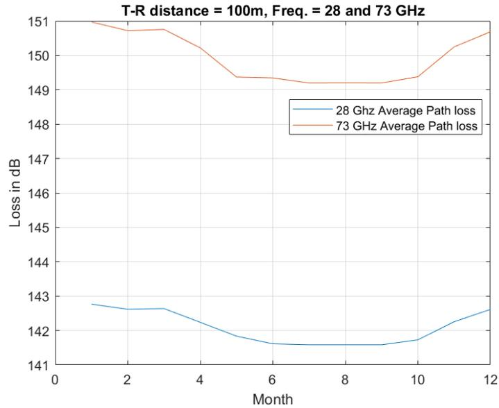
Figure 4.11: Path loss at 28 and 73 GHz for LOS case.
