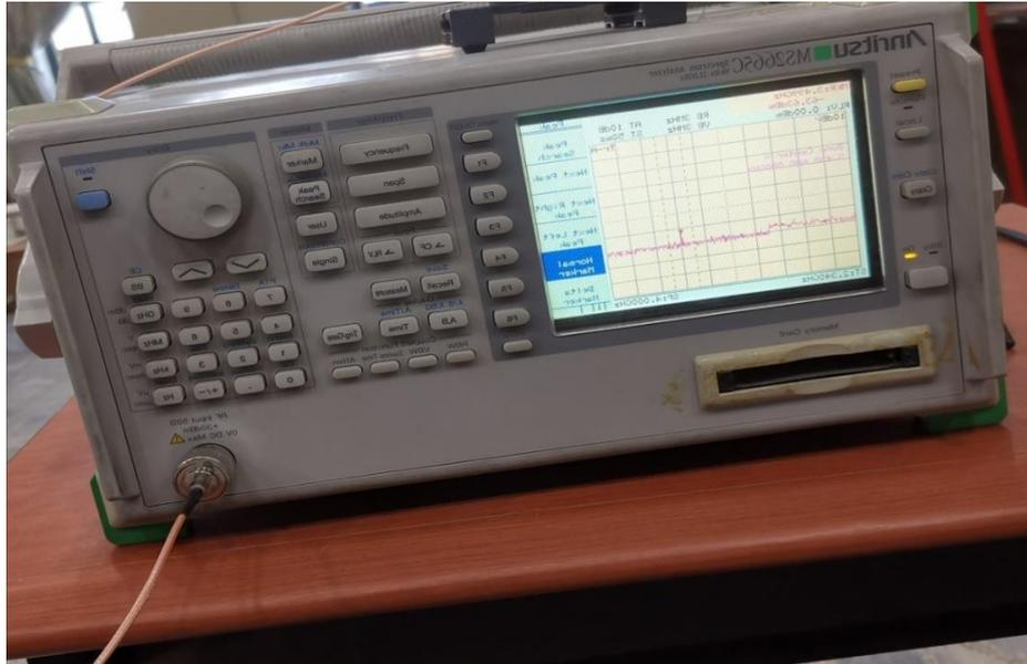
Figure 3.6: Anritsu spectrum analyzer.
