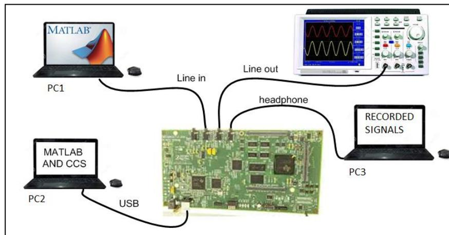
**Figure (4.1): Input and output devices connected to TMS320C6713 KDS KIT**
