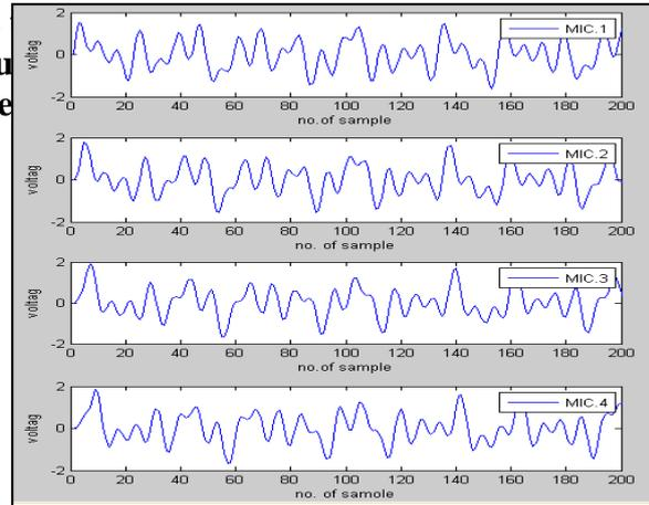
As well as the first microphone assumed as a reference, its input will be the summation of the four signals without delay, while the input of the other microphones will be the summation of the four signals but each signal with delay calculated by the four calculation blocks.
