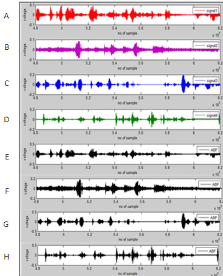
**Figure (3.32): (ABF) (speech inputs signals) & outputs signals in case (4 MICs, 4source) (non uniform phase and amplitude ABF)**
