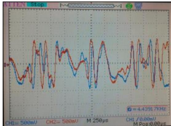
**Figure (4.13):**The input tone signals to each microphone in case (2 MICs, 4 sources)
