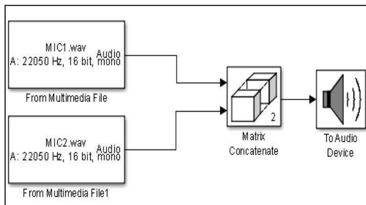
**Figure (4.3): MATLAB-SIMULINK circuit that used to generate the two microphone signals (in Pc1)**
