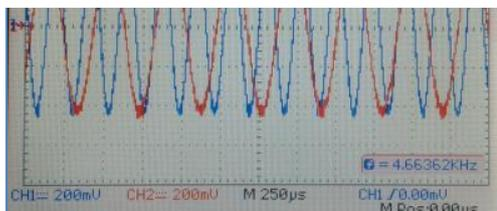
Figure (4.6): The input tone signals to each microphone in case (2 MICs, 2 sources)
