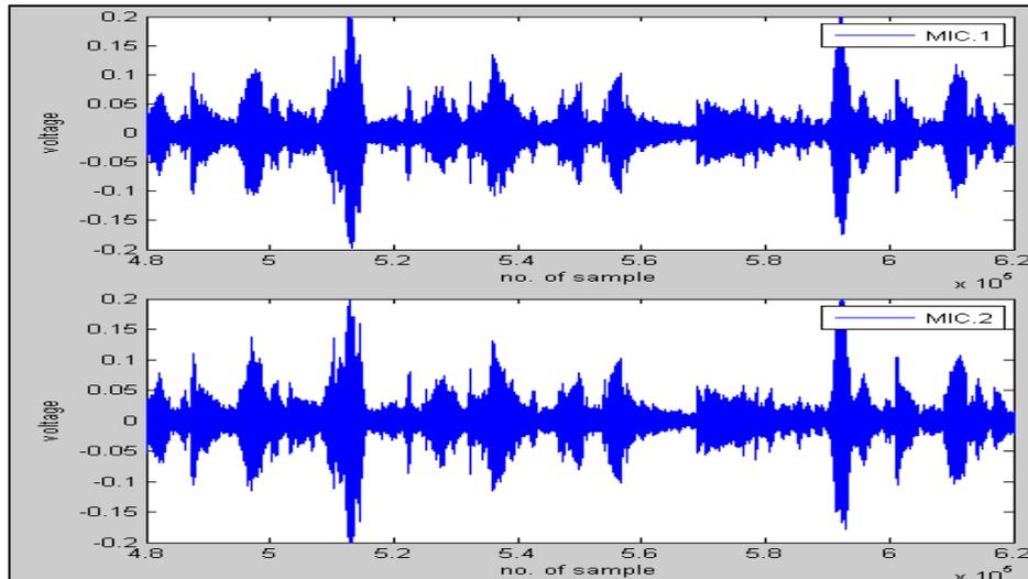
**Figure (3.8): The input speech signals to each microphone in case (2 MICs, 2 sources)**
