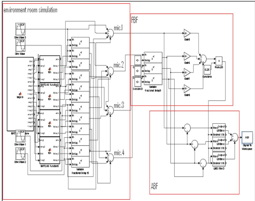
**Figure (3.28): Simulation system for 4 MICs, 4 sources non-uniform phase and amplitude tested by single tone signals**
