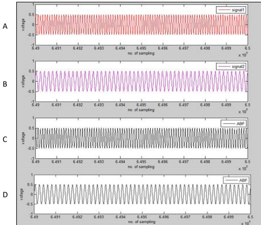
**Figure (3.6): (ABF) (single tone inputs signals) & output signals
