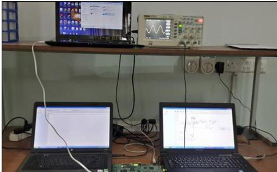
**Figure (4.2): TMS320C6713 KDS KIT based hardware implementation system of the (MABF) system using two microphones**
