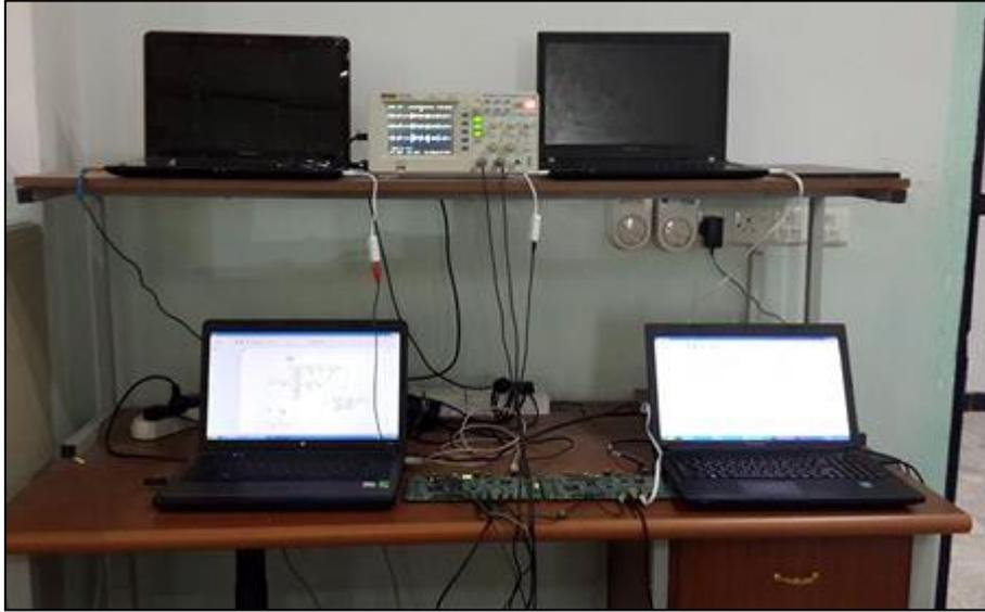
**Figure (4.20): Two TMS320C6713 KDS KITs based hardware implementation system of the (MABF) system using four microphones**
