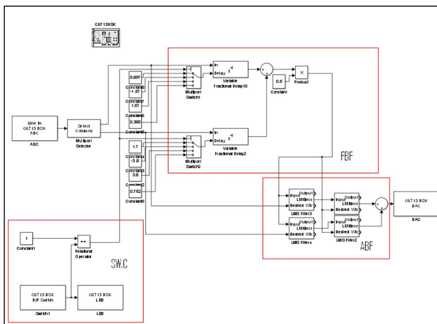
**Figure (4.23): Part1 Simulation system for 2 MICs, 4 sources using TMS320C6713KDS KIT1 (PC2)**
