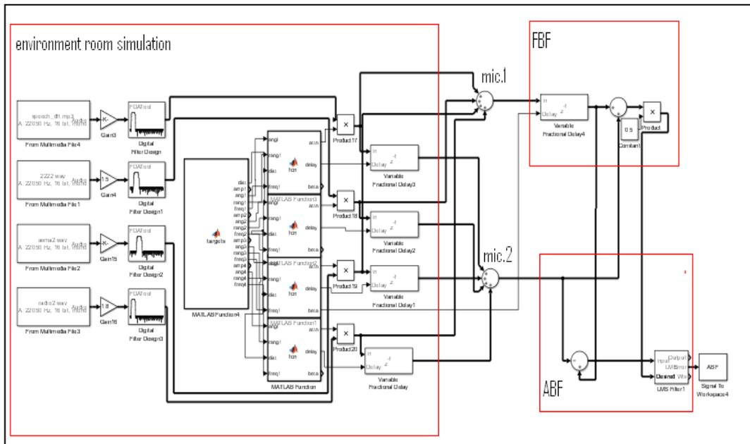
**Figure (3.16): Simulation system for 2 MICs, 4 speech sources uniform phase and amplitude**
