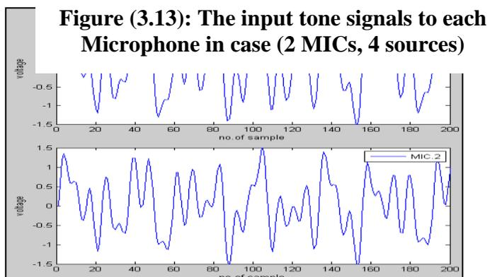
As well as the first microphone assumed as a reference, his output will be the summation of the four signals without delay, while the output of the second microphone must be the summation of the four signals but each signal with delay calculated by the four calculation blocks.
