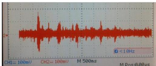
**Figure (4.10):The input speech signals to each microphone in case (2 MICs, 2 sources) Ch1 (blue line) is MIC1 signal (ref.MIC) Ch2 (red line) is MIC2 signal**
