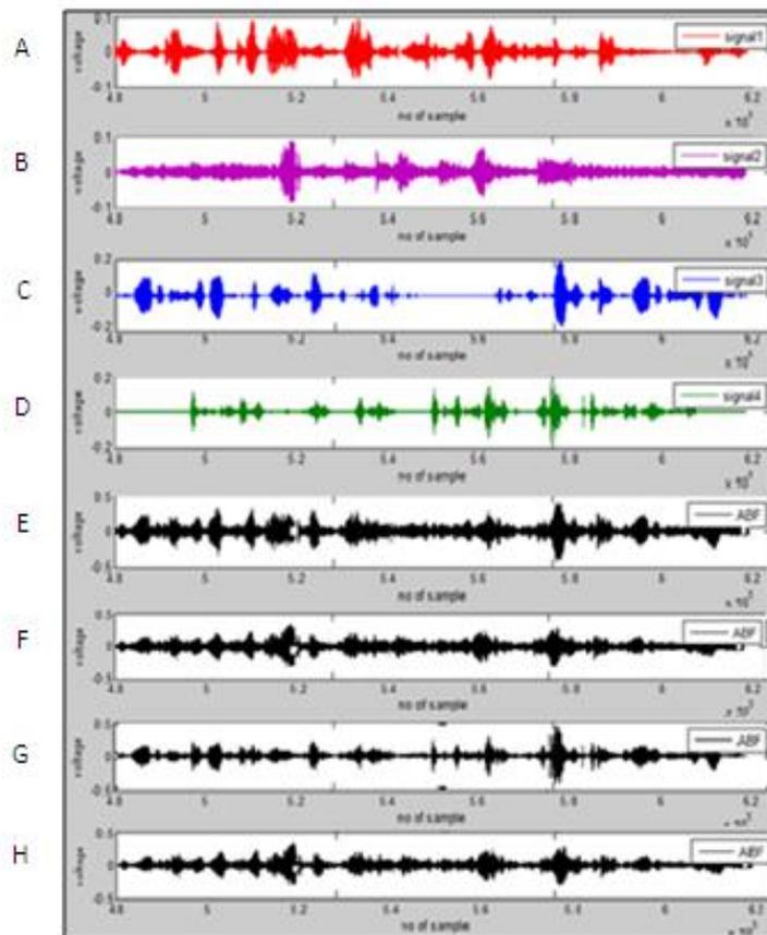
**Figure (3.27): (ABF) (speech inputs signals) & outputs signals in case (4 MICs, 4source) (uniform phase and amplitude ABF)**
