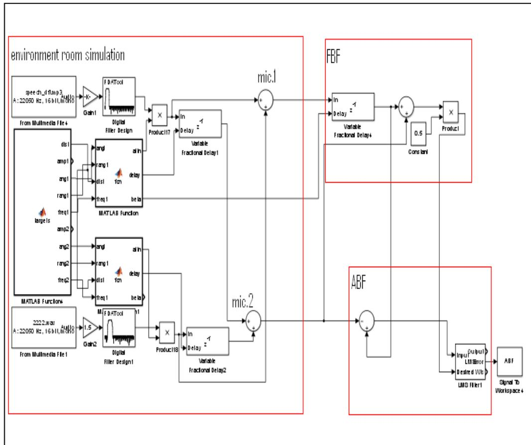
**Figure (3.7): Simulation system for 2 MICs, 2 sources tested by speech signals**
