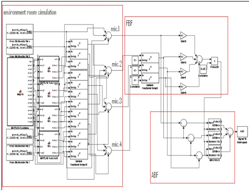
**Figure (3.31): Simulation system for 4 MICs, 4 speech sources nonuniform phase and amplitude beamforming system tested by speech signals**
