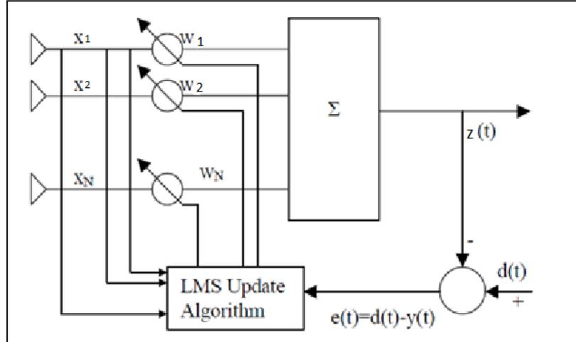
Figure (2.5): LMS adaptive beamforming network [28].
