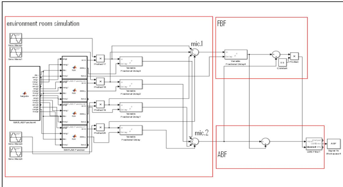
**Figure (3.11): Simulation system for 2 MICs, 4 sources uniform phase and amplitude tested by single tone signals**
