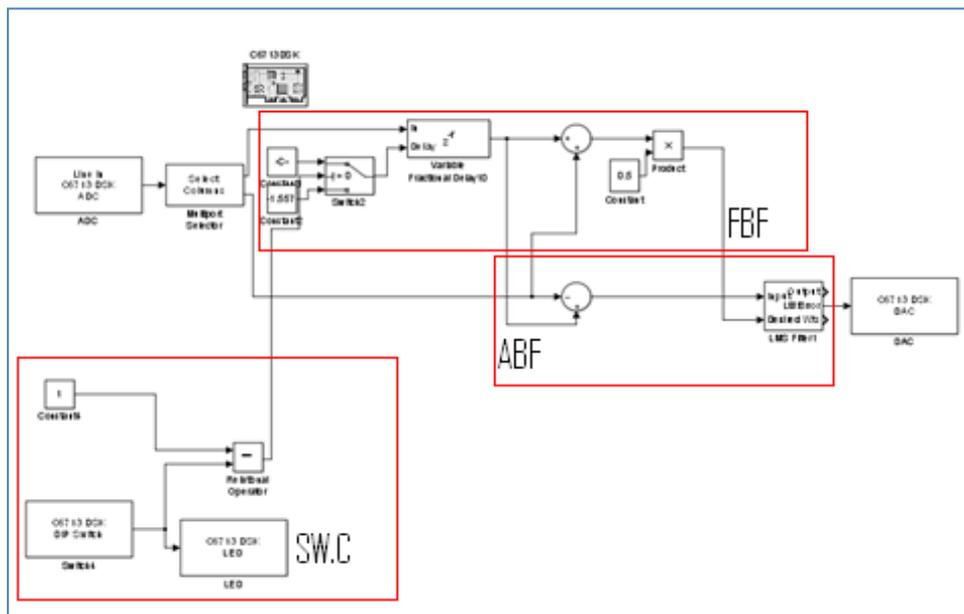
**Figure (4.7): Simulation system for 2 MICs, 2 sources using TMS320C6713KDS KIT**
