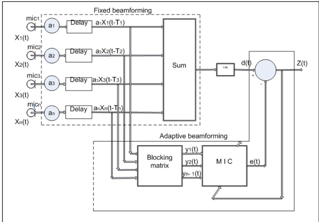
**Figure (2.4): Diagram of GSC with delay and sum**
