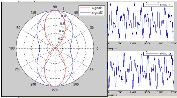
**Figure (3.3): The array factor for signal1 and signal2 at broadside (2 MICs, 2 sources)**
