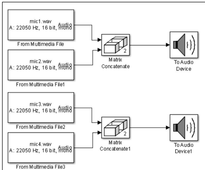
**Figure (4.21): MATLAB-SIMULINK circuit that used to generate the four microphone signals (in PC1)**
