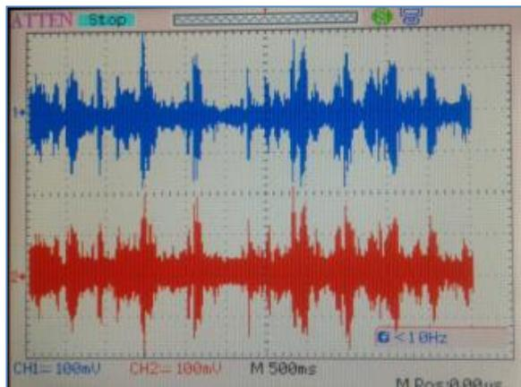
**Figure (4.17): The input speech signals to each microphone in case (2 MICs, 4 sources)
