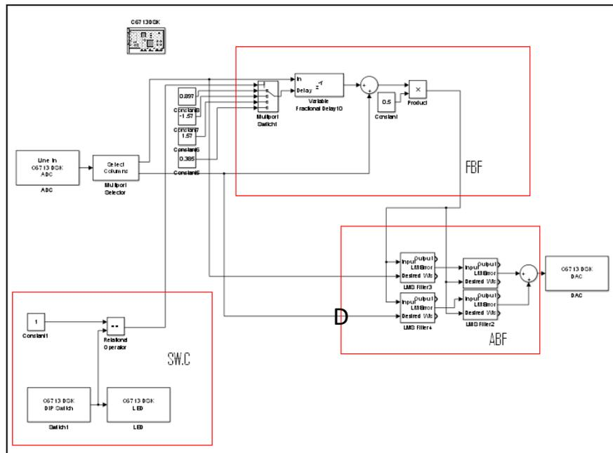
**Figure (4.24): Part2 Simulation system for 2 MICs, 4 sources using TMS320C6713KDS KIT2 (PC3)**
