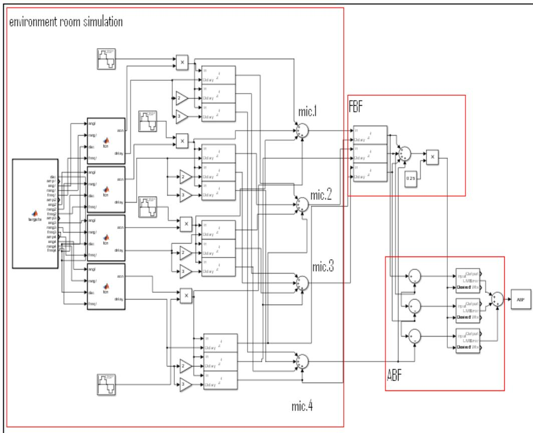
**Figure (3.20): Simulation system for 4 MICs, 4 sources uniform phase and amplitude tested by single tone signals**
