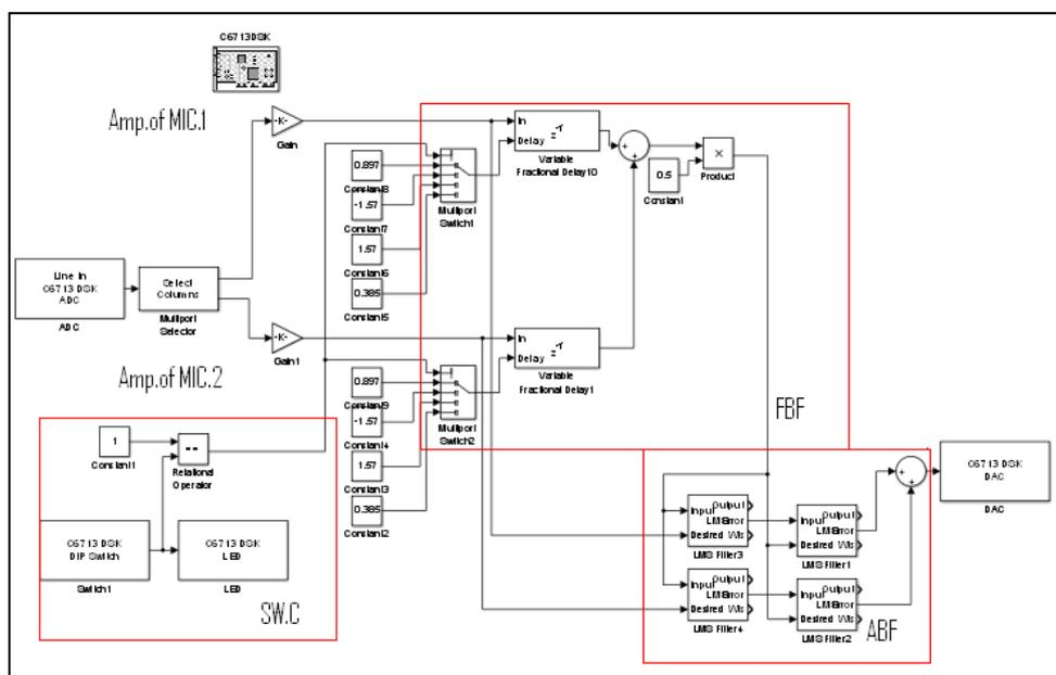
simulation circuit shown in figure (4.29) used to generate the KIT2 code in PC3.
