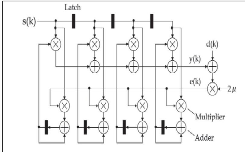
Figure (2.6): Structure of the 4-tap LMS adaptive filter [35]
