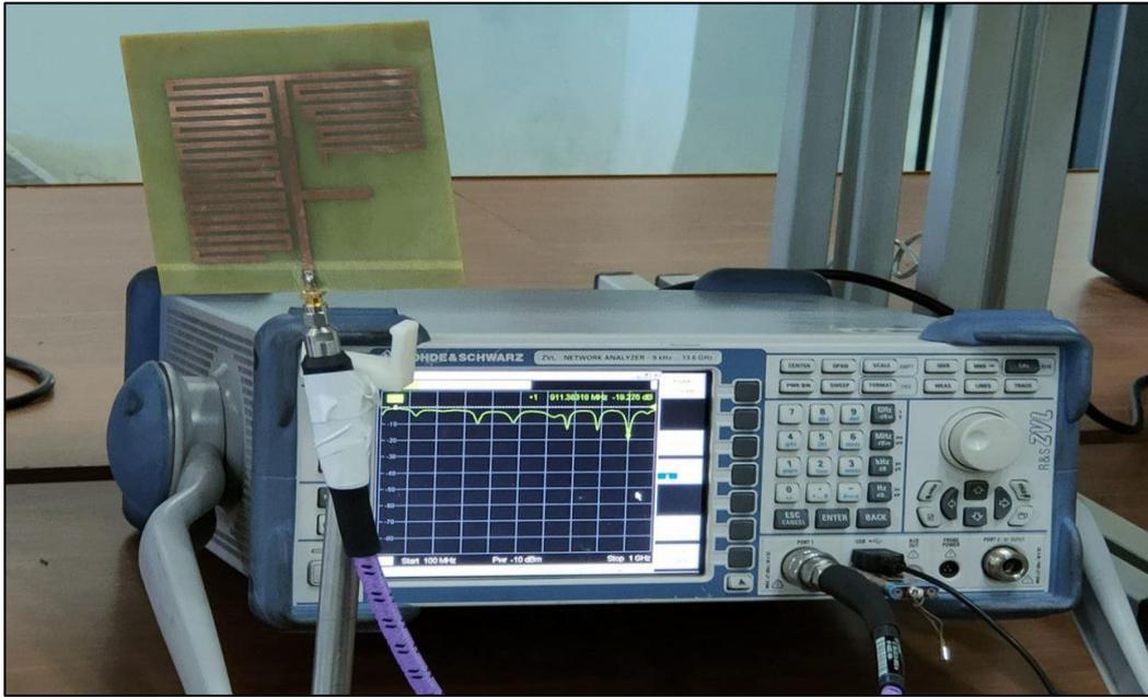
**Fig. 4.25. Experimental set up for measuring the antenna S-parameters.**
