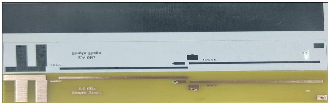
Fig.3.57: Rectifier circuit layout for fabrication.
