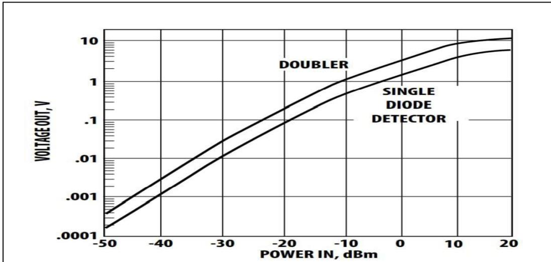
Fig.2.2: Voltage doubler output as sweep of input power compared with single diode rectifier [50].
