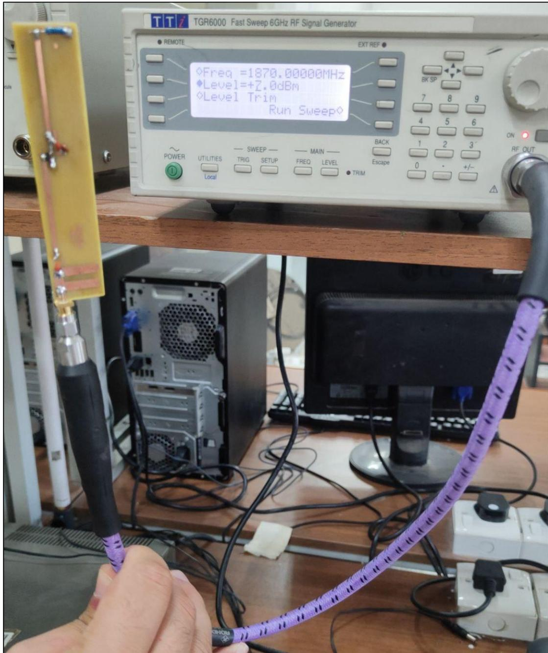
Fig.3.61: Photograph of the experimental setup showing the measurement of  $V_{dc}$  ( $V_{out}$ ) Versus  $P_{in}$  (dBm).
