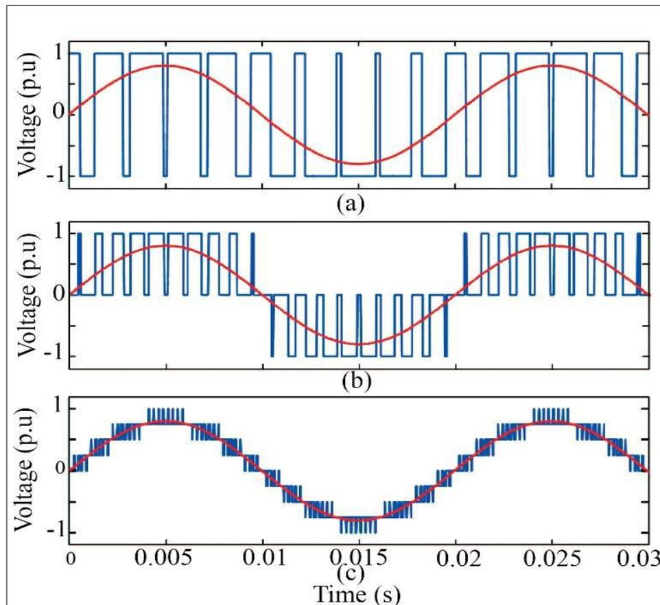
Figure 2.2 The Output Phase Voltage for (a): Two-level Inverter, (b): Three-level Inverter, (c) Nine-level Inverter [12]
