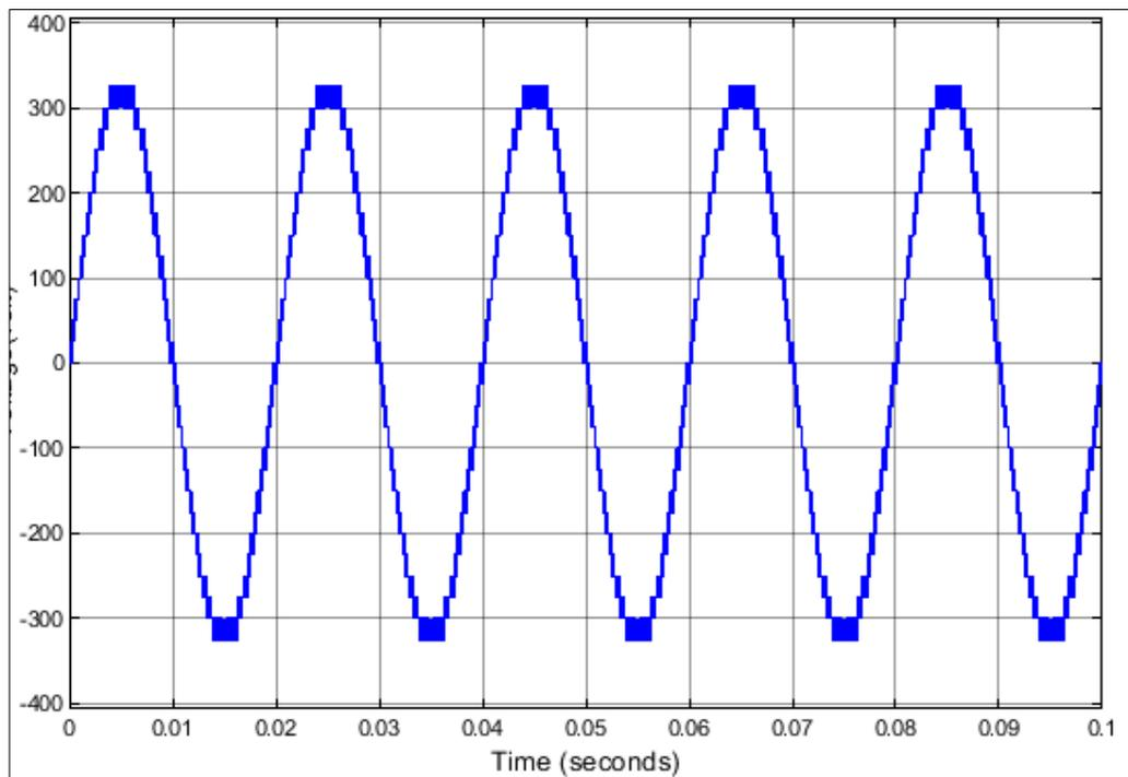
Figure 3.7 The Generated Waveform of SPWM without Filter
