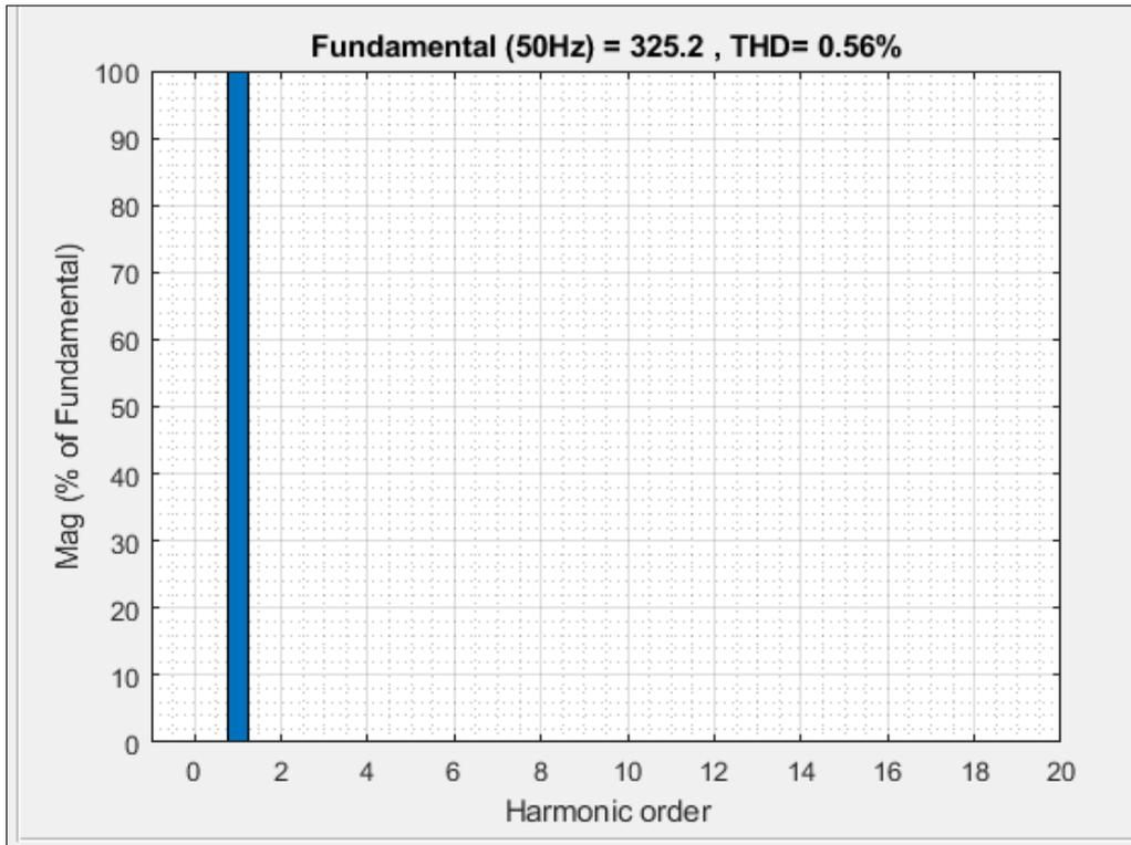
Figure 3.10 THD of the SPWM Output Signal with Filter
