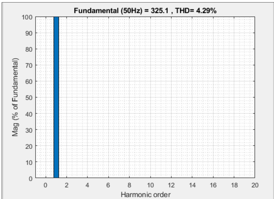
Figure 3.9 THD of the SPWM Output Signal without Filter
