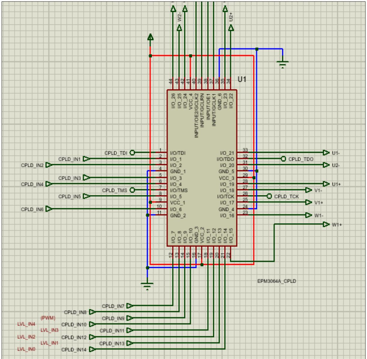
Figure 4.5 EPM3064A\_CPLD IC Circuit Connections
