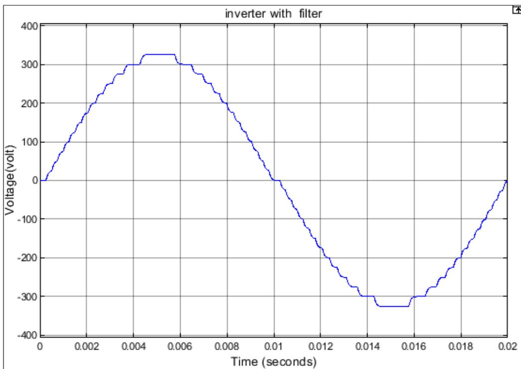
Figure 3.12 The Generated Waveform of SHE with Filter
