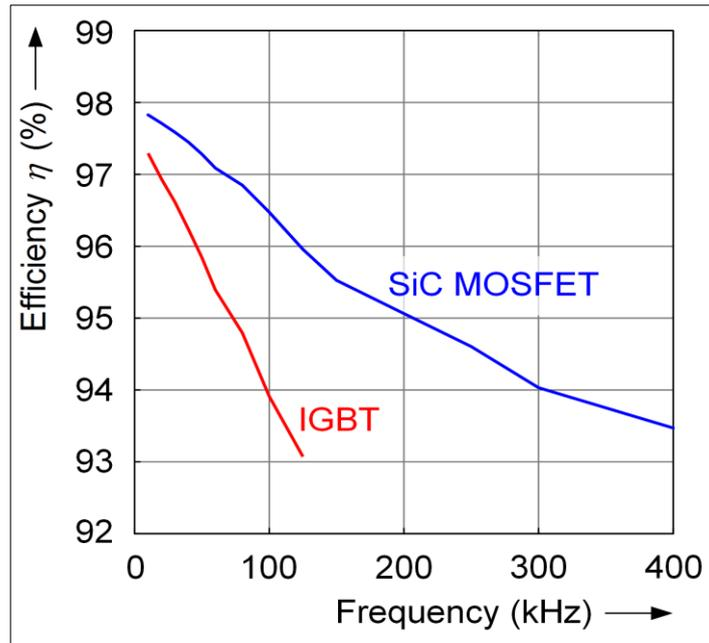
Figure 2.8 Measured Efficiency Over Switching Frequency at  $P_{out} = 10\text{kW}$  [36]
