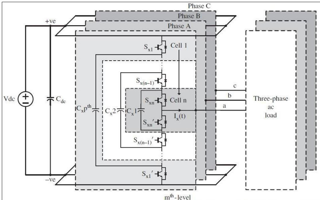
Figure 2.5 Three-Phase n-cell Multilevel Flying Capacitor Inverter [44].
