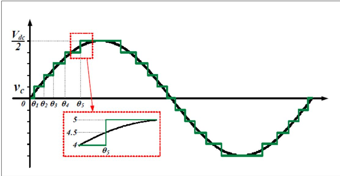
Figure 2.16 Operational Principle of the Nearest Level Modulation [64]
