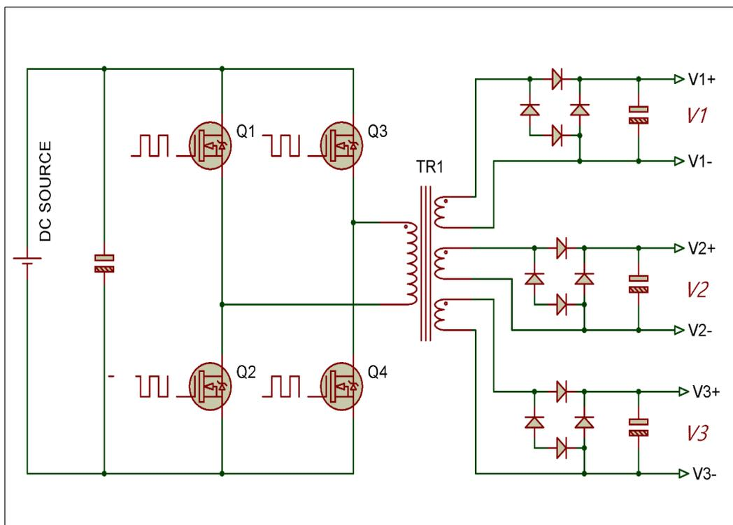
Figure 4.13 Single Source to Three Isolated Sources, 1kW DC-to-DC Converter
