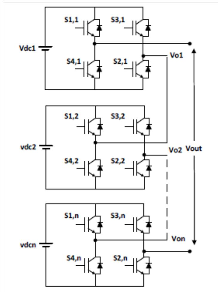
Figure 2.6 Cascaded H-bridge Multilevel Inverter (CHBMLI) [47]
