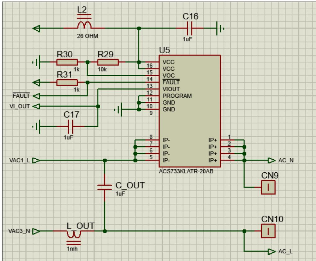
Figure 4.12 Schematic Design of the Current Measurement Circuit
