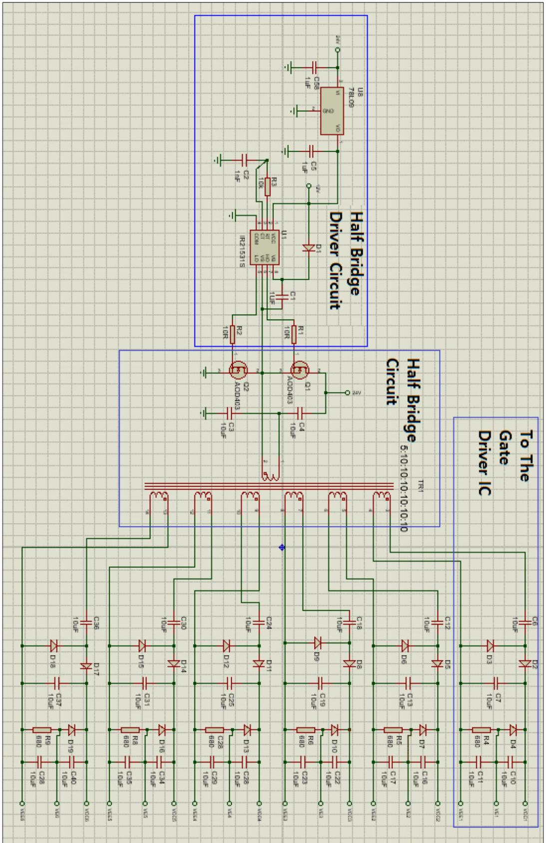
Figure 4.8 Stages of Generating +18, -5 Volt to Drive the Gate
