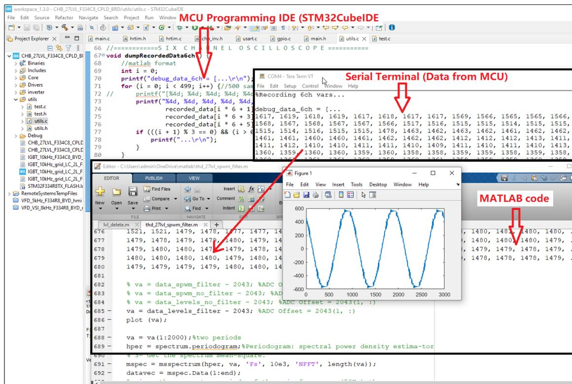
Figure 4.18 A Screenshot from the PC Showing the Process of Collecting Waveform Data Samples from the Inverter
