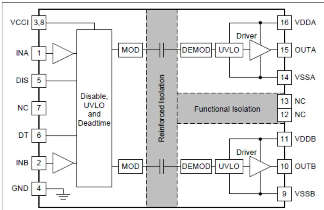
Figure 4.6 The Block Diagram of UCC21520DWR IC
