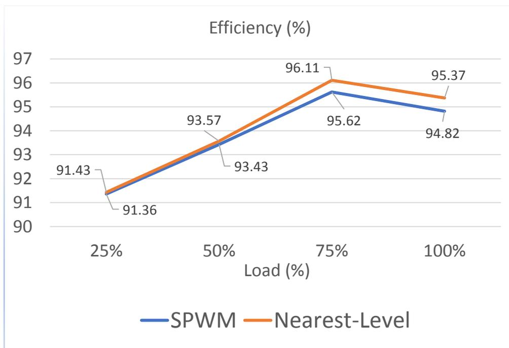
Figure 4.21 Efficiency over Multiple Load Steps for SWPM and Nearest-level Modulation Methods.
