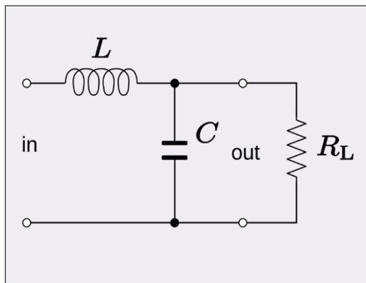
Figure 3.2 Typical Architecture of LC Filter
