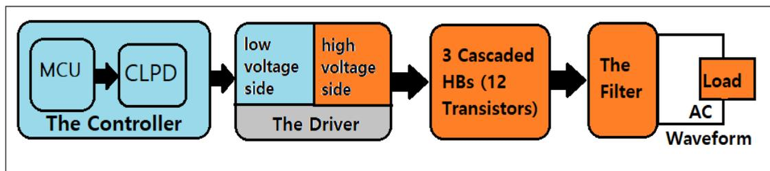
Figure 4.1 The Flow Chart of the Inverter Process
