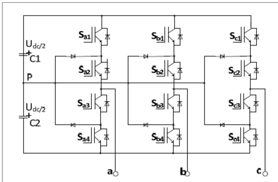
Figure 2.3 NPC Three Level Inverter Topology [41]
