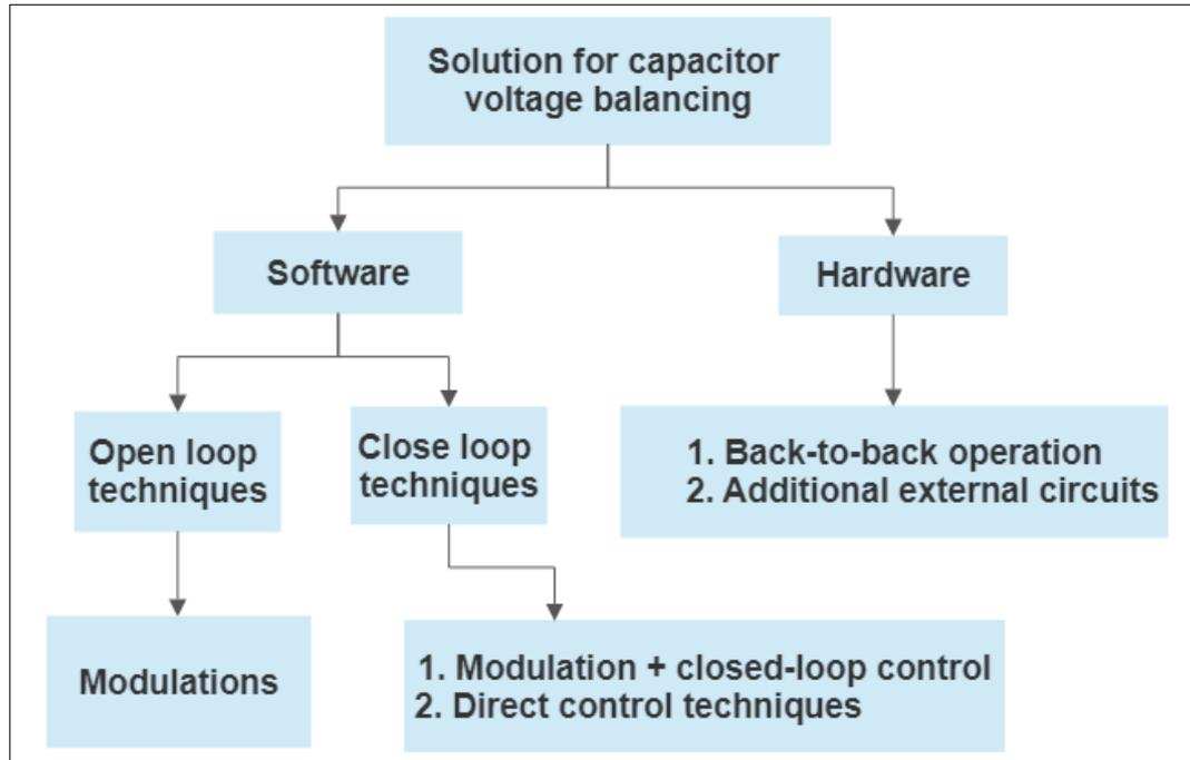
Figure 2.4 Classification of the Solutions for DC-link Capacitor Voltage Balancing in NPC Topology [42]
