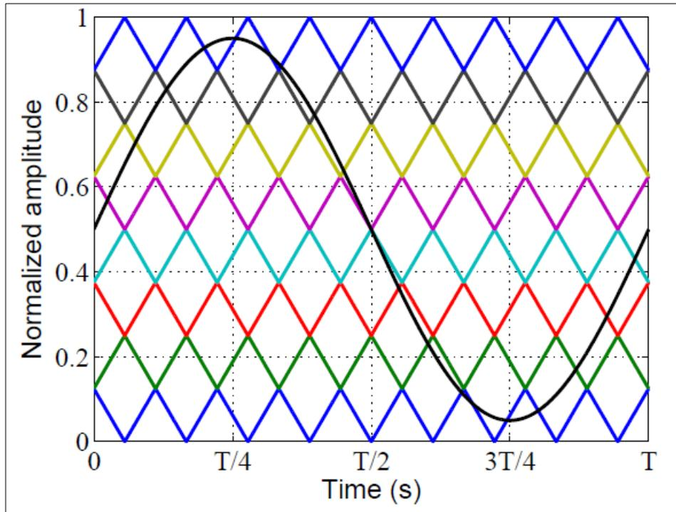
Figure 2.14 Alternative Phase Opposition Disposition PWM [61]
