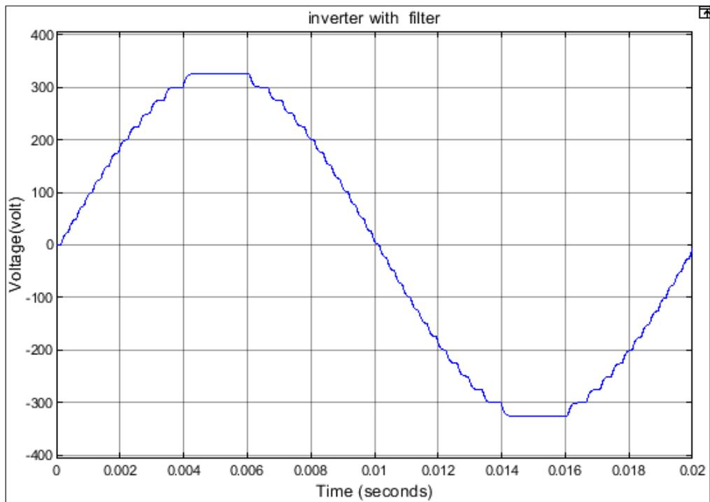
Figure 3.4 The Generated Waveform of Nearest Level with Filter
