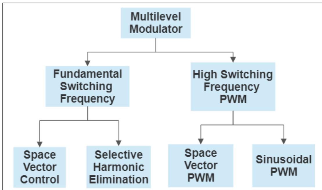
Figure 2.9 Classification of Modulation Methods [56]
