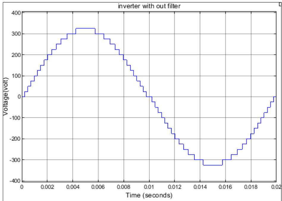
Figure 3.11 The Generated Waveform of SHE without Filter
