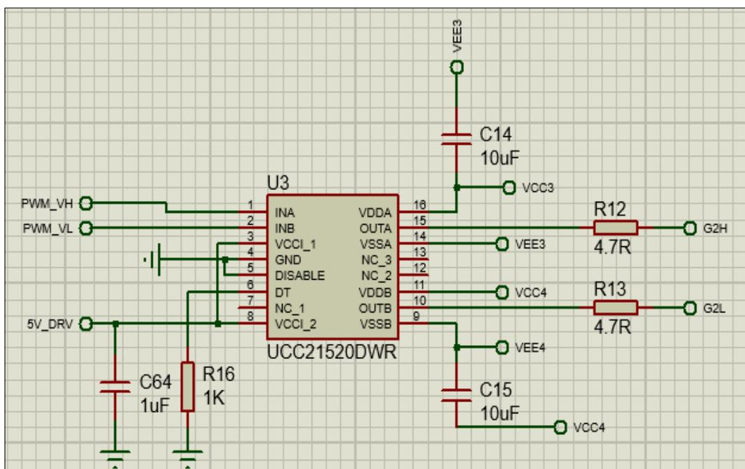
Figure 4.7 Design of the Isolated Dual Channels UCC21520DWR IC using Proteus Software
