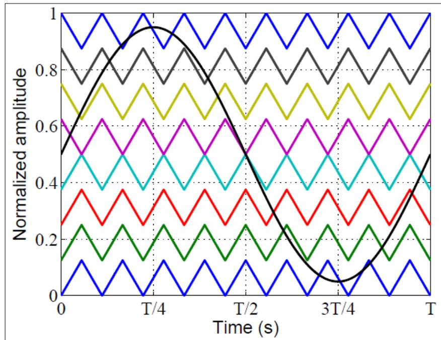
Figure 2.13 Phase Opposition Disposition PWM [61]
