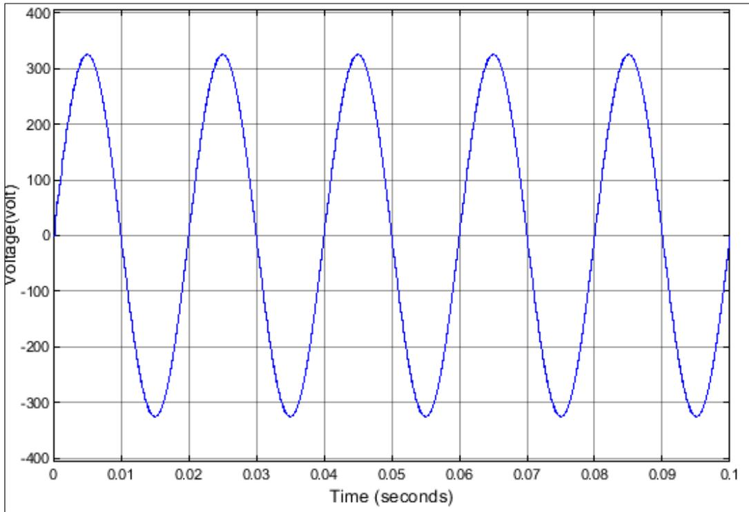
Figure 3.8 The Generated Waveform of SPWM with Filter
