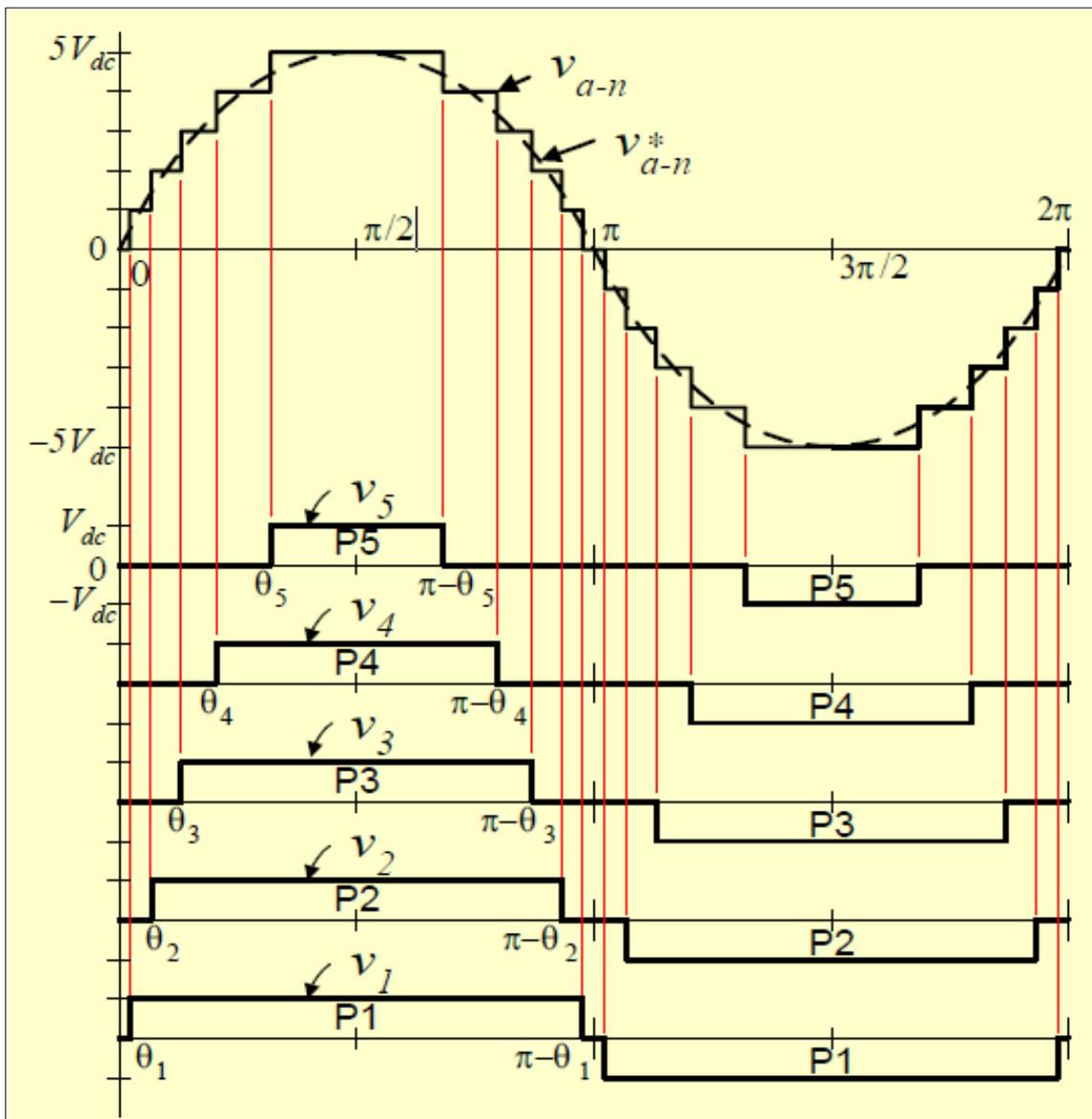
Figure 2.10 Output Waveform of an 11-level Cascade Multilevel Inverter [58]
