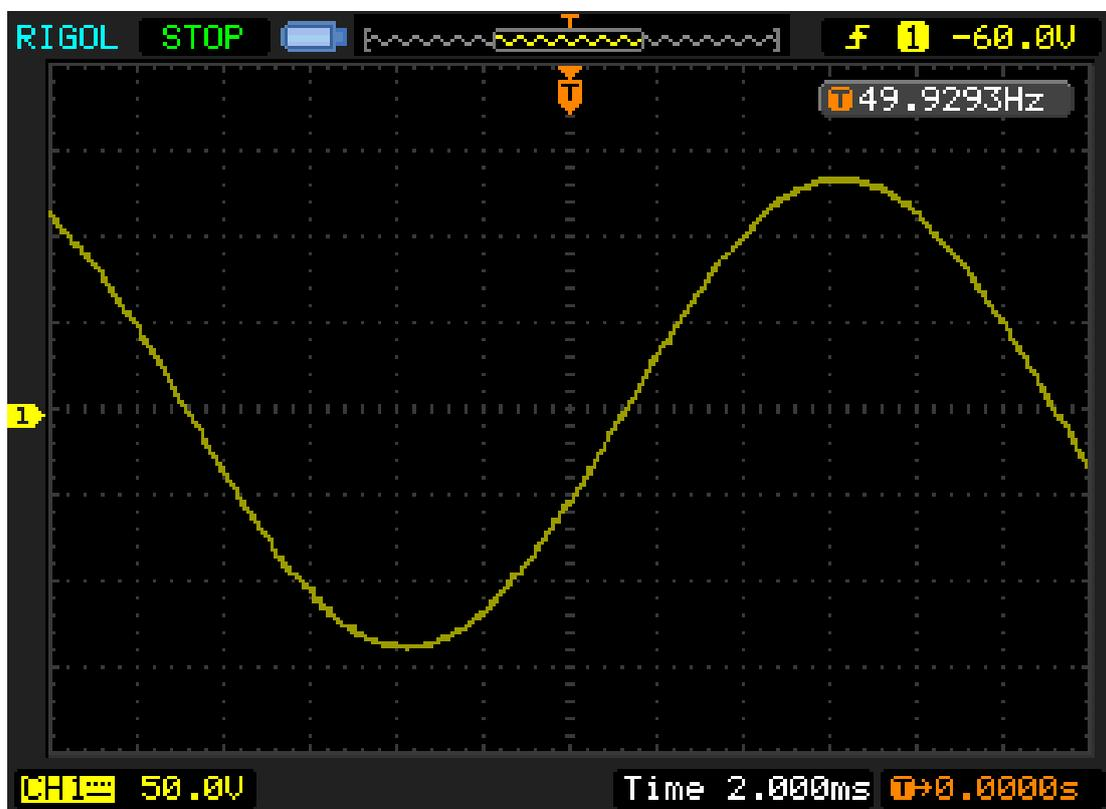
Figure 4.20 Inverter Output Waveform Using Nearest-level Modulation Combined with PWM (with LC Filter), Scale: 100:200k $\Omega$  Potentiometer ( $2 \times 50 = 100\text{V/div}$ )
