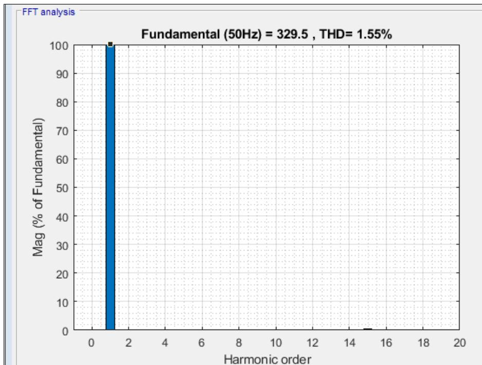
Figure 3.6 THD of The Nearest Level Output Signal with Filter
