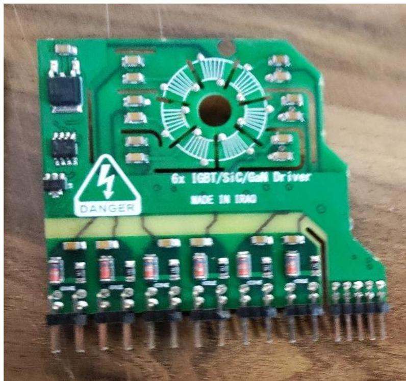
Figure 4.9 The Driver Power Supply Board
