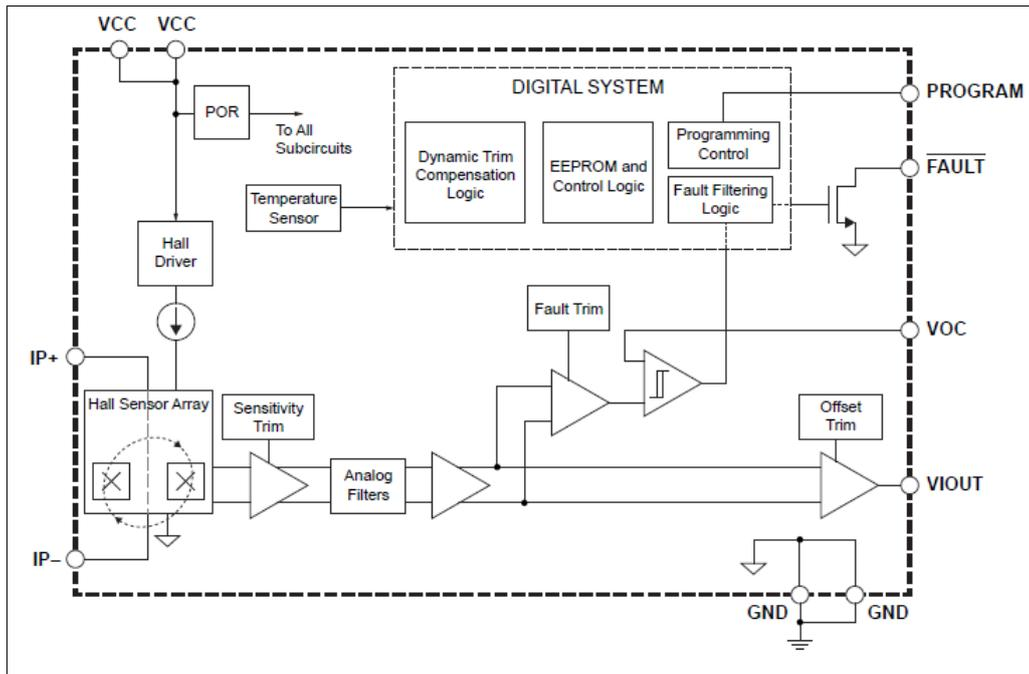
Figure 4.11 Functional Block Diagram of ACS733KLATR-20AB IC [67]
