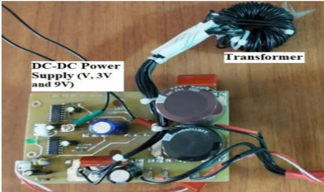
Figure 4.16 Complete DC-DC Converter Circuit
