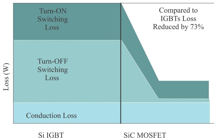
Figure 2.7 Loss Comparison of SiC-MOSFET and Si-IGBT
