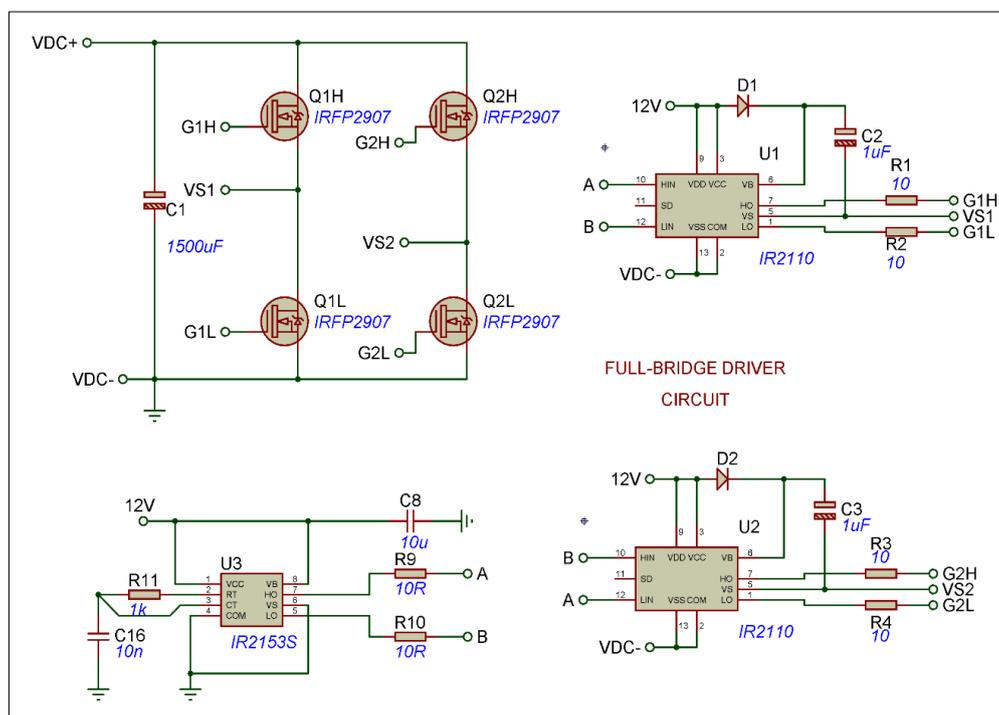
Figure 4.14 Primary Side Circuit of The DC-DC Converter
