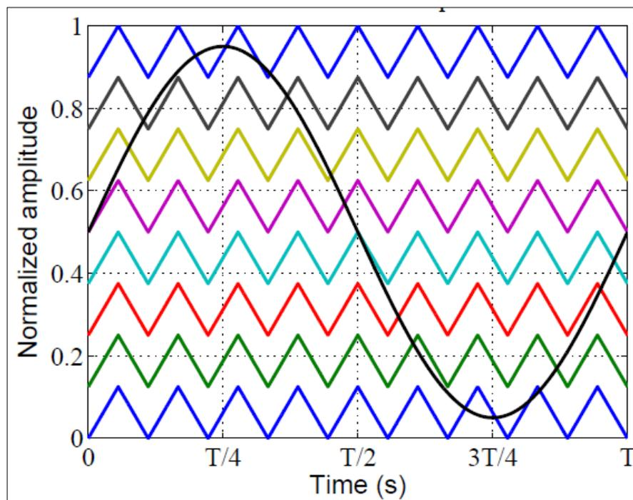
Figure 2.12 Phase Disposition PWM [61]
