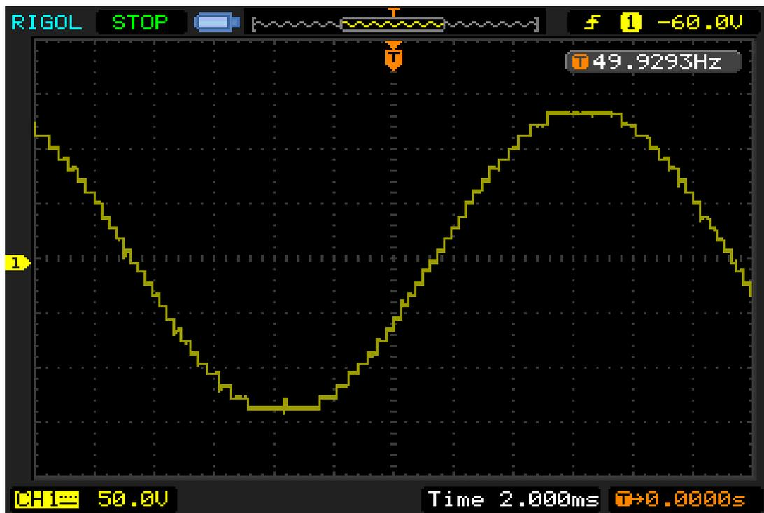
Figure 4.19 Inverter output Waveform using Nearest-level Modulation (w/o filter), Scale: 100:200kΩ Potentiometer (2×50= 100V/div)
