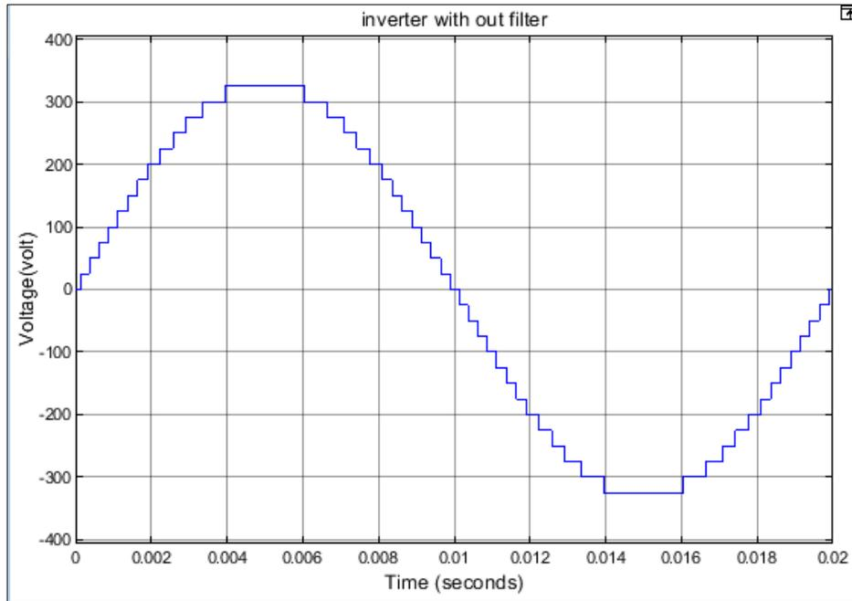
Figure 3.3 The Generated Waveform of Nearest Level without Filter
