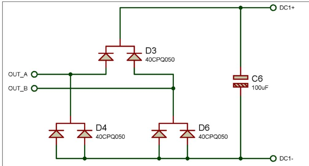
Figure 4.15 Secondary Rectifier Circuit for V1 (25VDC) Output
