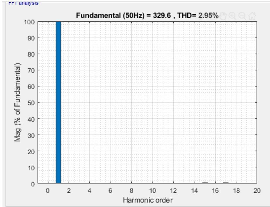
Figure 3.5 THD of the Nearest Level Output Signal without Filter
