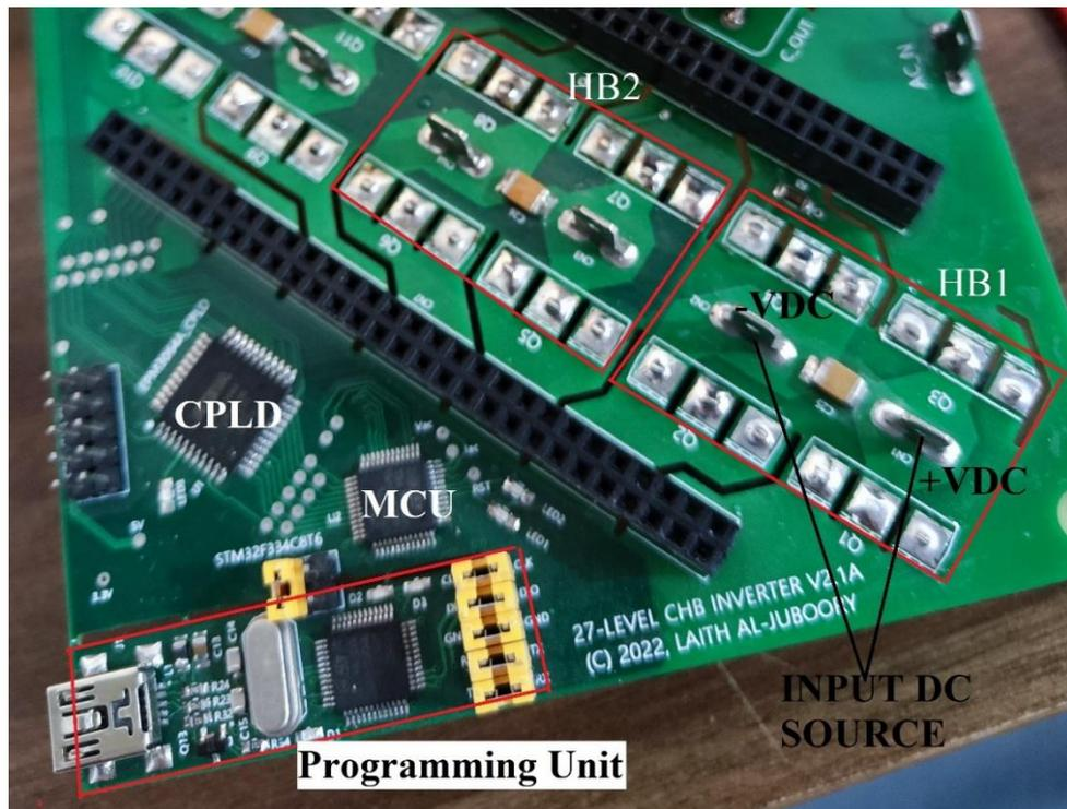
Figure 4.10 The Actual Design of the Main Board (MCU, CPLD and CHBs)
