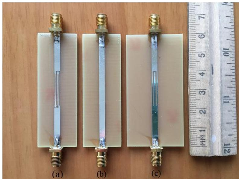
Fig. 3.45 Photographs of the fabricated prototypes; (a) the filter with the interlaced U-slots, (b) the transmission line, and (c) the filter with a single U-slot.
