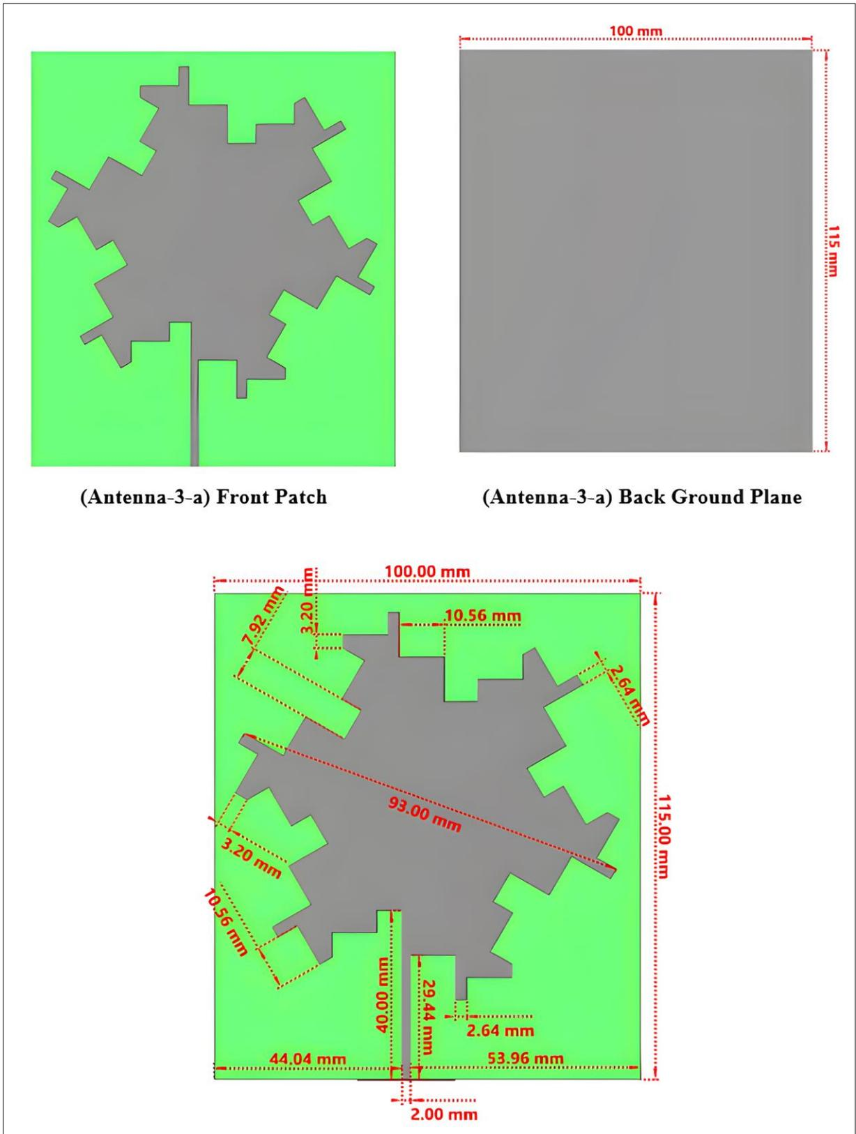
Figure 3.39 The first stage of the proposed antenna (Antenna-3-a) with dimensions.
