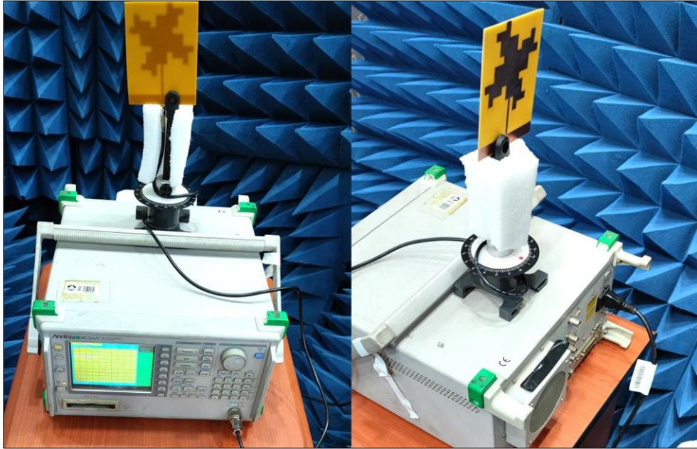
Figure 4.40 The testing environment used to measure the normalized 2D radiation pattern for the proposed (Antenna-5).
