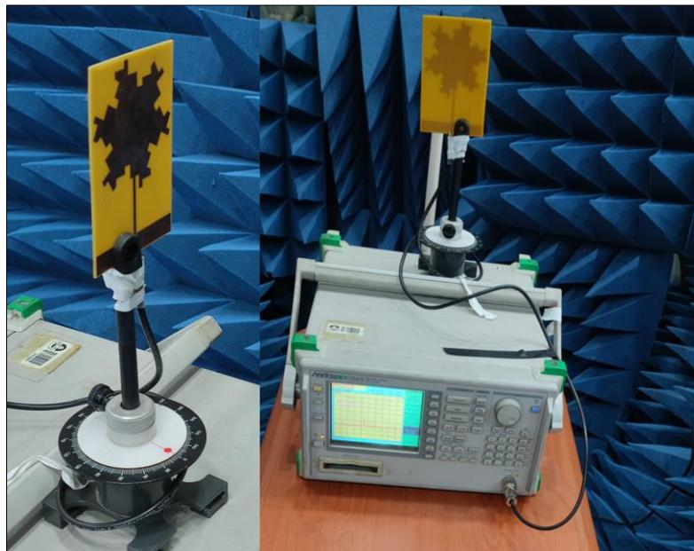
Figure 4.44 The testing environment used to measure the normalized 2D radiation pattern for the proposed (Antenna-6).
