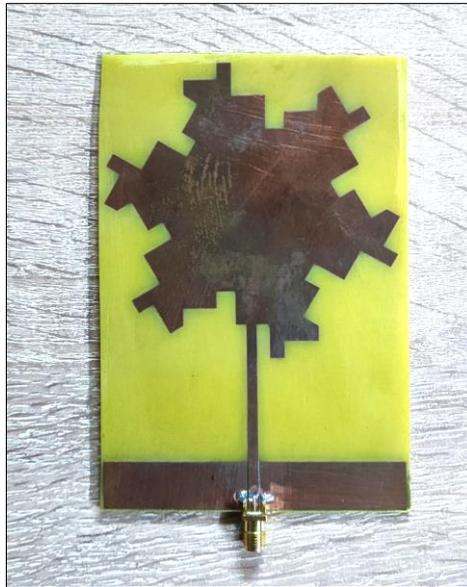
Figure 4.43 The physical structure of the proposed (Antenna-6).
