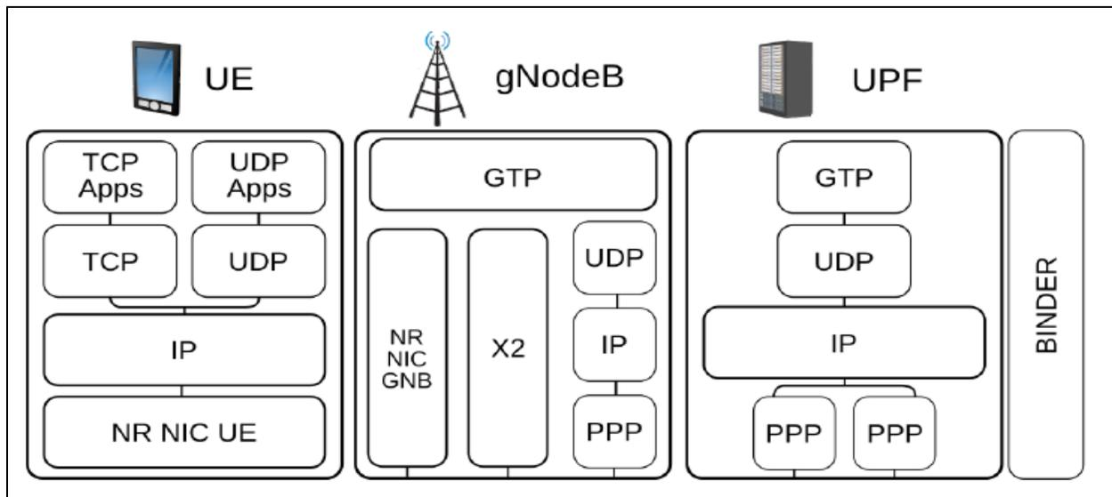
Figure.3.1: The architecture of the 5G system [61].
