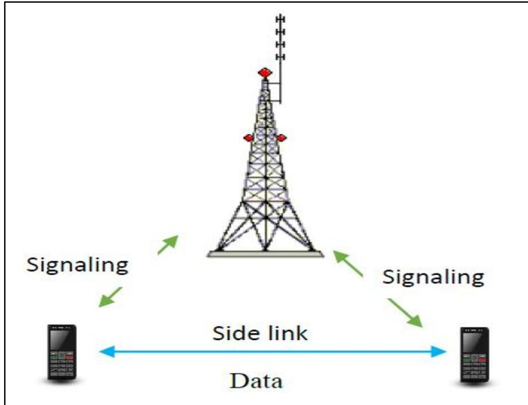
Figure.2.11: Data and control communication lines on the Side-link [50].
