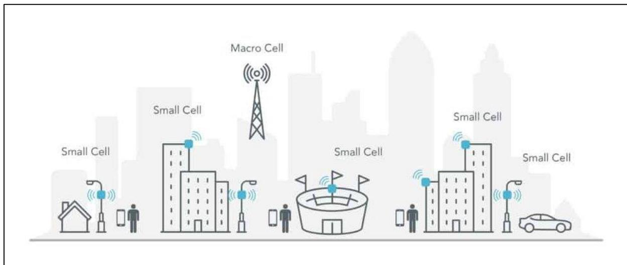
Figure.2.5: Small cell base station[36].
