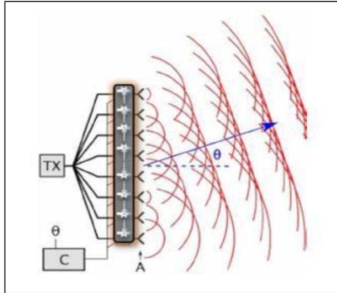
Figure.2.4: The influence of phase shift on beamforming [33].
