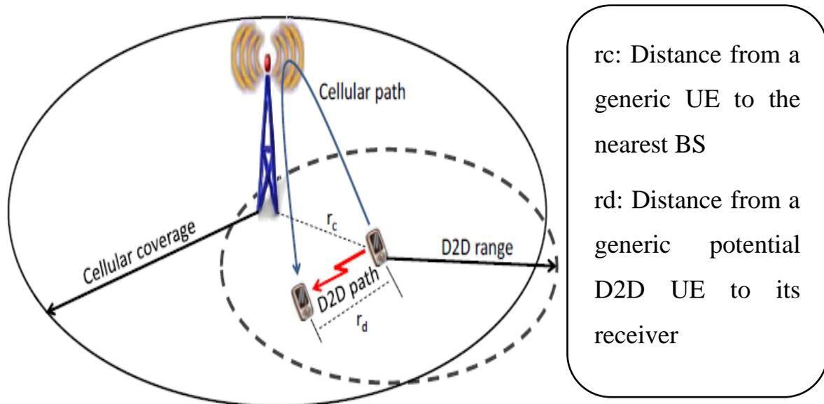
Figure.2.13: Wireless network with D2D capability [55].
