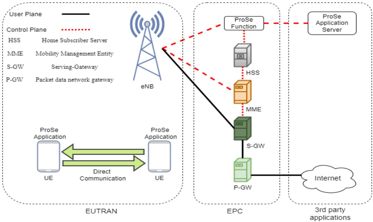
Figure.2.12: D2D communication-based architecture of 3GPP ProSe[52].
