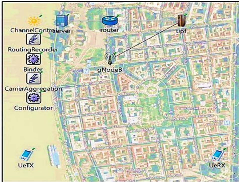
Figure.3.5: Simulation D2D communication in OMNET++ in NED file.
