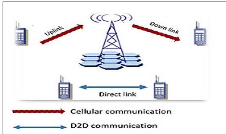
Figure.2.7: Device to Device (D2D) communication [17].
