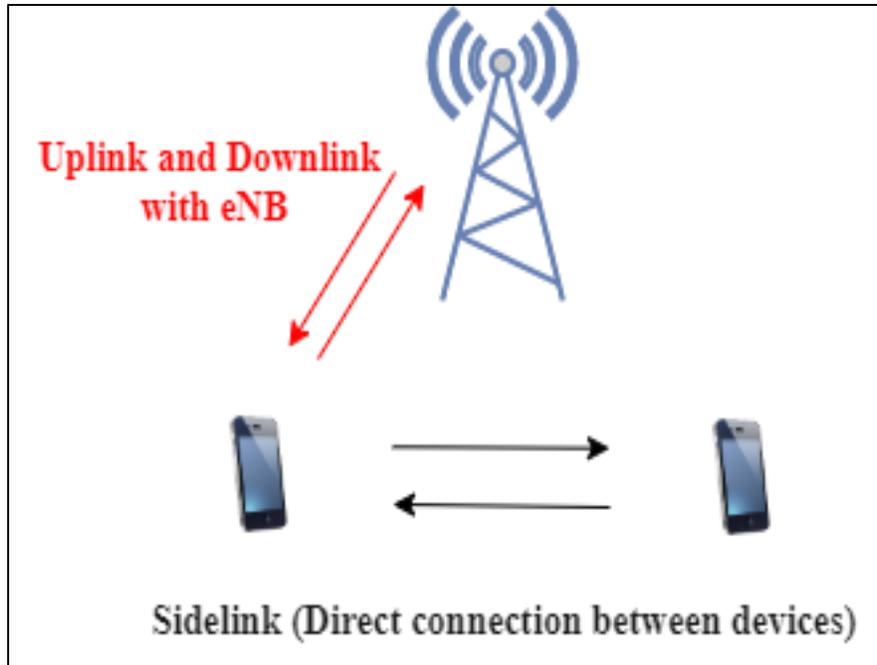
Figure.3.4: Sidelink Control and Data communication links.
