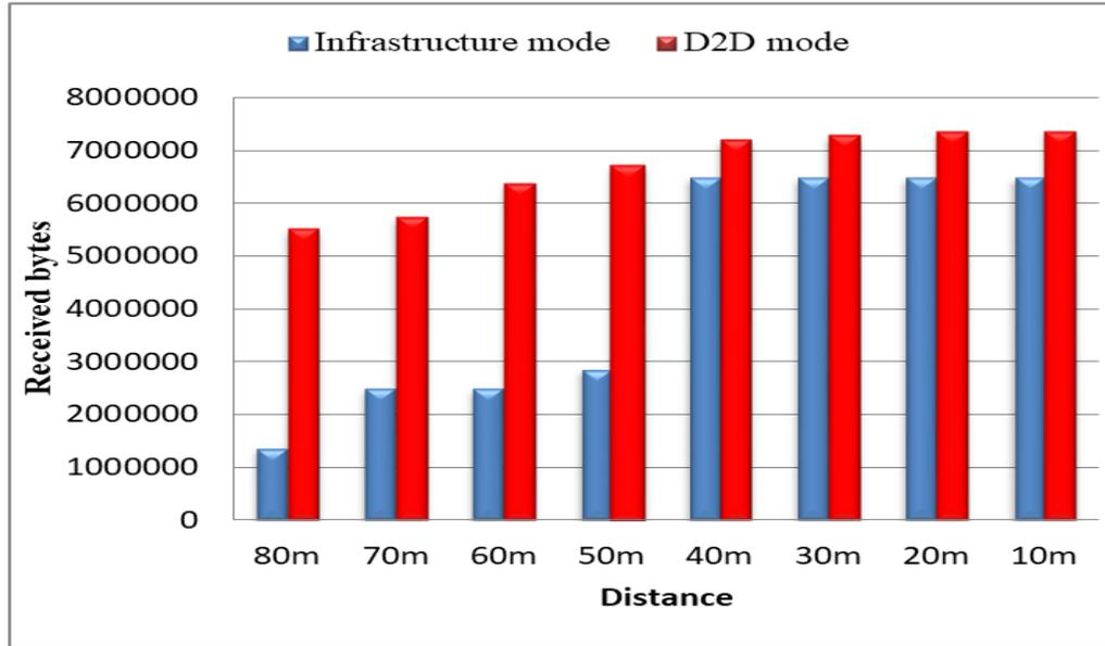
Figure.4.3: Received bytes versus distance.
