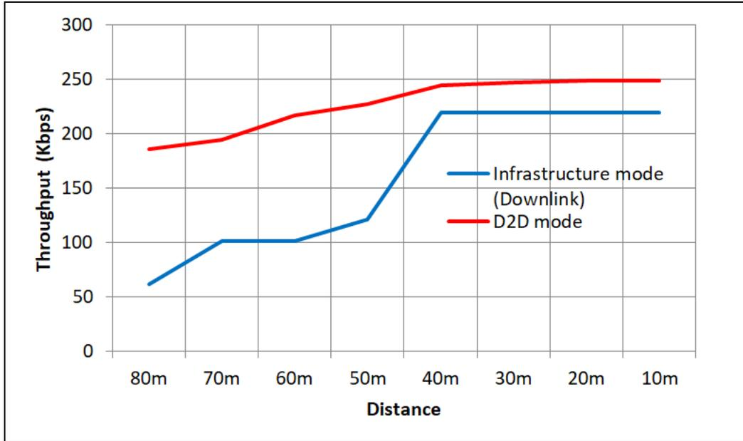
Figure.4.2: Downlink Throughput versus Distance.
