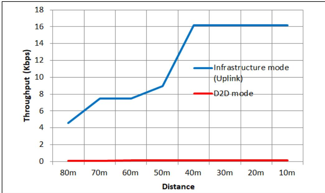
Figure.4.1: Uplink Throughput versus Distance.
