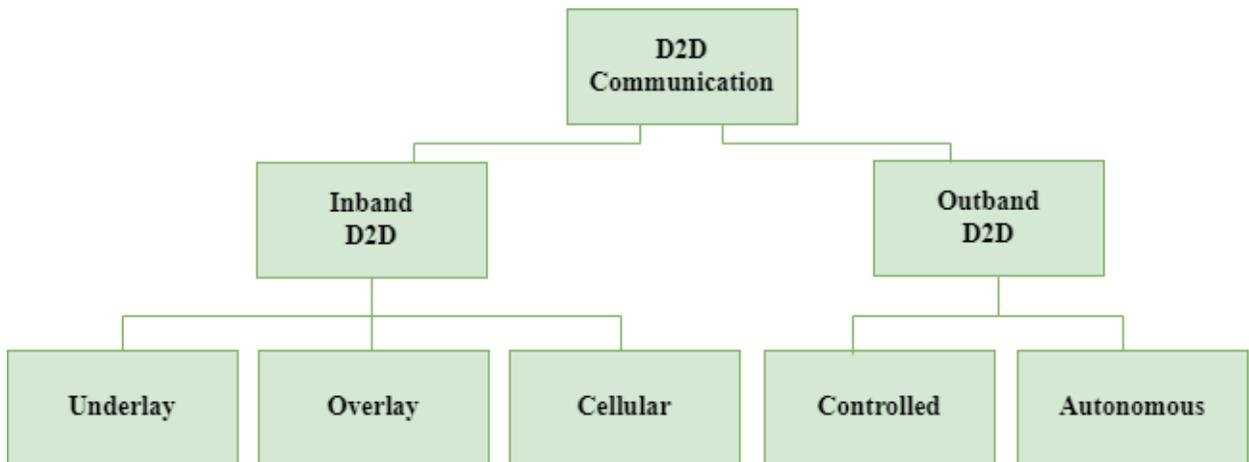
Figure.2.8: Classification of D2D communications [43].
