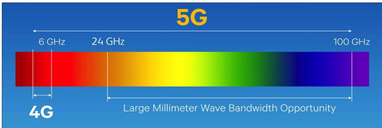
Figure.2.1: The Millimeter-wave Bandwidth [26].
