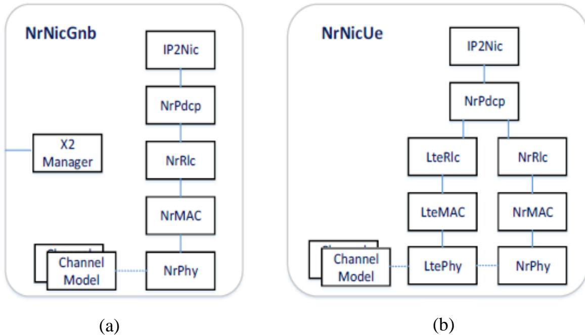
Figure.3.2: The structure of NIC modules in NR
