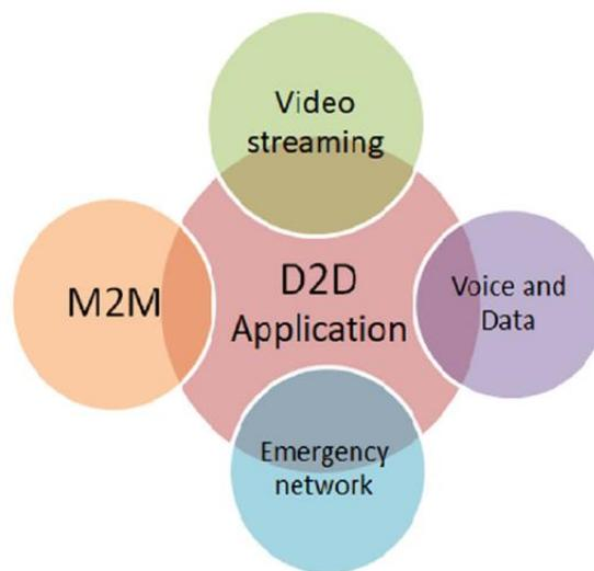
Figure.2.10: Applications of D2D communications [47].
