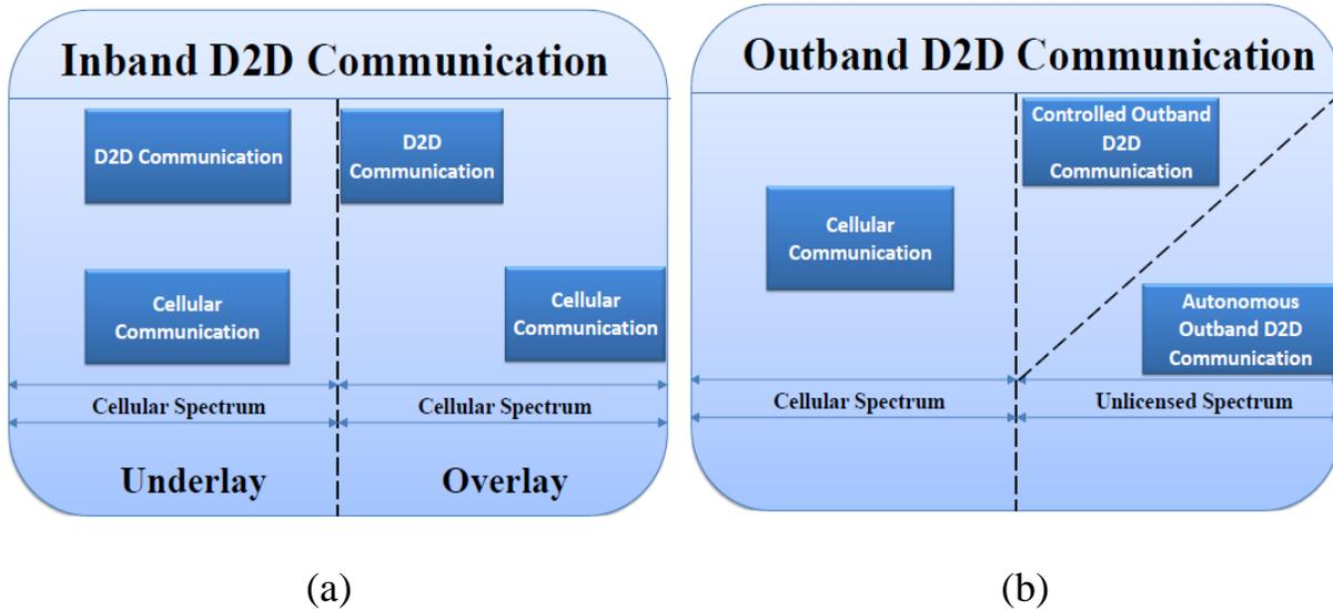
Figure.2.9: The spectrum of D2D communications in wireless networks
