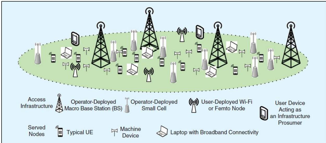
Figure.2.6: Ultra Dense Networks (UDN) in 5G wireless networks [38].
