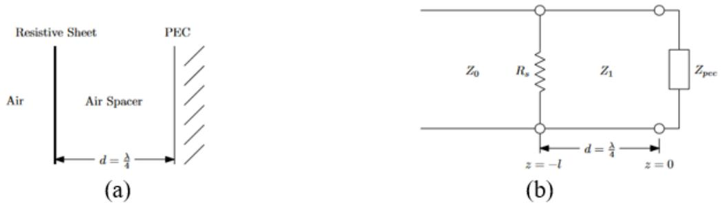
Figure 2.3 (a) Diagram of the Salisbury screen (b) transmission line equivalent circuit [35].
