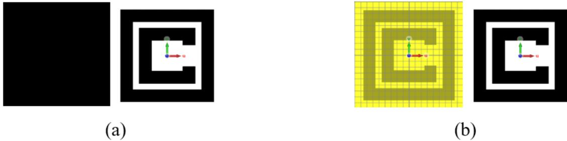
Figure 4.39 Geometry of double ring (open inner ring) unit cells (a) carbon GP, (b) copper GP.
