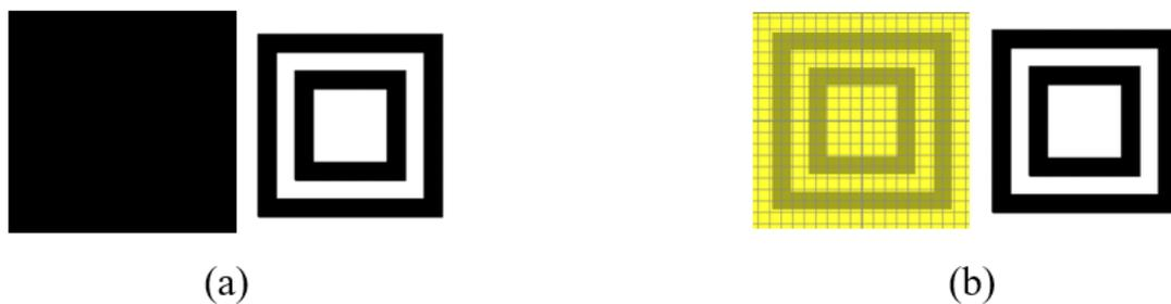
Figure 4.30 Geometry of the carbon rings unit cells (a) carbon ground plane, (b) copper ground plane.
