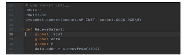
Figure 4.2 UDP Socket API piece of code
