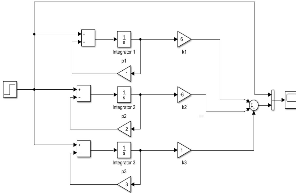
**Fig. 2 :** Simulation Diagram for the Diagonal Canonical form (DCF)
