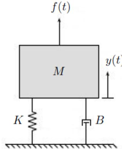
Figure 1: Simple mechanical system.
