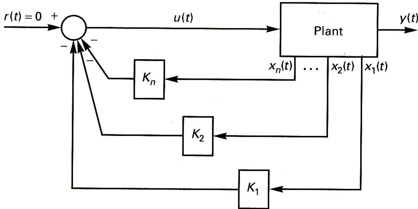
Figure 2: Pole-placement design.
