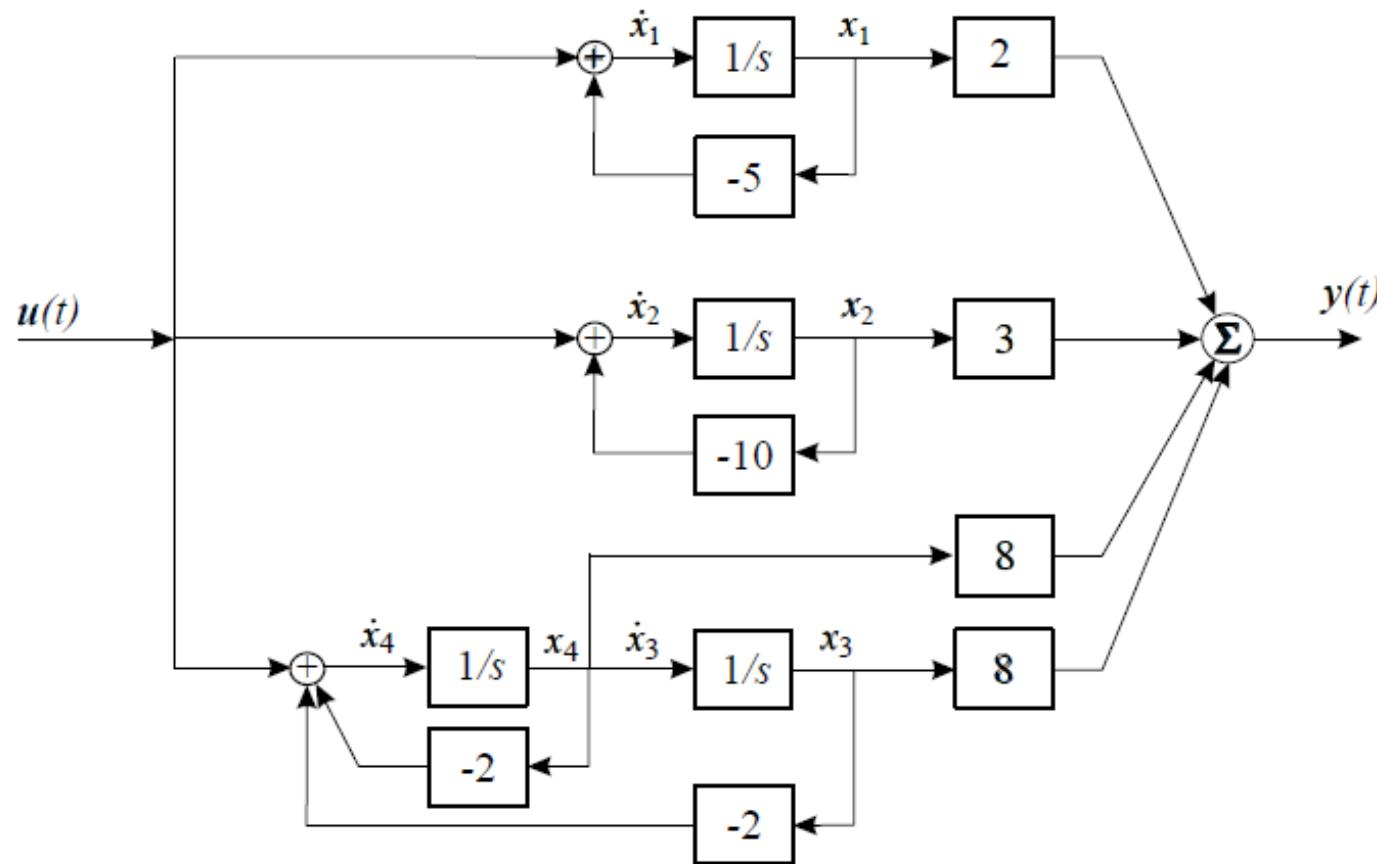
**Figure 3:** Simulation diagram for a system with complex conjugate poles
