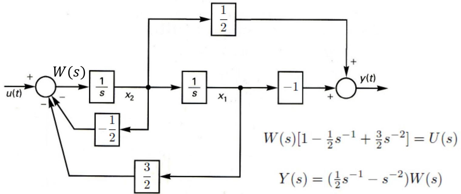
Figure 3: Simulation diagram for Example 3 in control canonical form.
