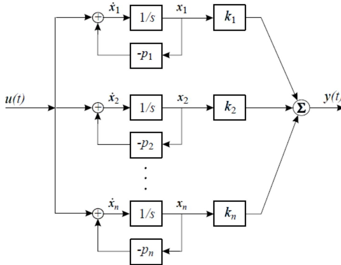
Figure 1: The simulation diagram for the Diagonal Canonical form
