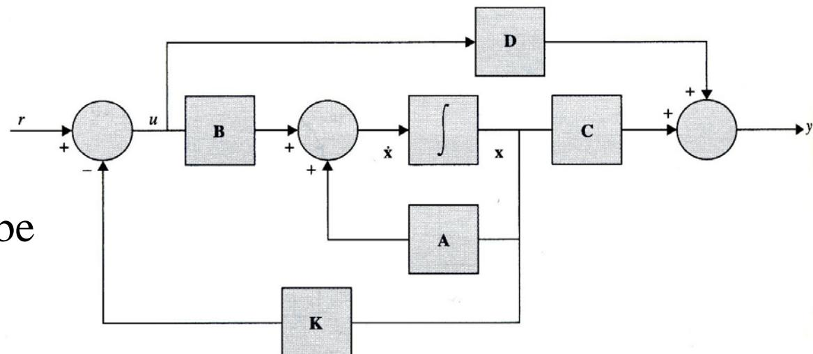
**Figure 1:** State variable feedback system.
