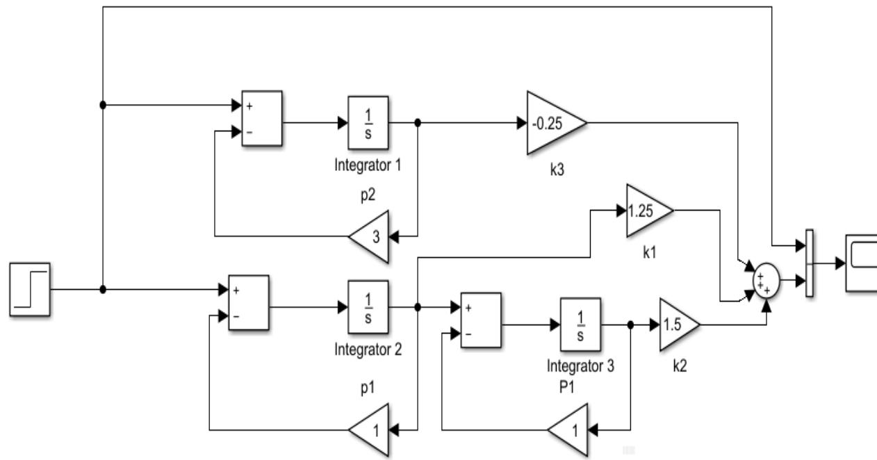
**Fig. 3 :** Simulation Diagram for the Jordan Canonical form (JCF)
