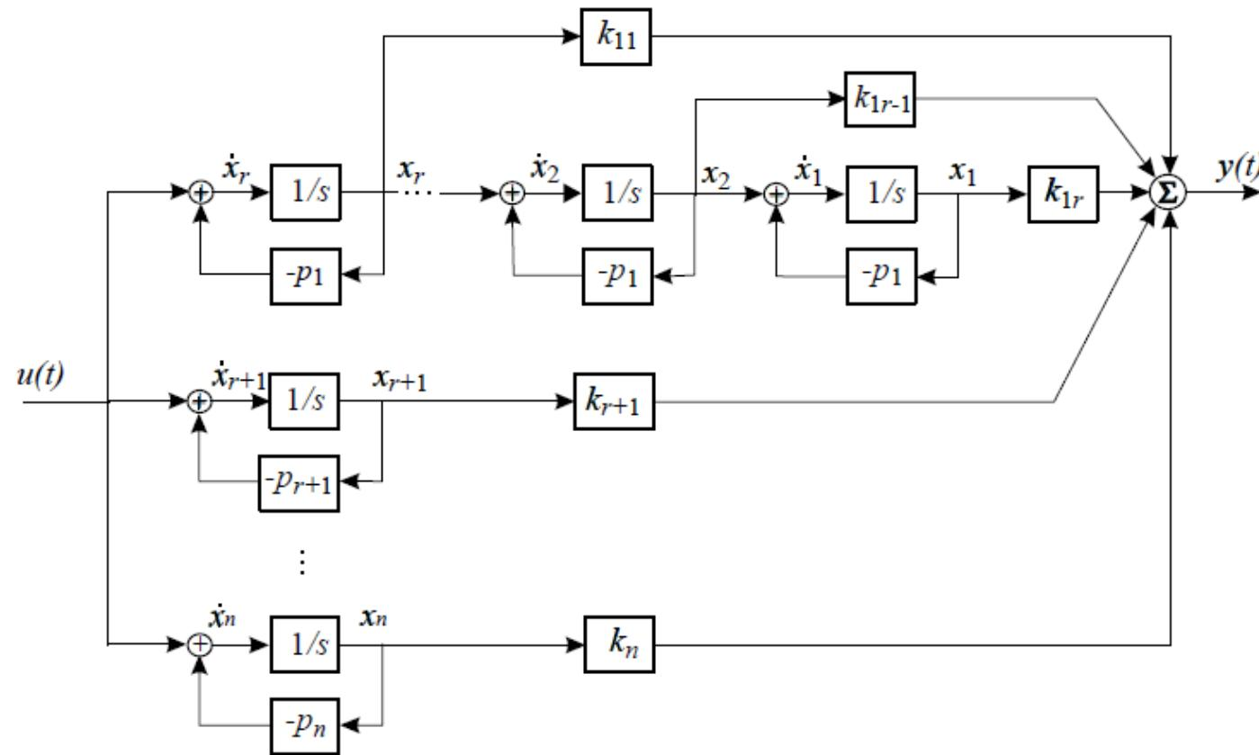
Figure 4: The simulation diagram for the Jordan canonical form
