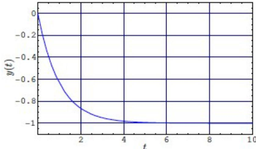
**Figure 1:** Output response of the system to a step input.
