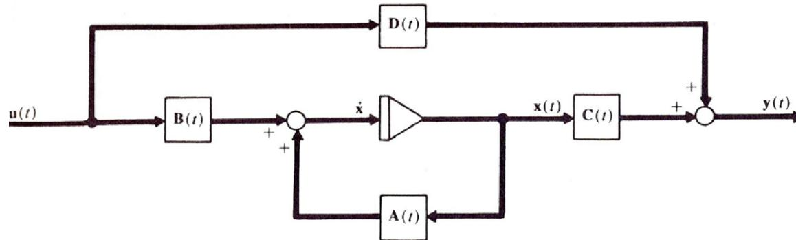
Figure 2 State space representation of CT linear system.
