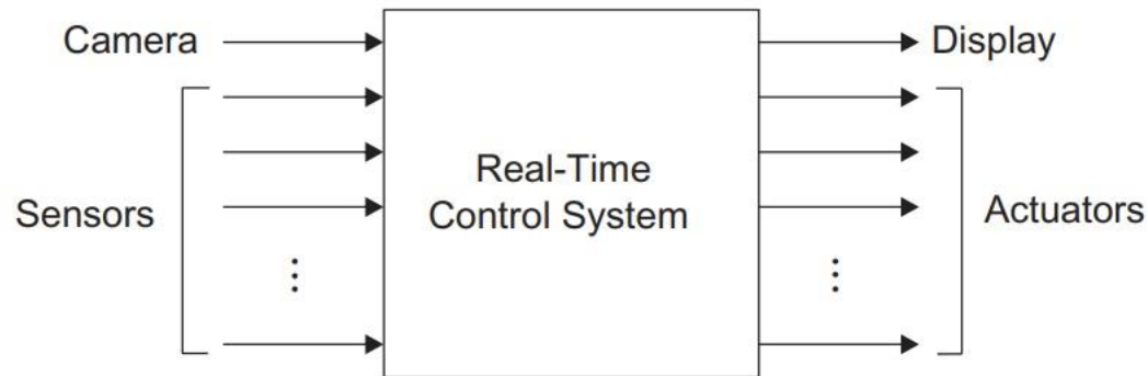
Figure 1.2. A real-time control system including inputs from a camera and multiple sensors, as well as outputs to a display and multiple actuators.
