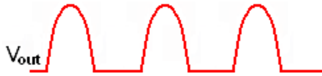
Figure 4c: 60 Hz half-wave output voltage for three input cycles
