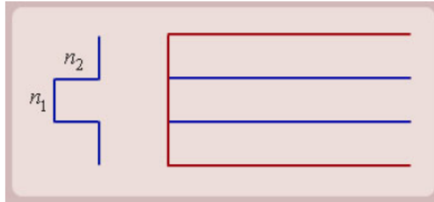
Figure (5): Step Index Fiber (Refractive index profile)
